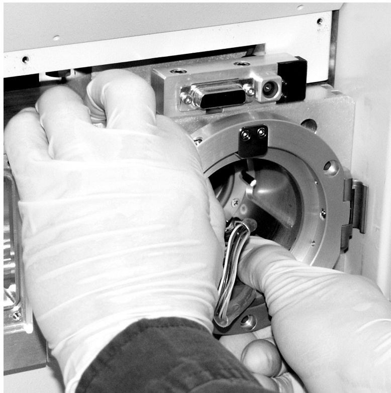
Figure 56. Removing the ion optics cage assembly
