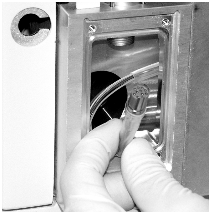
Figure 53. Unplugging the ion source cable harness connector
