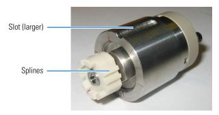
8. Also verify that the two splines on the pod align with the matching splines inside the valve holder (see Figure 27). If necessary, twist the end of the pod to adjust the position of the splines.
