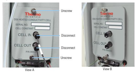
4. Grip the two loosened screws and pull the cell cover toward you to remove it from the component panel. Do not pull from the CELL IN and CELL OUT fittings.
