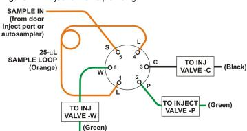
Figure 14. Injection valve plumbing
