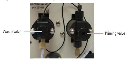
4. If the O-ring is removed with the valve knob in Step 3, pull the O-ring off the end of the knob (see Figure 36). If the O-ring is not removed with the valve knob, insert a thin object (for example, the bent end of a paper clip) into the cavity in the pump head and carefully pull out the O-ring.
