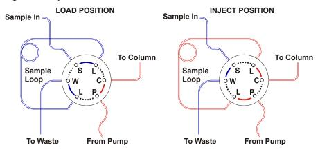
Eluent flows through the Load or Inject path, depending on the valve position.
