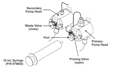
3. Open the priming valve by turning it one-quarter to one-half turn counterclockwise.
