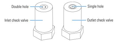
**Note** The pump will not operate properly unless the cartridge is installed in the housing in the correct orientation. Liquid flows through the check valve in the large single hole and out the small double holes.
