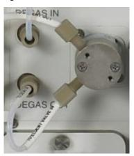
The eluent valve controls the flow from the eluent reservoir. The valve opens automatically when the pump is started and closes when the pump is turned off. The valve can also be opened and closed manually from the Chromeleon ePanel (see "Chromeleon 7 Chromatography Data System" on page 14). This lets you perform service procedures on pump components without eluent leaks occurring.
