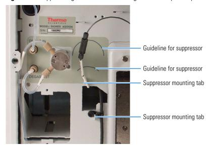
12. Press the suppressor onto the tabs and then slide it down until it locks into place. Pull slightly on the center of the suppressor to verify that it is securely fastened.
