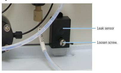
4. Remove the leak sensor from the component panel and begin pulling the cable out of the opening in the panel. The cable attached to the leak sensor is connected to a matching cable inside the Dionex Aquion. Continue pulling the cable until the connectors for the two cables are outside the panel (see Figure 47).
