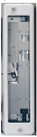
The column heater provides temperature control for the separator and guard columns.
