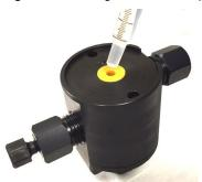
4. Reinsert the piston into the seal, and then push the piston into the head (see Figure 34). The seal should hydraulically pop out from the head.
