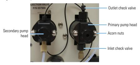
**Note** The *inlet* check valve assembly housing has a 1/4-28 port. The *outlet* check valve assembly housing has a 10-32 port.
