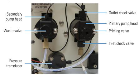
The secondary pump head delivers eluent to the remainder of the chromatography system (the injection valve, column, and detector). The waste valve is on the front of the secondary pump head (see Figure 12).
