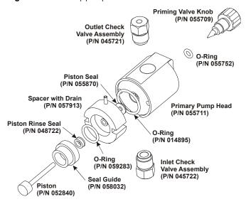
Figure 31. Secondary pump head
