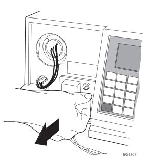
Figure 4-3 Removing the Flow Cell Assembly
