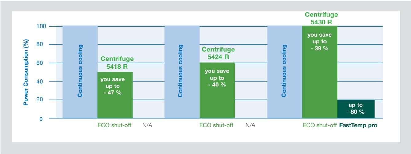
Comparing continuous cooling, ECO shut-off, and FastTemp pro. (N/A: not applicable)
