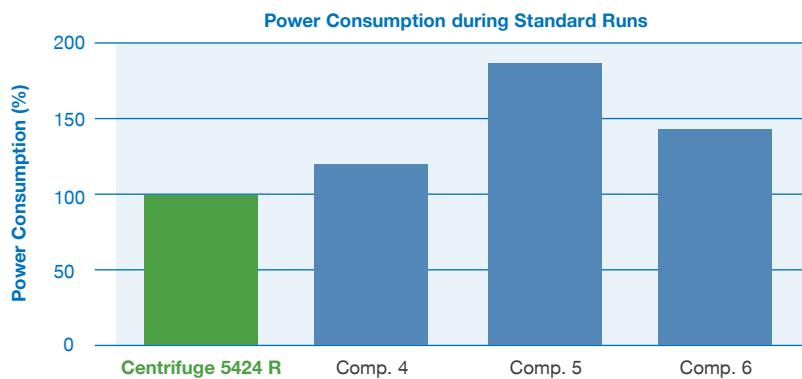
20,000 x g; 60 min; 4 °C; 10x 1.5 mL microtubes with 1,000 µL water each; FastTemp run before
