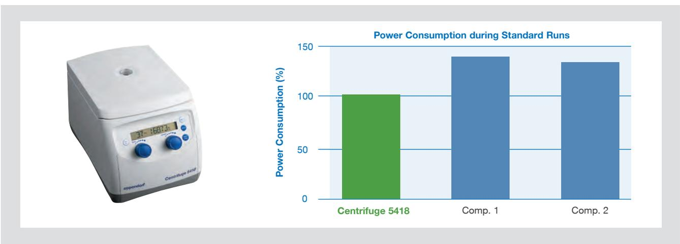
16,000 x g, 60 min, room temperature, 10x 1.5 mL microtubes with 1,000 µL water each
