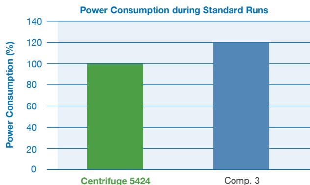
20,000 x g, 60 min, room temperature, 10x 1.5 mL microtubes with 1,000 µL water each
