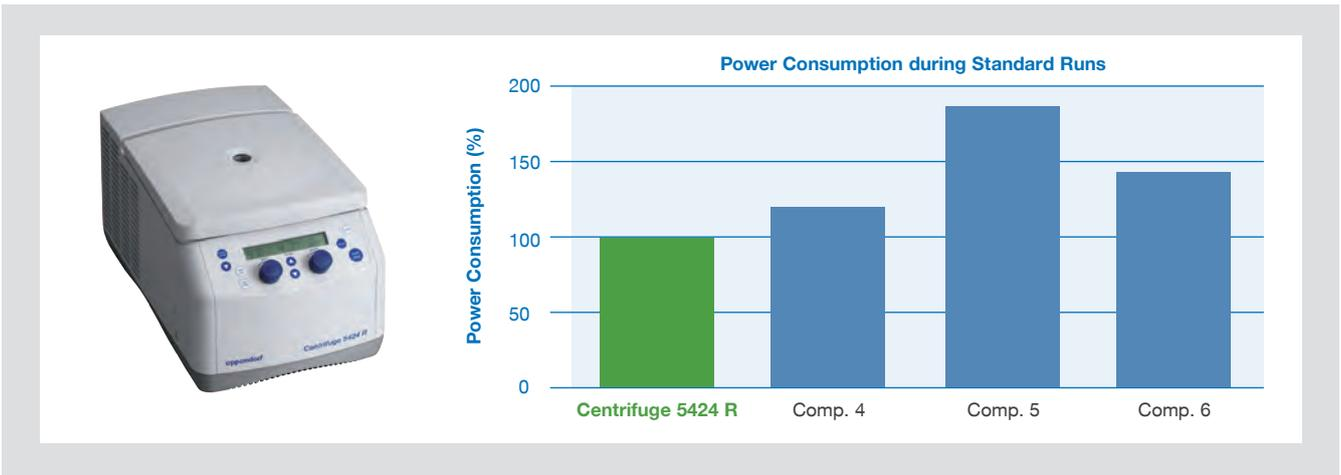
20,000 x g; 60 min; 4 °C; 10x 1.5 mL microtubes with 1,000 µL water each; FastTemp run before
