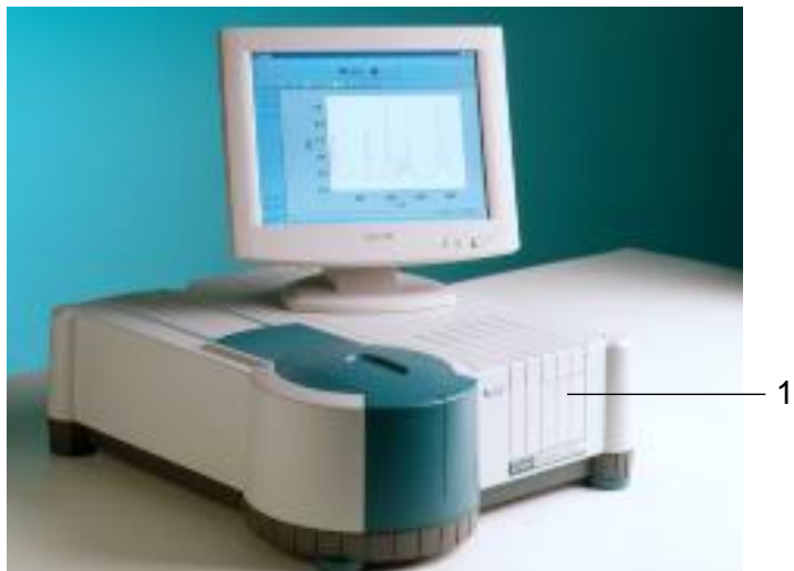
Figure 5. The snap-out panel (1) on the front of the Cary 50
