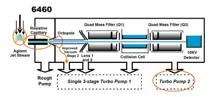
Figure 1 Innovative Enhancements (circled) in the K6460<sup>\*</sup>
