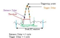
Figure 5 Example of Trigger Window
