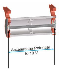
Figure 14 Collision cell design
