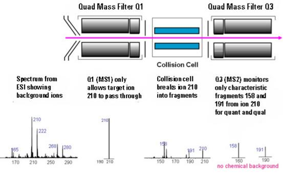
Figure 8 Multiple reaction monitoring (MRM)
