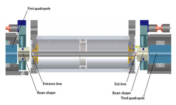
Figure 12 Collision cell technology for the K6460 produces higher sensitivity and faster responses without memory or cross-talk effects
