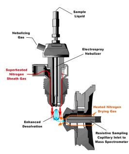
Figure 9 Electrospray Ion Source with Agilent Jet Stream Technology
