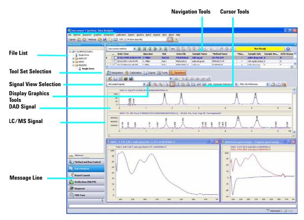
The various tool sets available in Data Analysis View are shown on the following pages. You can view a description of a button by moving the cursor over it.
