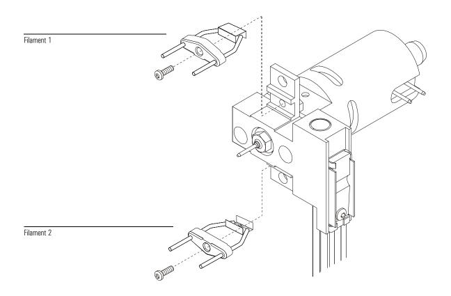
6 Maintaining the MSD To reinstall a filament
