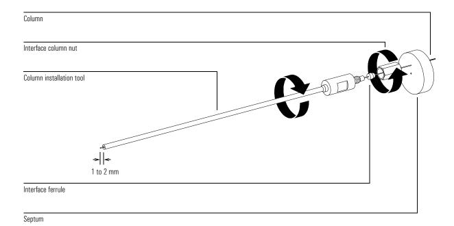
8 Remove the column and nut from the installation tool.
