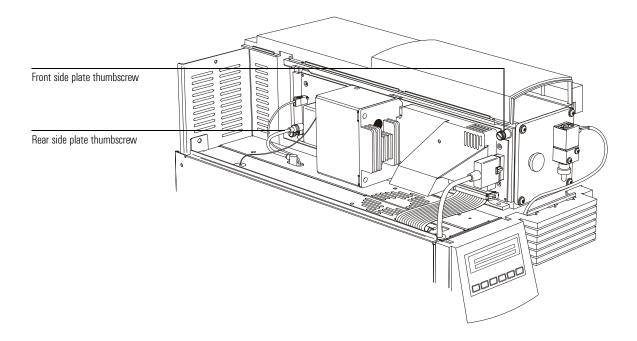
The MSD can now be stored or moved. The foreline pump cannot be disconnected. It must be moved with the MSD. Make sure the MSD remains upright and is never tipped on its side or inverted.
