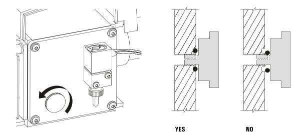
8 Turn the vent valve knob counterclockwise *only* 3/4 turns or until you hear the hissing sound of air flowing into the analyzer chamber.
