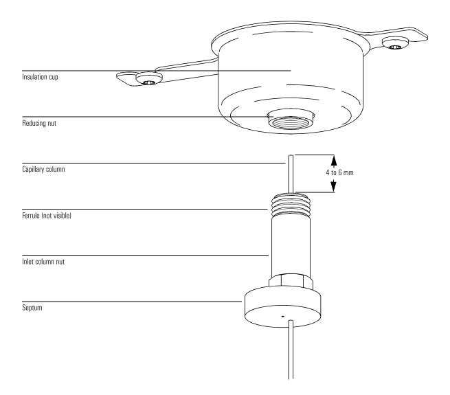
1 Installing GC Columns To condition a capillary column
