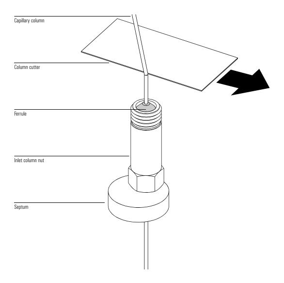
1 Installing GC Columns To install a capillary column in a split/splitless inlet
