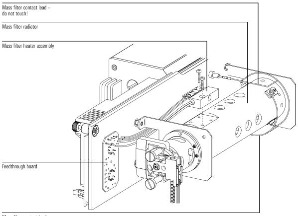
Mass filter contact lead do not touch! 6 Maintaining the MSD
