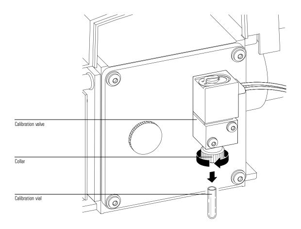
6 Maintaining the MSD To refill and reinstall the El calibration vial
