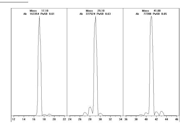
Methane pre-tune after more than a day of baking out. Note the low abundance of m/z 19 and absence of any visible peak at m/z 32. Your MSD will probably show more water at first, but the abundance of m/z 19 should still be less than 50% of m/z 17.
