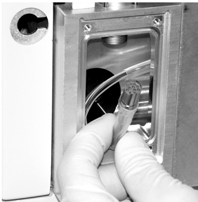
Figure 52. Unplugging the ion source cable harness connector
