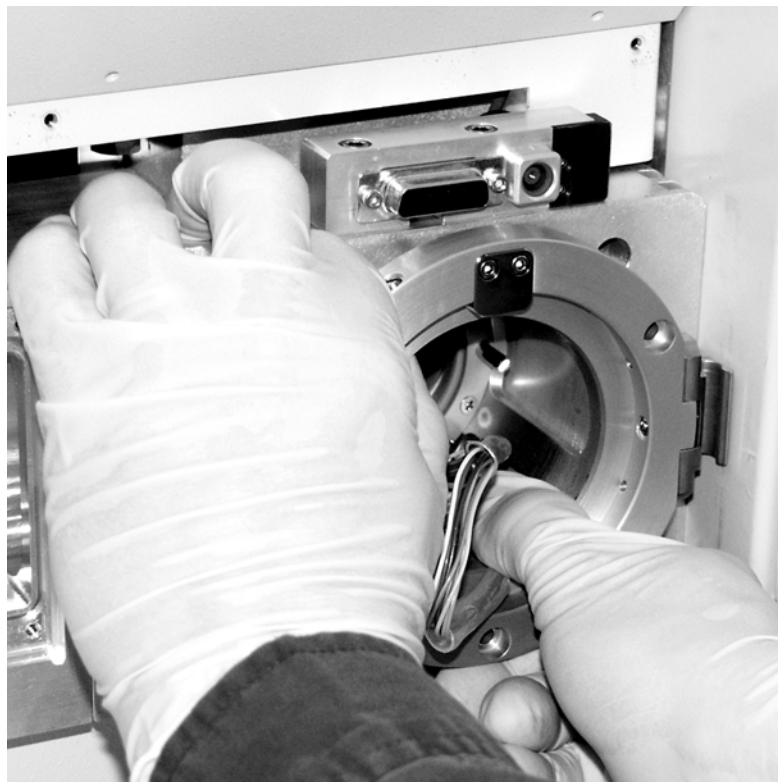
Figure 55. Removing the ion optics cage assembly
