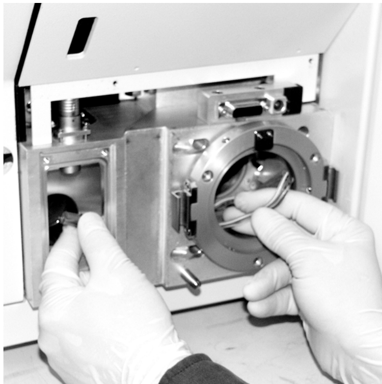
Figure 54. Pulling the ion source cable harness out of the ion optics cage assembly
