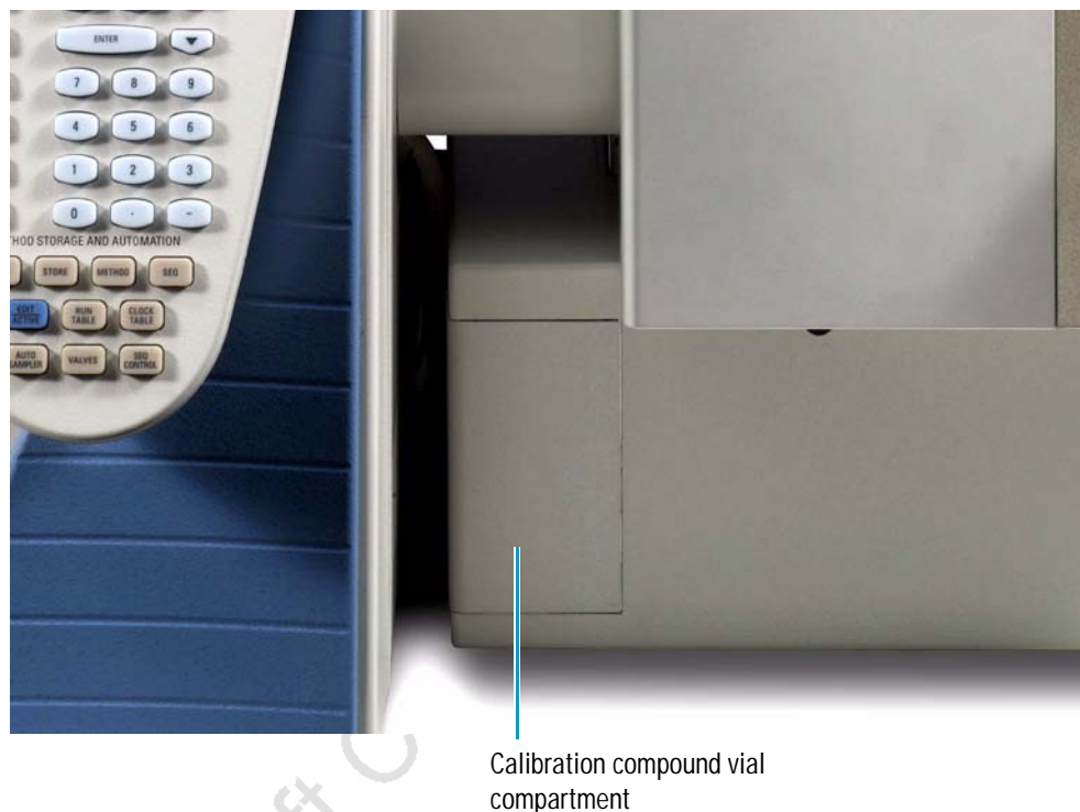
Figure 60. Location of the calibration compound vial compartment
