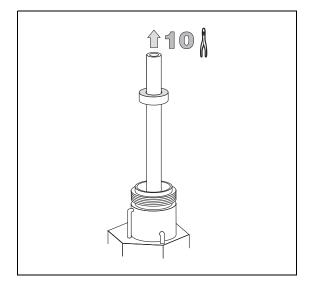
11. If you are going to use a new liner, go to step 14. If you are going to clean the liner, put the dirty liner into an ultrasonic bath filled with a methanol/acetone mixture (1:1) and sonicate it for about half an hour. 12. Using tweezers, remove the liner from the bath and dry it with compressed clean air.
