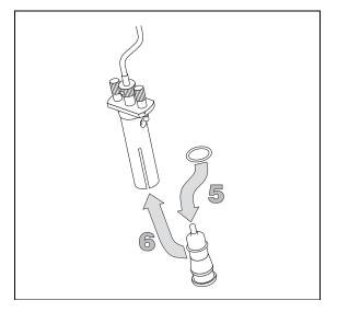
7. Insert the lamp holder into the lamp housing
