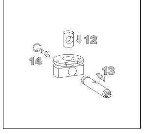
15. Reassemble the two parts of the injector body.
