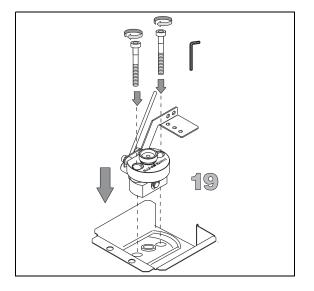
21. .Reinstall the automatic actuator on the OC housing paying attention to insert the valve lever through the slot provided on the automatic actuator shaft.
