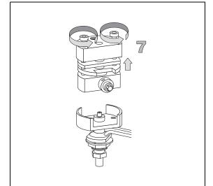
8. Disassemble the injector body, separating the head from the lower part.
