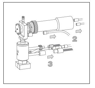
4. Loosen the nut that fixes the ECD detector to its base body with the proper tool contained in the standard outfit and remove the detectors from the ECD base body.
