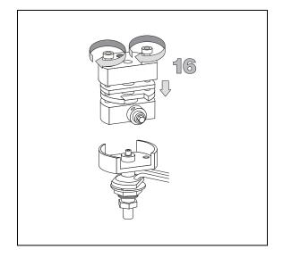
17. Insert the valve lever into its housing, tightening the retaining screw.
