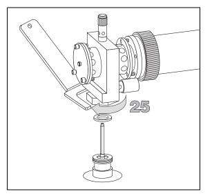
25. Place the detector on its base body, paying attention that the aluminium ring has been inserted in the correct position, then tighten the fixing nut.
