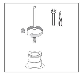
9. Place the detector on its base body, paying attention that the aluminium ring has been inserted in the correct position, then tighten the fixing nut.
