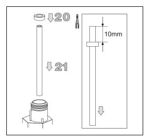
22. Tighten the liner cap using the liner cap wrench provided with the GC.
