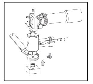
5. Using tweezers, remove the worn silver seal from its housing in the base body.
