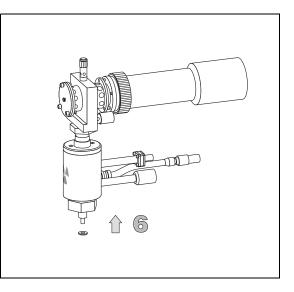
7. Remount the detectors on the ECD base body, tightening the fixing nut with the proper tool.
