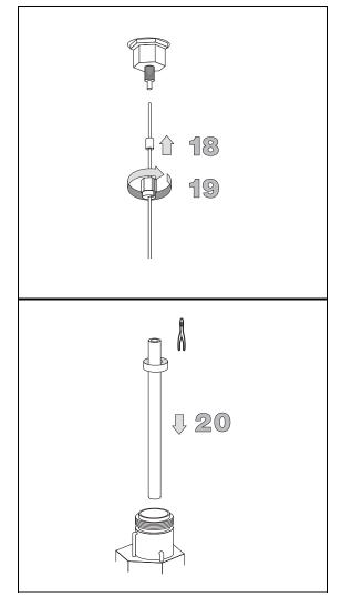
20. Using tweezers, insert the liner into the injector and push it gently towards the bottom fitting. Make sure you insert the bevelled end of the liner towards the bottom of the injector.
