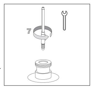
11. When the jet is dry, insert the jet into the detector base body and tighten it.
