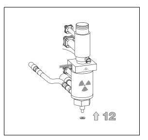
13. Remount the detector on its base body, tightening the fixing nut with the proper tool.
