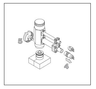
6. Unscrew the two fixing screws and remove the lower connector holder assembly from the detector cell.
