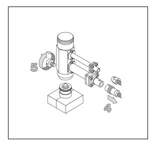
6. Using the tool provided with the GC, unscrew the worn jet from the detector base body.
