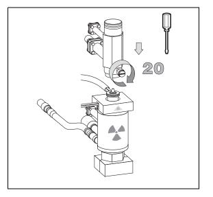
21. Reconnect the signal and ignition cables to the FID and the signal, excitation and heater cables to the ECD detector.
