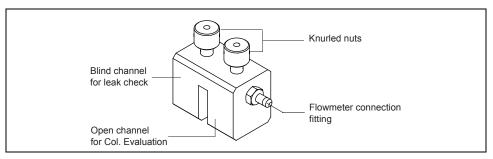
Figure 10-1. Column-flow Meter Connector
