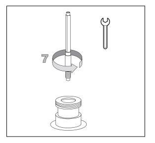
8. Place a new jet into the housing and tighten it.
