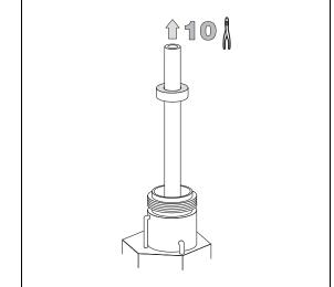
11. If you are going to use a new liner, go to step 14. If you are going to clean the liner, put the dirty liner into an ultrasonic bath filled with a methanol/acetone mixture (1:1) and sonicate it for about half an hour. 12. Using tweezers, remove the liner from the bath and dry it with compressed clean air.
