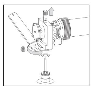
Using the 5 mm wrench provided with the GC, loosen the worn jet and remove it from the detector base body.
