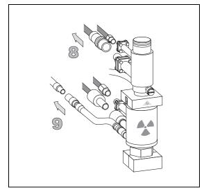
10. Loosen the nut that fixes the ECD detector to its base body with the proper tool contained in the standard outfit and remove the detectors from the ECD base body.
