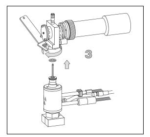
4. Disconnect the signal, excitation and heater cables from the ECD detector.
