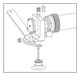
7. Loosen the knurled nut that fixes the photomultiplier tube and remove it from the detector body.
