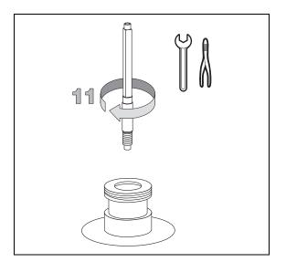
12. Place the detector on its base body, paying attention that the aluminium ring has been inserted in the correct position, then tighten the fixing nut.
