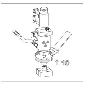
11. Using tweezers, remove the worn silver seal from its housing in the base body.
