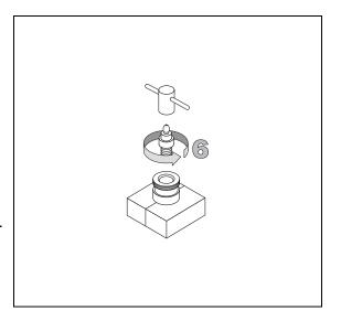
When the jet is dry, place the jet into the housing and tighten it with the proper tool. Ensure the jet is perfectly vertically aligned to avoid damaging its ceramic part.
