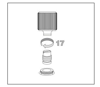
Insert the analytical column with its ferrule into the bottom of the injector in its previous position. Refer to the TRACE<sup>™</sup>GC Operating Manual for instructions.
