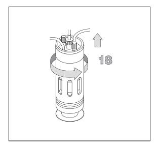
19. Tighten the detector cell using the fixing tool provided.
