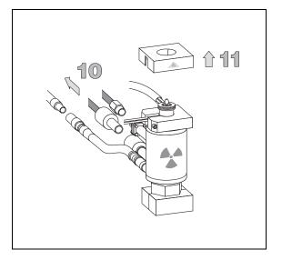
12. Remove the heater from the top of the ECD detector unscrewing and removing the 4 mm Allen fixing screw. Use a 3 mm Allen wrench.
