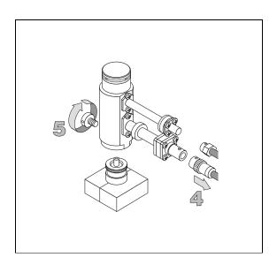
6. Using the tool provided with the GC, unscrew the metal jet.
