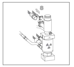
9. Loosen the fixing screw on the front of the NPD cell and remove it.
