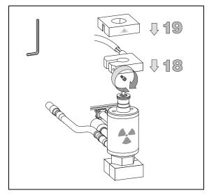
20. Remount the NPD detector on the top of the ECD and tighten the fixing screw.
