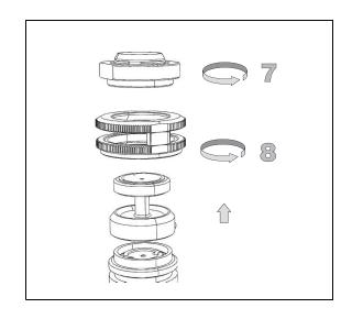
9. Use the liner cap wrench provided with the GC to remove the injector liner cap.
