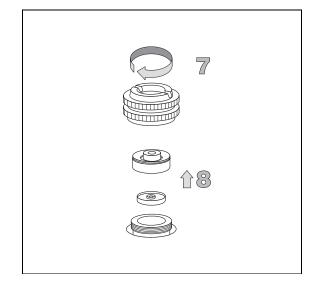
9. Use the screwdriver provided with the GC to remove the injector liner cap.
