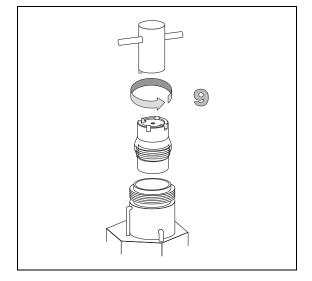
10. Use tweezers to remove the liner with the graphite seal.
