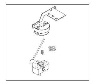
19. Remount the injector body on its base, tightening the two Allen screws.
