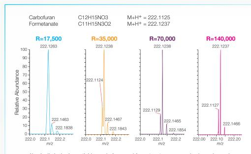
Nominally isobaric pesticides carbofuran and formetanate are unresolved or only poorly resolved at the highest resolutions available in Q-TOF instruments. The higher resolutions easily achieved by the Q Exactive instrument clearly resolve analytes from complex matrix interferences without sacrificing sensitivity.
