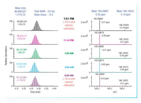
A 12-hour continuous UHPLC-MS analysis of d5 hippuric acid (*m/z* 185.0969) from rat plasma demonstrates the Q Exactive mass spectrometer's robust ion statistics and highly stable mass accuracy.
