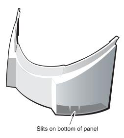
Position the in and out tubes either so that they will both pass through one port, or so that they pass on either side. Replace the sample compartment front panel, ensuring that the tubes are correctly located in the slit(s) and are not being pinched between the front panel and the body of the instrument. Ensure that the tubes do not obstruct the light beam. If necessary, secure the tubes using the self-adhesive tubing clips supplied.
