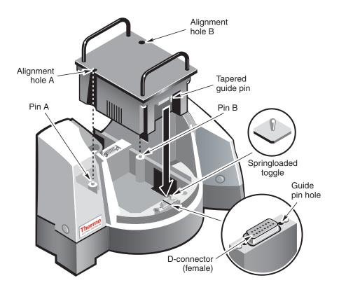
Note On the Smart Peltier Thermostatted Single Cell Holder, the alignment holes and pins are not visible due to the plastic cover over the unit. ▲
