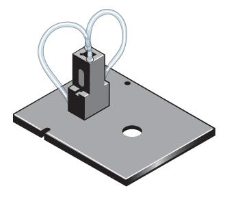
The sample compartment front panel has two slits through which the tubing can be routed. The slits are located to the left and right of the center, and open downwards. Foam baffles fit around the tubing to exclude light from the sample compartment.
