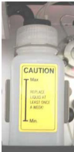
Figure 5: Rear seal wash solution bottle. Wash solution needs to be changed on a weekly basis and consists of 20% methanol or ethanol. The bottle is fitted in a metal holder and the entire holder is lifted off.
