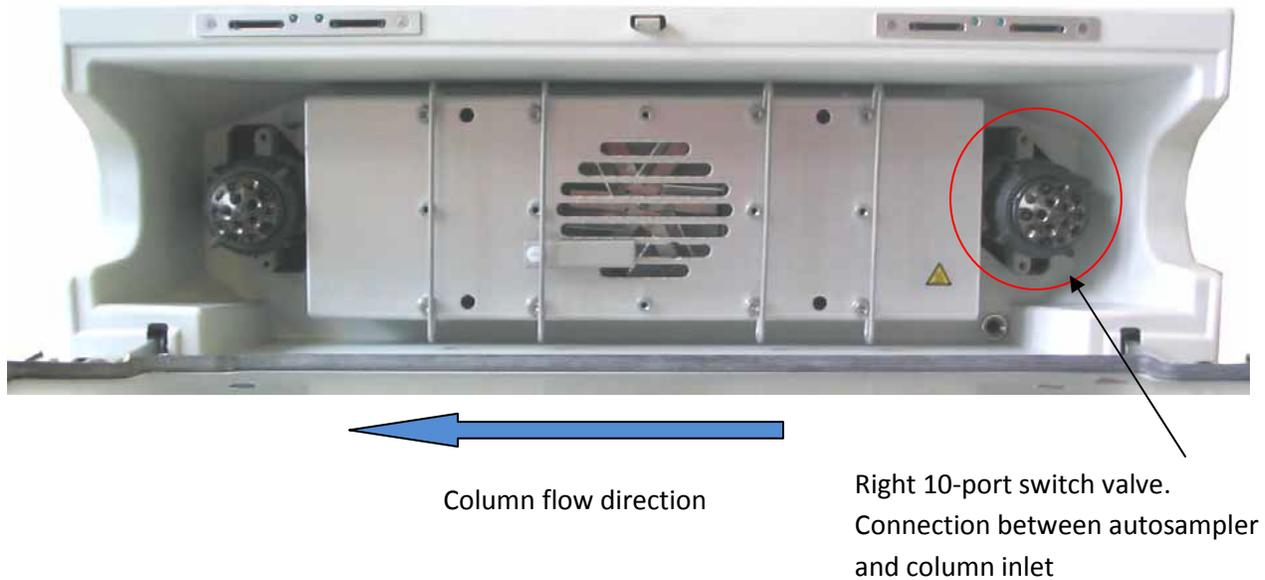
Figure 10: Internals of column compartment with two 10-port switch valves. Blue arrow indicates flow direction, which should fit with column flow directions.
