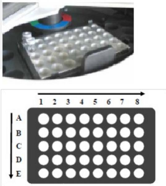
Figure 8: Upper: Autosampler - view from lid opening. Lower: Vial rack layout.
