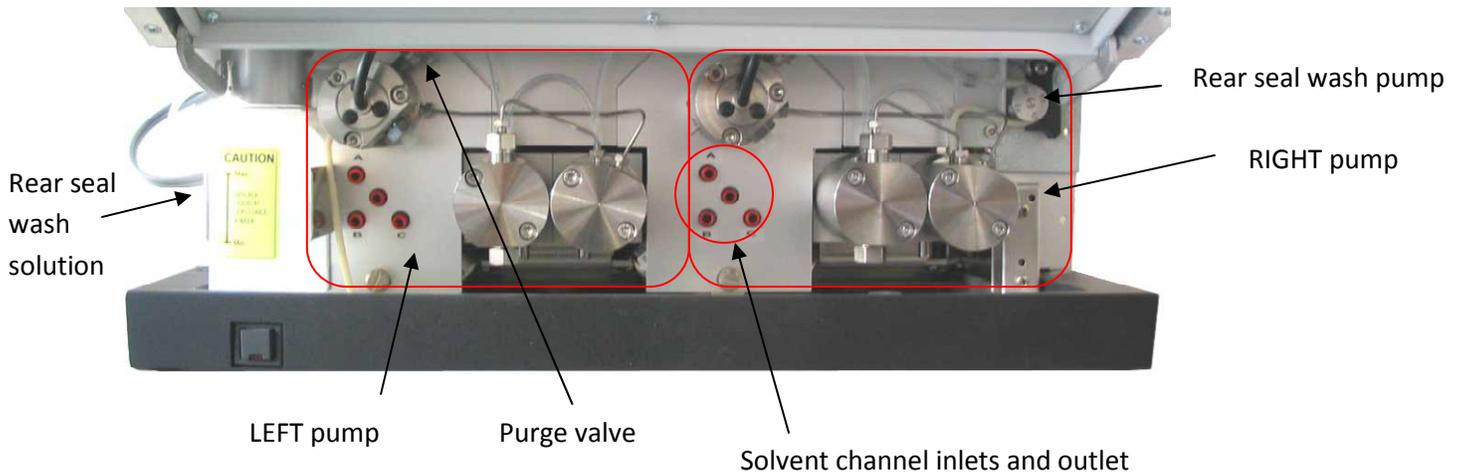
Figure 4: Internals of Dual Pump
