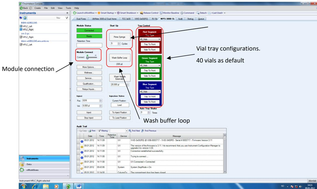
Figure 9: Autosampler tab.
