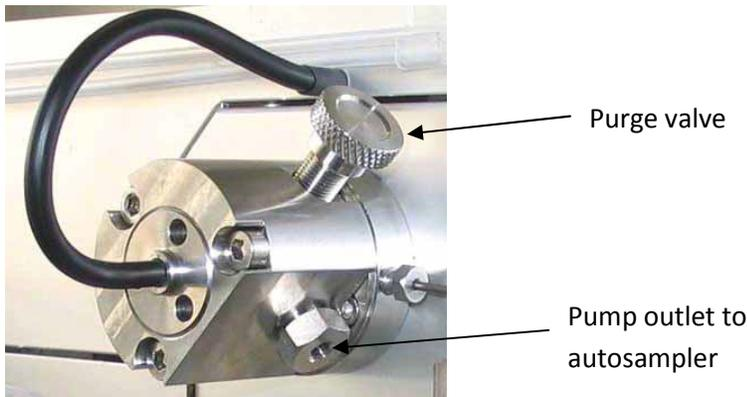
Figure 6: Pump head with purge valve and outlet to autosampler. Changing from one operating pump head to the other you simply move the yellow connection tube to the other pump head outlet.
