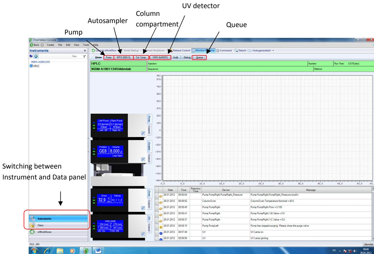
Figure 3: Module and system overview from controlling software Chromeleon™ 7. Unmarked tabs: “Home”; System overview tab. “Audit”; Audit trail logging every event in the system. “Startup”; Programmed system startup (not recommended to use).
