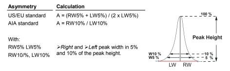
For ideal peaks, Asymmetry is A = 1. For realistic, tailing peaks, however, A is between 1.2 and 5. Values higher than 5 often produce imprecise quantitative results.
