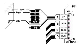
Now, start the **Server Configuration** to install/configure the **Sharable Device Dionex AD Converter**. The channels of the A/D converter are then available for installing instruments with analog signal output.
