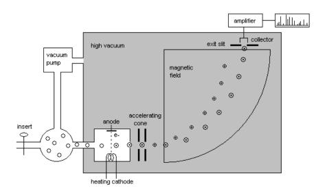
The ions that are created via the electron impact are first accelerated by means of the cones and then separated according to their mass in the magnetic field. Due to the varying intensity of the magnetic field (or the accelerating voltage), ions of different masses are directed through the exit slit into the collector and registered. In this way, mass spectrometers perform a mass scan similar to the wavelength scanning of many photodiode array detectors.
