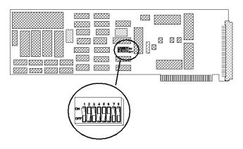
Position the board as indicated in the figure, using the block with the eight switches for setting the I/O-address as a guideline. Proper installation is in three steps:
