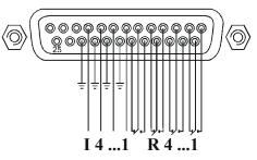
The maximum switching potential of the relays is 100 V with a contact rating of 10 W. Ensure not to exceed a max. current of 0.5 A. To enable a reaction to external events (e.g. inject signal), the relay board offers four remote inputs, which are released when a relay closing contact (e.g. of the autosampler) grounds the corresponding input signal.
