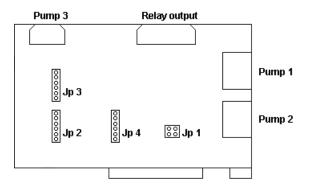
The figure illustrates the elements of the pump control board that are relevant for installation. Installation requires the following steps:
