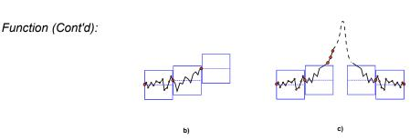
If three successive data points are located above or below the rectangle (simplified!), the peak recognition algorithm will recognize a peak. When the signal difference of one data point to the next one becomes so small that they are within the bandwidth again, the peak end is indicated (c).
