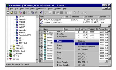
If four different channels of a sample are recorded with a diode array detector during sample processing, as is in this example, a separate chromatogram will be available for each channel (here: **3DFIELD** and **UV\_VIS-1** to **UV\_VIS-3**).
