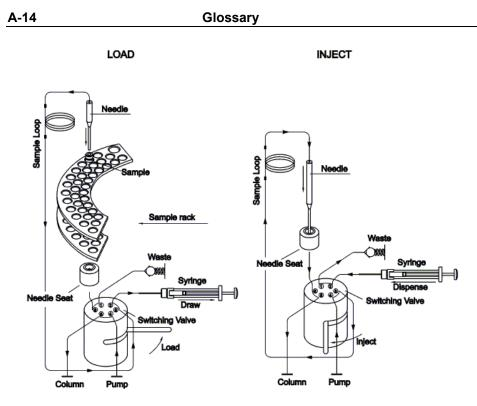
The Dionex Autosamplers Gina 50, Gina 160, ASI-100/ASI-100T, and AS50 function on this basis. Apart from the standard model, a coolable version (Gina 50T) and a model with integrated derivatization or method program (Gina 160) are available. (With the ASI-100/ASI-100T samplers, derivatization and method programming is possible with the standard version.)
