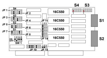
Each physical interface corresponds to a logical interface that is configured via different address combinations (I/O-address). Each logical interface can be assigned to one of a maximum of eight available interrupts.
