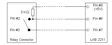
The connection illustrated here for pin 9 must also be installed for the pins 10, 11, 12, 13, and 24 of the LKB connector.
