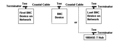
Tips: Link the devices in a single line in any order. The PeakNet6 Workstation can be anywhere in the network. A terminator plug must be installed at each end of the network.
