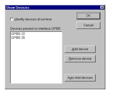
Ensure that the **Identify devices at run-time** checkbox is **disabled** and use the **Add Device** button to manually add the HPIB address you will be using for your module(s). For information on the default HPIB address of each module see the corresponding Agilent manuals.
