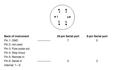
By connecting the pins 1 - 5 on the pump connector, the pump is immediately switched to **Remote** operation after it is switched on!
