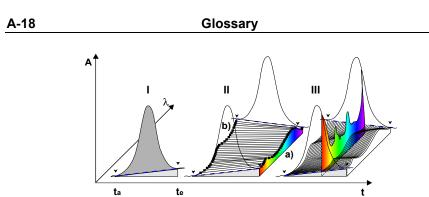
This is performed for all detected wavelengths. The absorption values at all wavelengths measured at the time ta and te result in the baseline spectrum of peak start and peak end (**II**, **a** and **b**). Between these two spectra, the Dionex Chromatography Management System performs an interpolation and thus calculates a separate baseline spectrum for each peak data point. Outside the peak limits, the 3D-field is by definition zero.
