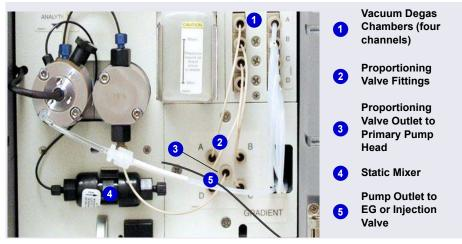
Figure 2-4. Analytical Gradient Pump Components
