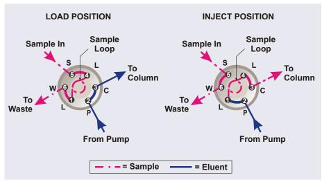
Figure 2-27. Injection Valve Flow Schematics (6-Port Valve)
