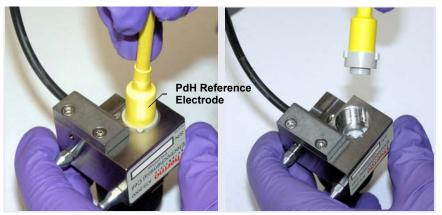
**Figure 9-69.** Removing the PdH Reference Electrode from the Reference Electrode Well
