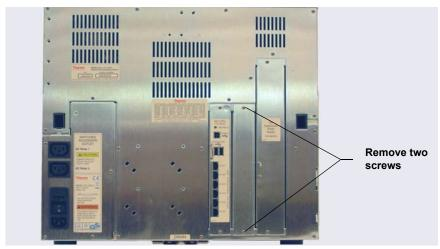
Figure 9-38. DC Rear Panel: Removing the I/O Option Cover Plate
