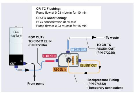
Figure 9-27. Flow Schematic for Flushing and Conditioning the CR-TC (Capillary)
