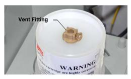
Figure 9-15. Capillary Dionex EGC Vent Fitting
