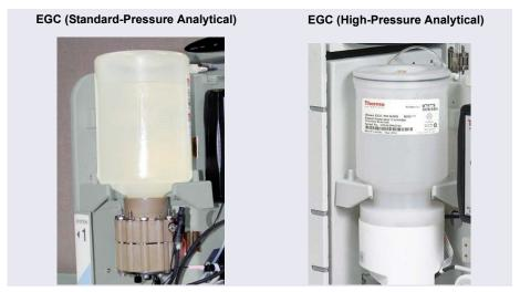
Figure 9-25. Analytical Dionex EGC Installed in Holder
