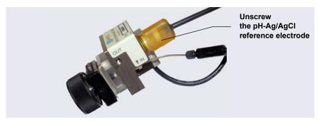
**Figure 9-59.** Removing the pH-Ag/AgCl Reference Electrode (Cell Configured for Analytical IC Shown)
