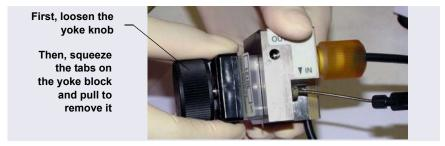
**Figure 9-56.** Disassembling the ED Cell (Cell Configured for Analytical IC Shown)
