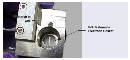
Figure 9-70. Removing the PdH Reference Electrode Gasket
