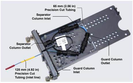
**Figure 9-50.** 150 mm Separator Column and 35 mm Guard Column Installed in Capillary Column Tray
