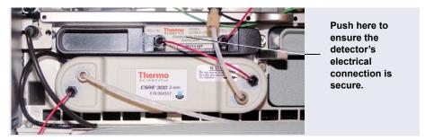
Figure 8-3. Conductivity Detector Connection
