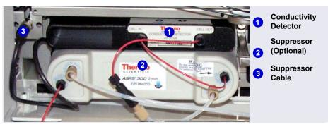
Figure 2-29. Analytical Conductivity Detector with Suppressor (System #1)
