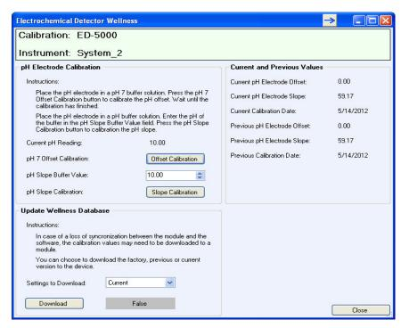
**Figure 9-61.** Wellness Panel: Dionex ICS-5000<sup>+</sup> Electrochemical Detector (Chromeleon 7 Version Shown)
