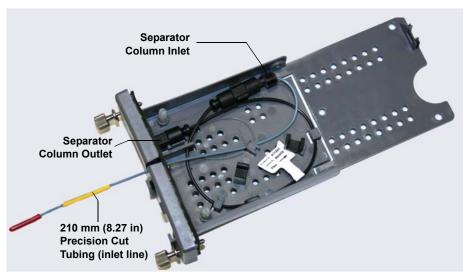
Figure 9-49. 250 mm Separator Column Installed in Capillary Column Tray
