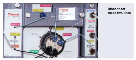
Figure 9-44. Disconnect Capillary Tray Eluent Lines (Conductivity System Plumbing Shown)
