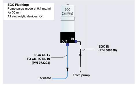
Figure 9-20. Flow Schematic for Flushing the Dionex EGC (Capillary)
