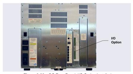
Figure 9-39. DC Rear Panel: I/O Option Installed
