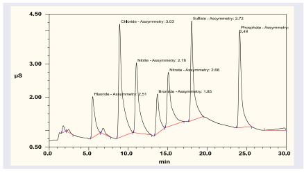
Figure 8-2. Tailing Peaks Caused by Incorrectly Installed
