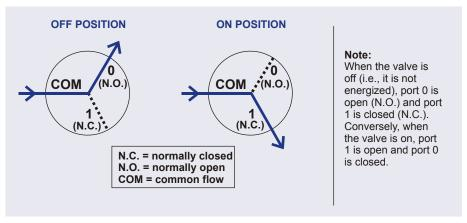
Figure 2-44. Three-Way Low-Pressure Valve Flow Schematics
