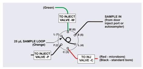
Figure 2-66. Injection Valve Plumbing (6-Port Valve)
