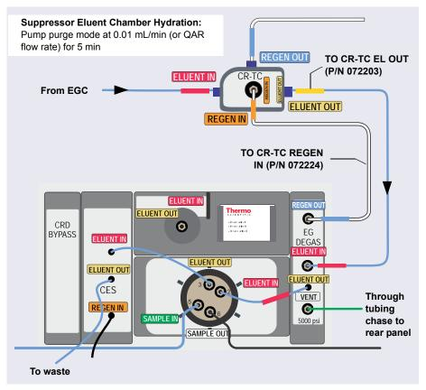
**Figure 9-43.** Flow Schematic for Hydrating the Suppressor Eluent Chamber in a Capillary IC System
