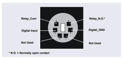
Figure 2-63. Digital I/O Connector
