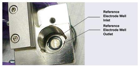
**Figure 9-63.** Reference Electrode Well with Reference Electrode Gasket for Capillary IC Installed
