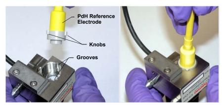
**Figure 9-72.** Inserting the PdH Reference Electrode Fitting into the Reference Electrode Well
