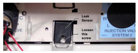
Figure 9-34. Leak Sensor
