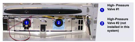
**Figure 8-5.** High-Pressure Valves #1 and #2 (In DC Lower Compartment)
