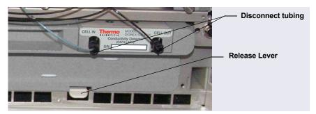
Figure 9-54. Disconnecting the CD Liquid Lines (Capillary CD shown)
