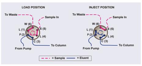
Figure 2-64. TC Injection Valve Flow Schematics (6-Port Valve)
