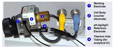
**Figure 2-32.** ED Cell with pH-Ag/AgCl Reference Electrode (Cell Configured for Analytical IC Shown)
