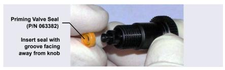
Figure 9-12. Replacing the Priming Valve Seal
