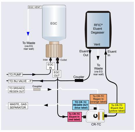
**Figure 2-15.** EG Flow Schematic Example for Standard-Pressure Analytical IC
