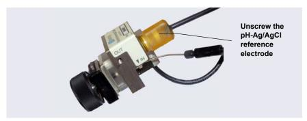
**Figure 9-66.** Removing the pH-Ag/AgCl Reference Electrode (Cell Configured for Analytical IC Shown)
