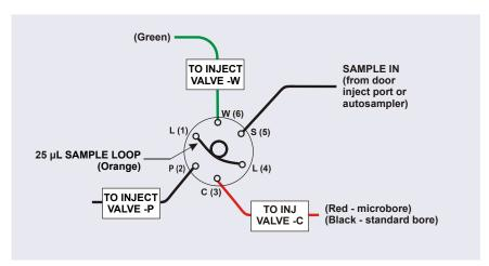
6. Reconnect all liquid lines to the injection valve (see <u>Figure 9-77</u>).
