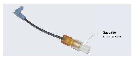
Figure 9-60. pH-Ag/AgCl Reference Electrode in Storage Cap
