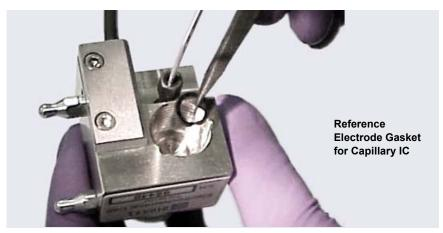
Figure 9-62. Reference Electrode Gasket for Capillary IC
