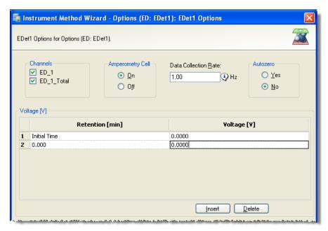
Figure 2-49. DC Amperometry Instrument Method Wizard Page in Chromeleon 7
