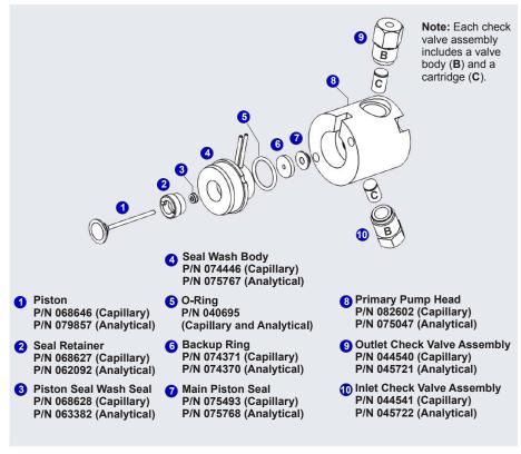
Figure 9-6. DP/SP Pump: Primary Pump Head Assembly
