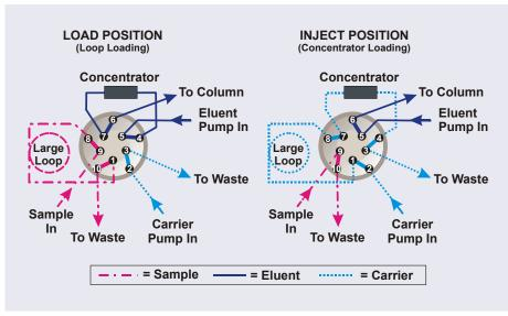
**Figure 2-28.** Injection Valve Flow Schematics (10-Port Valve) Example Connections: Large Loop to Concentrator
