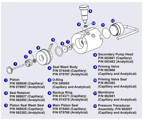
Figure 9-7. DP/SP: Secondary Pump Head Assembly
