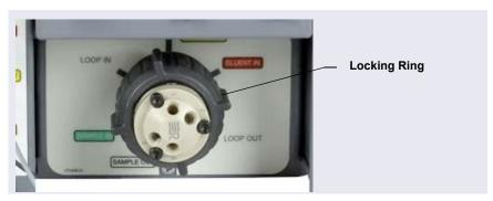
Figure 9-36. Unscrew the Locking Ring (Valve in IC Cube Shown)
