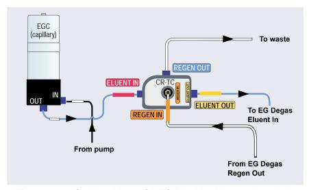
**Figure 9-28.** Capillary Dionex CR-TC Plumbing Diagram: Installation Completed
