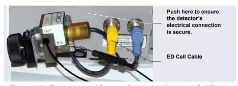
Figure 8-4. Electrochemical Detector Connection (Analytical Cell Shown)
