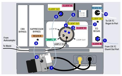
**Figure 2-22.** IC Cube Eluent and Regenerant Flow Schematic for Electrochemical Detection (PdH Electrode Shown)
