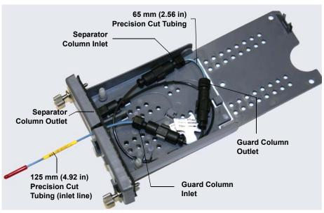
**Figure 9-48.** 250 mm Separator Column and 50 mm Guard Column Installed in Capillary Column Tray
