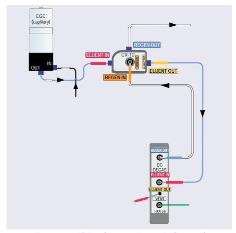
Figure 2-14. EG Flow Schematic Example for Capillary IC
