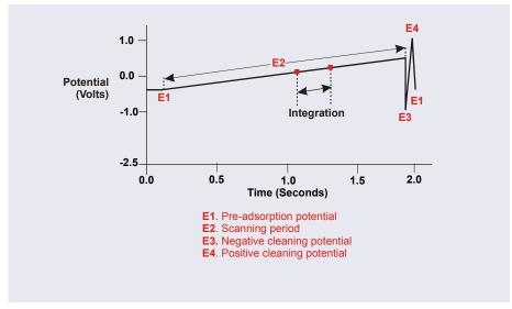
Figure 2-55. Example Scanning Waveform
