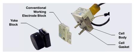
Figure 9-57. ED Cell Components
