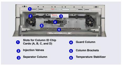
Figure 2-61. TC Interior View (Dual System Configuration Shown)
