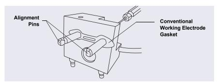
Figure 9-58. ED Cell Gasket for Conventional Working Electrodes
