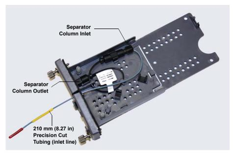
Figure 9-51. 150 mm Separator Column Installed in Capillary Column Tray
