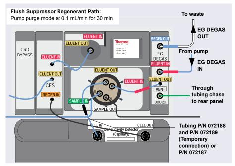
**Figure 9-42.** Flow Schematic for Filling and Flushing the Regenerant Path in a Capillary Suppressor
