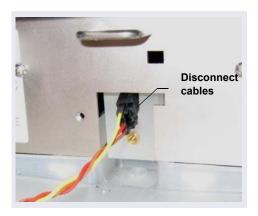
Figure 9-35. Leak Sensor Cable
