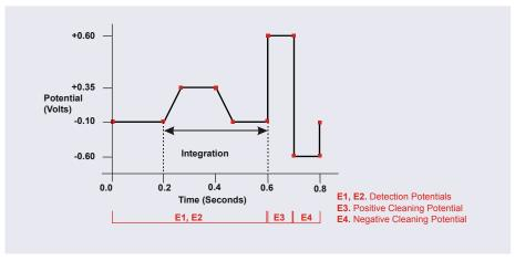
Figure 2-51. Example Integrated Amperometry Waveform
