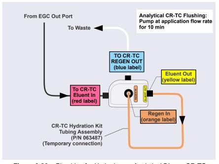
Figure 9-29. Plumbing for Hydrating an Analytical Dionex CR-TC
