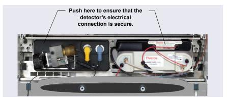
Figure 8-1. Detector Connection
