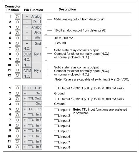
Figure 2-34. Optional Rear Panel I/O Connector Strips
