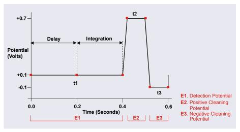
Figure 2-50. Example Pulsed Amperometry Waveform
