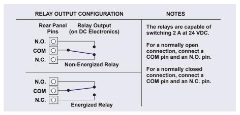
Figure 2-37. Relay Output Configuration
