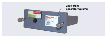
Figure 9-46. Capillary Column Tray with Column Label
