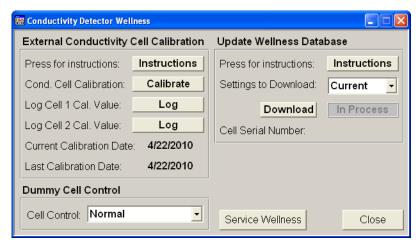
**Figure 9-52.** Wellness Panel: Dionex ICS-5000<sup>+</sup> Conductivity Detector (Chromeleon 6.8 Version Shown)
