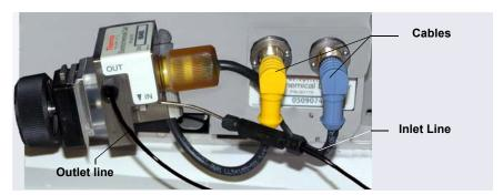
**Figure 9-55.** Disconnecting the ED Cell (Cell Configured for Analytical IC Shown)
