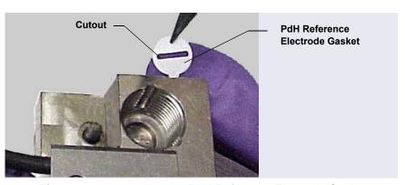
Figure 9-71. Installing the PdH Reference Electrode Gasket
