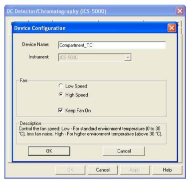
Figure 2-25. Setting the DC Upper Compartment Fan Speed
