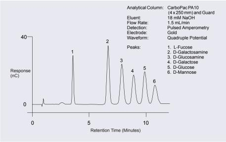
Figure 2-56. Example Chromatogram for a Pulsed Amperometry Application
