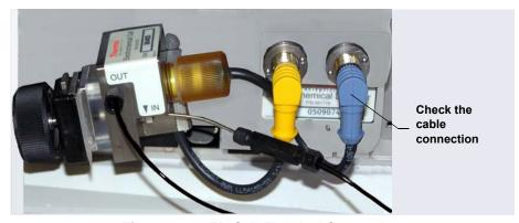
Figure 8-8. ED Cell Electrical Connections
