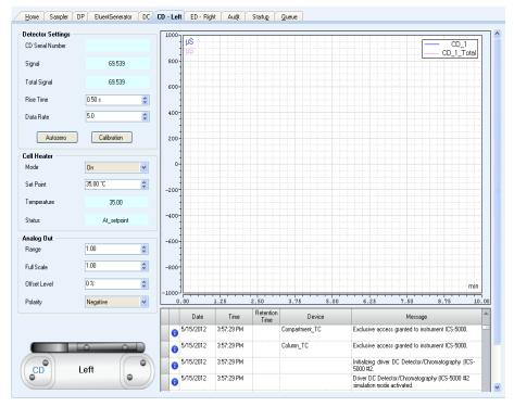
**Figure 2-36.** Conductivity Detector Control Panel (Chromeleon 7 Version Shown)
