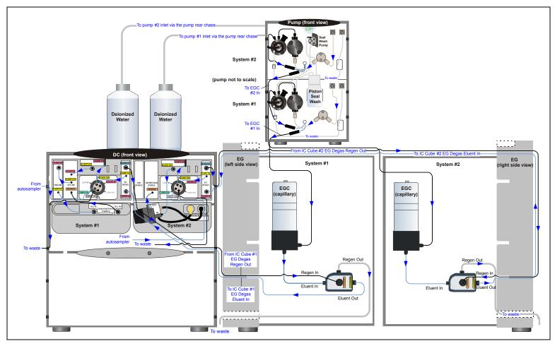
Figure 3-1. Capillary IC: Dual RFIC-EG System (CD/CD)
