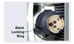
Figure 9-78. Unscrewing the Locking Ring
