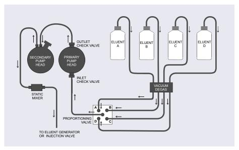
Figure 2-6. Gradient Pump Flow Schematic
