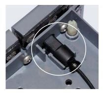
Figure 9-45. Separator Column Outlet Fitting
