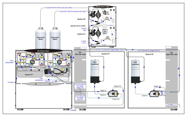
Figure 3-2. Capillary IC: Dual RFIC-EG System (CD/ED)
