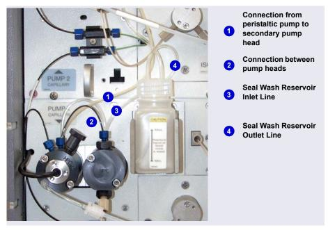
Figure 4-5. Piston Seal Wash Connections to Pump 1
