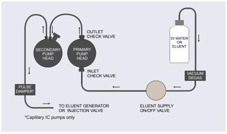
Figure 2-5. Isocratic Pump Flow Schematic
