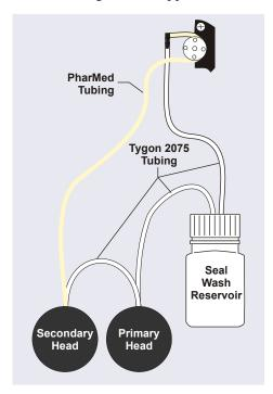
Figure 9-10. Piston Seal Wash Tubing Connections
