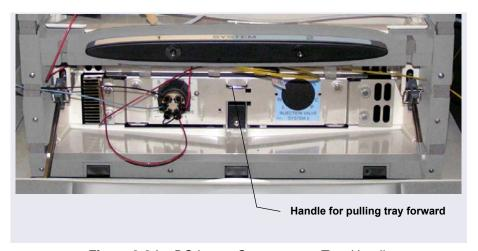
Figure 2-24. DC Lower Compartment Tray Handle
