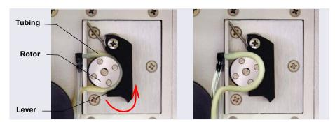
Figure 6-1. Peristaltic Pump for Seal Wash System
