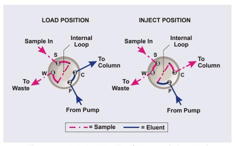
Figure 2-26. Injection Valve Flow Schematics (4-Port Valve)
