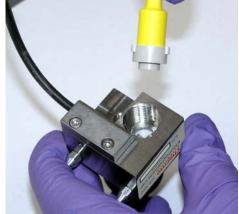
4. Using tweezers, remove the PdH reference electrode gasket from the well (see Figure 107).
