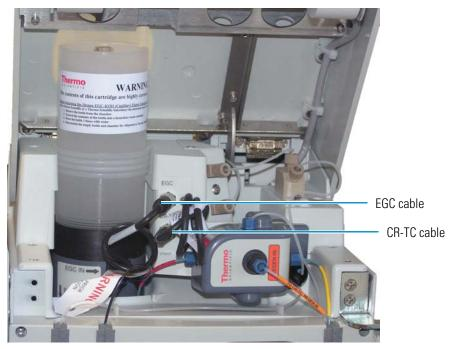
2. If the error appears again, the CR-TC may be faulty. Replace the CR-TC (see "Replacing a CR-TC" on page 143).
