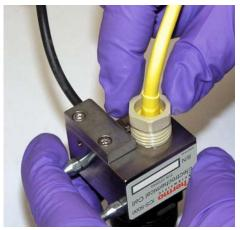
3. Pull the reference electrode out of the well (see Figure 106).
