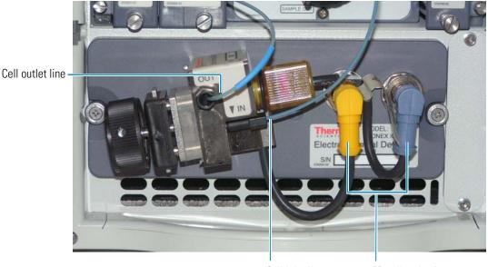
**Figure 93.** ED cell connections (cell with pH-Ag/AgCl reference electrode shown)
