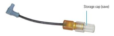
**IMPORTANT** Always store the electrode in the storage cap filled with saturated KCl solution when the cell is not in use. This prevents the pH-Ag/AgCl reference electrode membrane from drying out and damaging the electrode. For storage instructions, see page 48.
