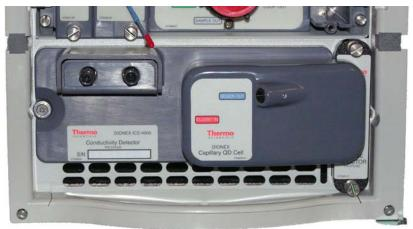
Figure 91. Dionex QDC 300 (Capillary) installed on Dionex ICS-4000 Conductivity Detector
