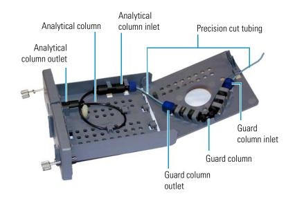
Figure 81. Analytical and guard columns installed in column cartridge
