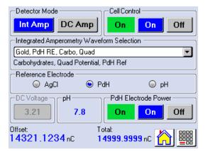
Figure 48. ED screen (integrated amperometry mode)
