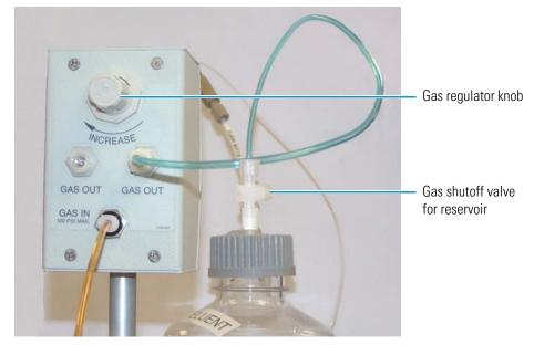
Figure 21. Gas connections to the regulator and reservoir
