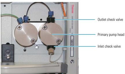
Figure 62. Pump components
