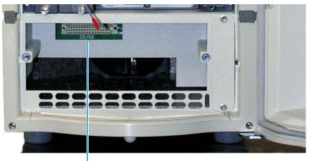
Figure 90. Lower section of the chromatography compartment without a detector
