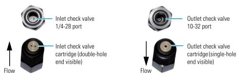
**Note** For correct pump operation, the check valve cartridges must be installed in their respective housings in the correct orientation. Liquid enters through the check valve in the large single hole and exits through the small double holes.
