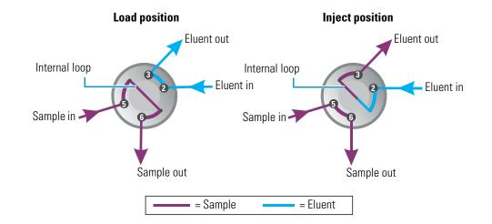
Figure 12. Injection valve flow schematics (4-port valve)
