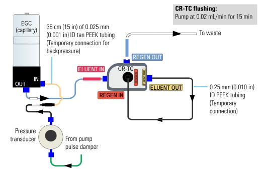
Figure 77. Flow schematic for flushing the CR-TC
