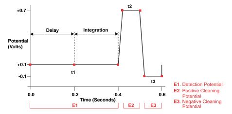
Figure 29. Example pulsed amperometry waveform
