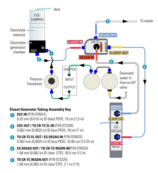
Figure 69. Eluent generator flow schematic (after setup is complete)
