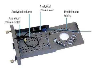
7. Lift up the analytical column outlet fitting (see Figure 83) slightly to free it from the clips and then slide the fitting out of the cartridge.
