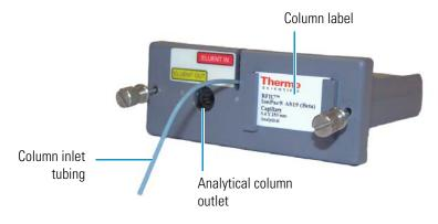
**Note** If the columns are installed correctly, the cartridge lid snaps closed easily. If the lid does not close easily, do not force it. Open the lid and verify that the columns and tubing are installed correctly and secured in the clips.
