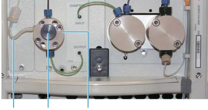
Priming Priming valve Pressure transducer waste line
