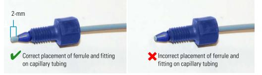
2. Insert the tubing into the port until it stops.
