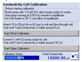
Figure 88. Conductivity Cell Calibration touch screen
