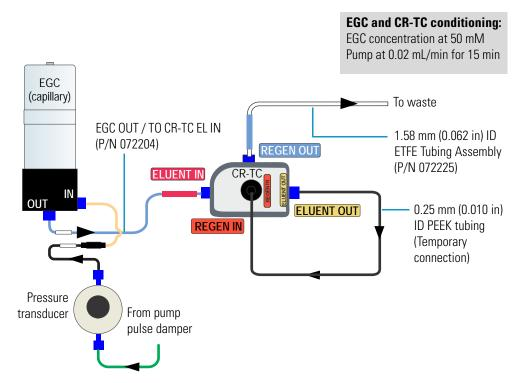
Figure 75. Flow schematic for conditioning the EGC
