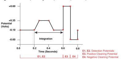
**Figure 30.** Example integrated pulsed amperometry waveform
