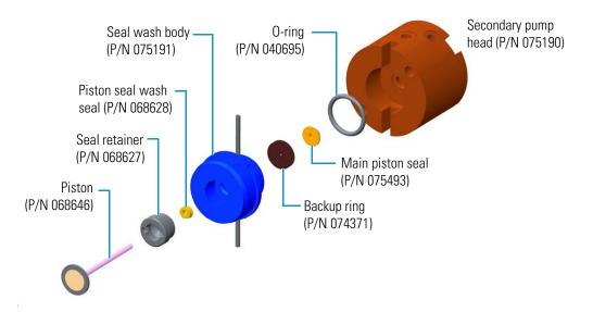
**Figure 65.** Secondary pump head assembly
