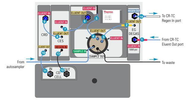
Figure 15. Dionex IC Cube flow schematic for conductivity detection (shown with optional CRD)
