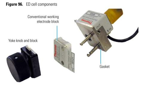
Use tweezers to remove the old cell gasket from the cell body (see Figure 97).
