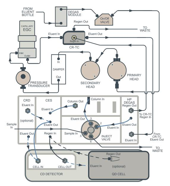
• Deionized water from the reservoir flows first through the eluent degas assembly and then through the eluent valve to the pump. The water is then pushed through a pulse damper, which smooths minor pressure variations from the pump to minimize baseline noise. From there, the water flows through the pressure transducer, which measures the system pressure.
