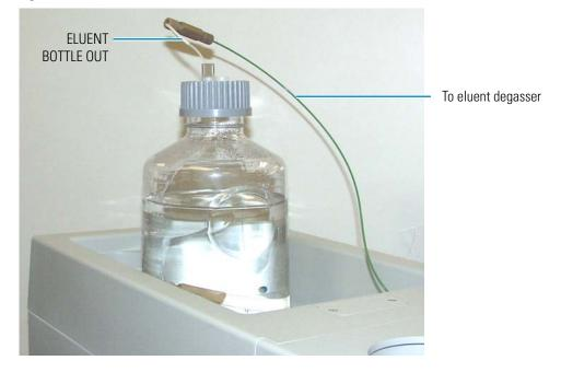
Figure 20. Eluent reservoir connections (reservoir P/N 075313 shown)
