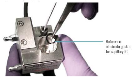
Figure 102. pH-Ag/AgCl reference electrode O-ring
