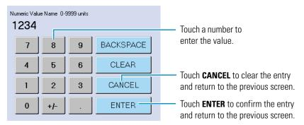
**Tip** The background color on some controls indicates the status of the corresponding device.
