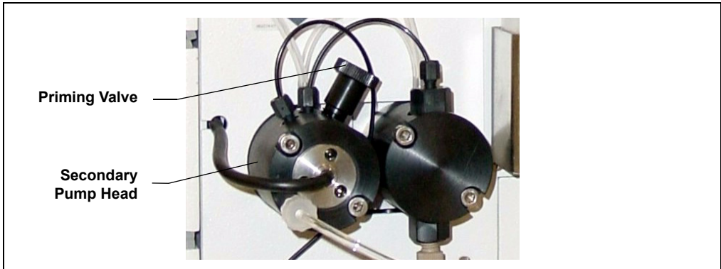
Figure 9-9. DP/SP Priming Valve
