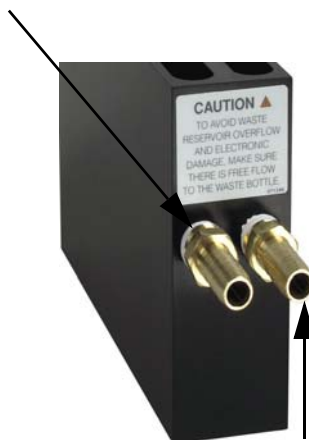
Figure B-7. Waste Tubing Connections
