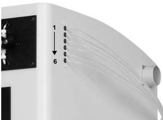
Figure 3-4. Dionex AutoTrace 280 Sample Inlet Ports
