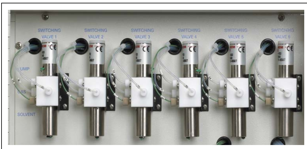
Figure 5-17. Switching Valve Compression Fittings
