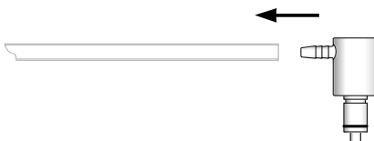
Figure B-10. Barbed Fitting on Tubing
