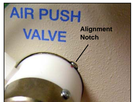
Figure 5-16. Air Push Valve Alignment Notch
