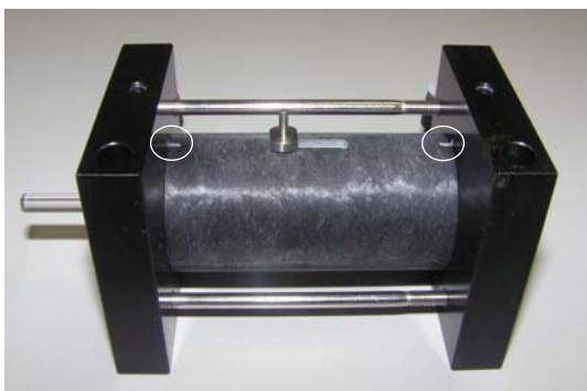
Figure 5-15. Alignment Marks on Pump Cylinder and End Plates
