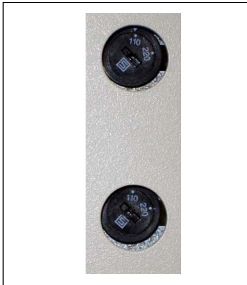
Figure B-3. Oven Voltage Switch Settings (110 Voltage Setting Currently Selected)
