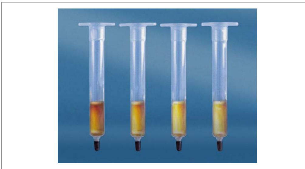
Figure E-4. Residual co-extractives after the ASE extraction of a coffee sample trapped on an SPE cartridge, the ASE cells containing varying from 0 to 6 g Florisil. From left to right: 1) No Florisil in the ASE cell, 2) 2 g Florisil in the ASE cell, 3) 4 g Florisil in the ASE cell, and 4) 6 g Florisil in the ASE cell
