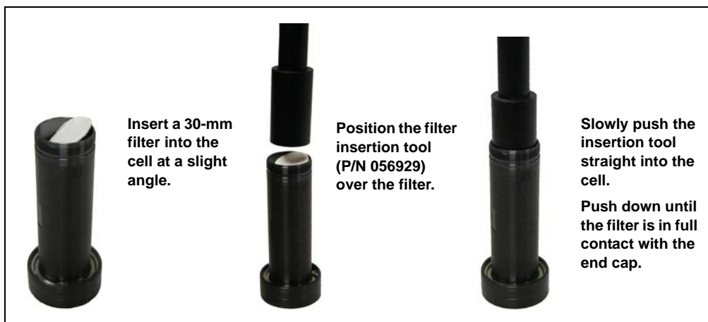
Figure 3-6. Installing a 30-mm Cell Filter in a 34-mL, 66-mL, or 100-mL Cell
