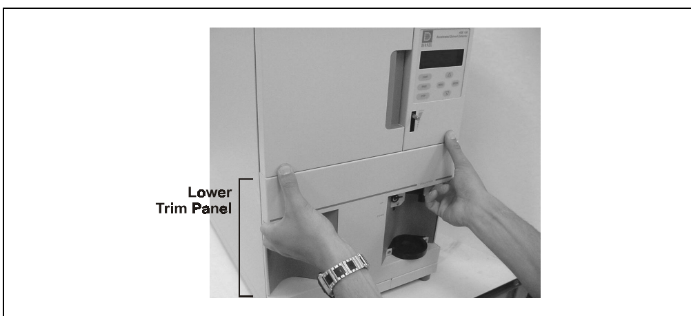
Figure 5-3. Removing the Lower Trim Panel
