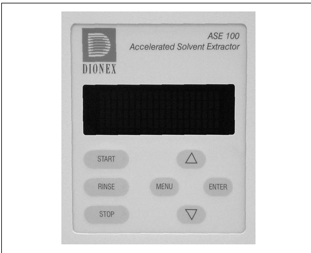
Figure 2-2. ASE 100 Control Panel
