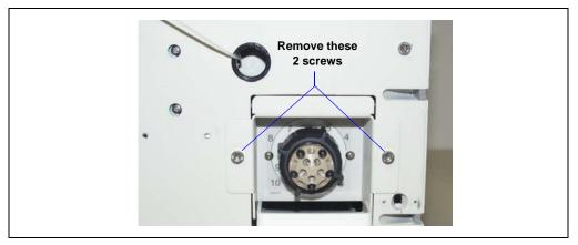
Figure 5-13. Removing the Valve Assembly
