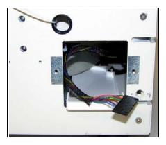
6. Press the cable's locking latch and insert the cable into the connector on the valve until you hear a click.
