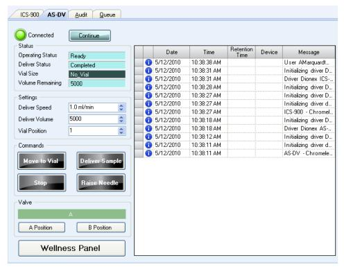
Figure 2-12. Chromeleon 7 ePanel Set: Dionex AS-DV ePanel
