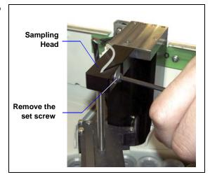
Figure 5-8. Removing the Set Screw
