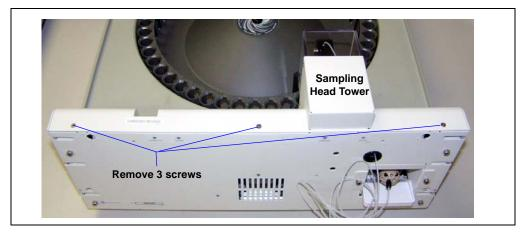
Figure 5-7. Removing the Sampling Head Tower Cover
