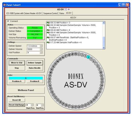
Figure 3-5. Example Chromeleon 6.8 Panel Tabset: Dionex AS-DV Control Panel
