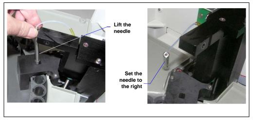
8. Lift the needle out of the carousel and set it to the right (see <u>Figure 5-4</u>).
