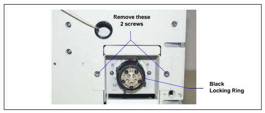
Figure 5-15. Removing the Valve Assembly
