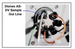
Figure B-3. IC System Injection Valve
