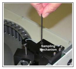
Figure 5-11. Manually Raising the Sampling Head
