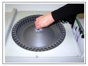
Figure 5-6. Removing the Carousel
