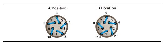
Figure 2-9. Optional 10-Port High-Pressure Valve Flow Schematics
