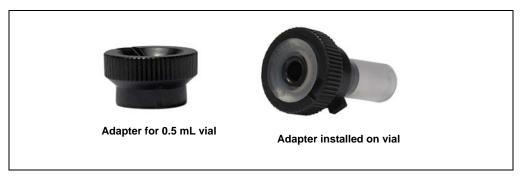
Figure 2-3. Vial Adapter for 0.5 mL Vials
