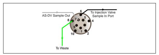
Figure B-7. 10-Port Valve Plumbing for Bleed Valve
