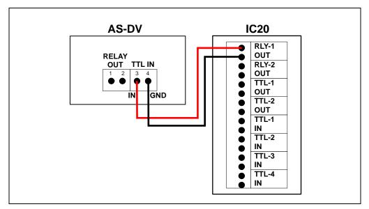
Figure C-4. Example TTL Input Connection: Dionex AS-DV Connected to Dionex IC20
