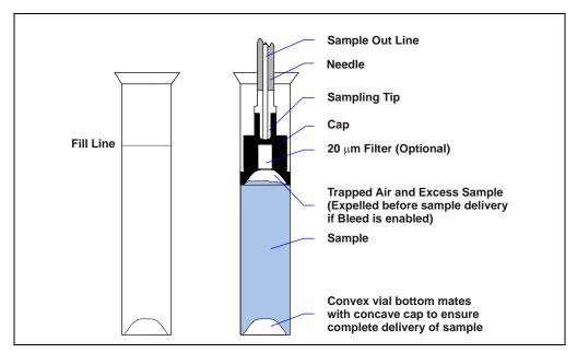
Figure 2-7. PolyVial, Cap, and Sampling Tip Features
