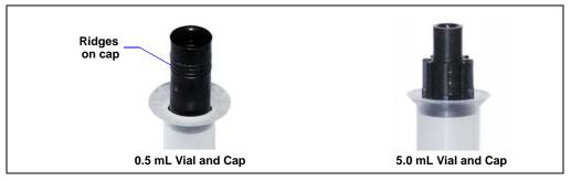
Figure 3-2. Caps Partially Inserted in Vials
