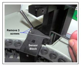
Figure 5-5. Removing the Sensor Block
