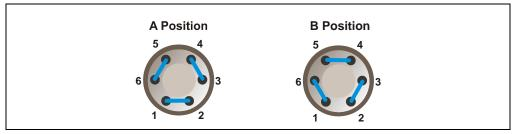
Figure 2-8. Optional 6-Port Hlgh-Pressure Valve Flow Schematics
