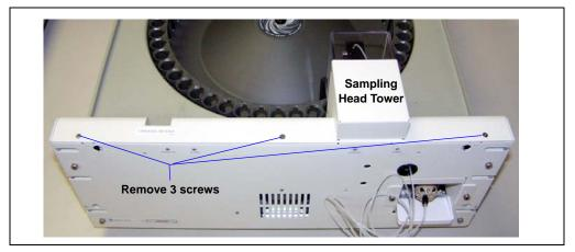
Figure 5-10. Removing the Sampling Head Tower Cover
