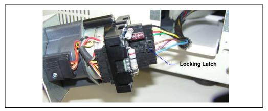
Figure 5-16. Disconnecting the Valve Cable
