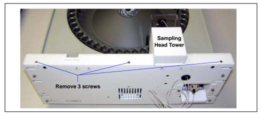
Figure 5-1. Removing the Sampling Head Tower Cover
