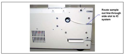
1. Route the sample out line through the side slot in the Dionex AS-DV chassis. Leave a little slack in the tubing.
