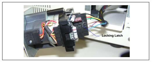
Figure B-4. Connecting the Valve Cable
