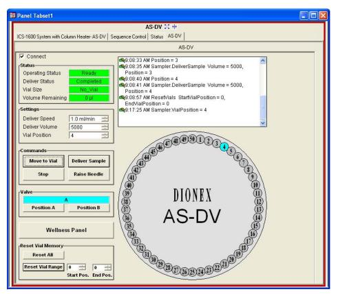
Figure 2-13. Chromeleon 6.8 Panel Tabset: Dionex AS-DV Control Panel
