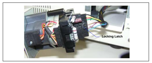
Figure 5-14. Disconnecting the Valve Cable
