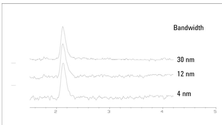
**Figure 36** Influence of Bandwidth on Signal and Noise
