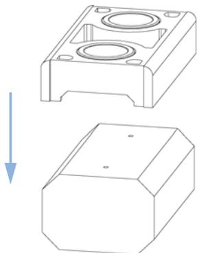
**8** Slide the quartz body completely into the cell body to the front stop (use for example a toothpick).
