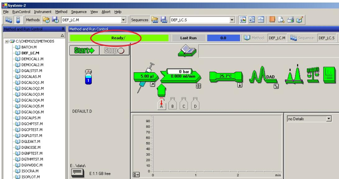
Figure 16 Turning on the HPLC Module
