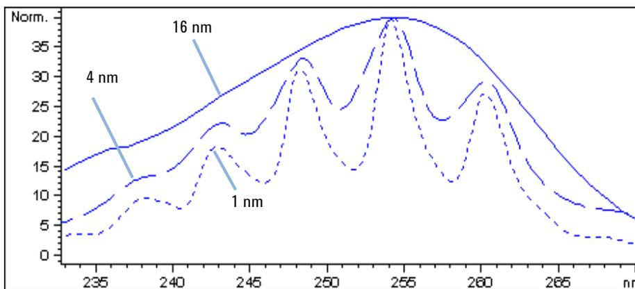
**Figure 38** Benzene at 1, 4 and 16 nm slit width (principle)
