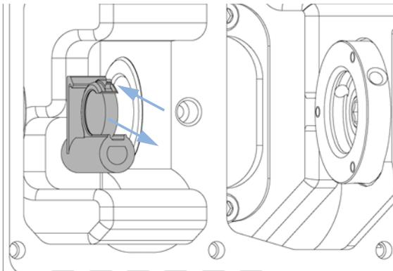
4 While releasing the holder with a screw driver, carefully insert the holmium oxide filter.
