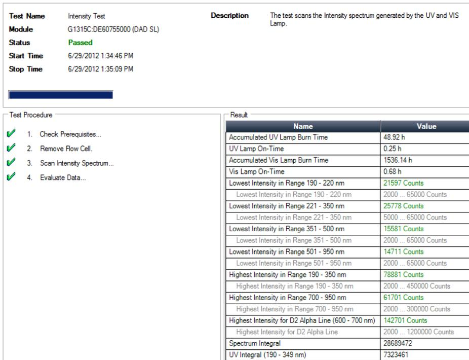
Figure 49 Intensity Test
