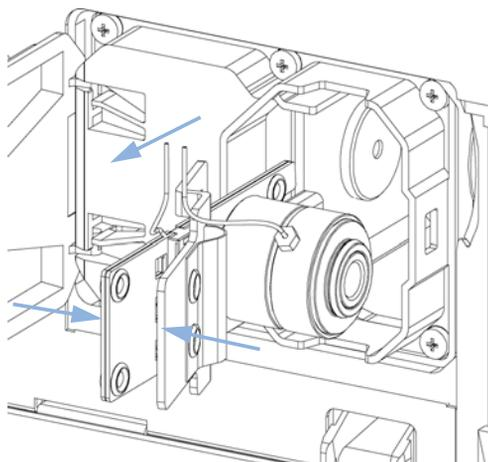
6 Insert the flow cell while pressing the flow cell holder.
