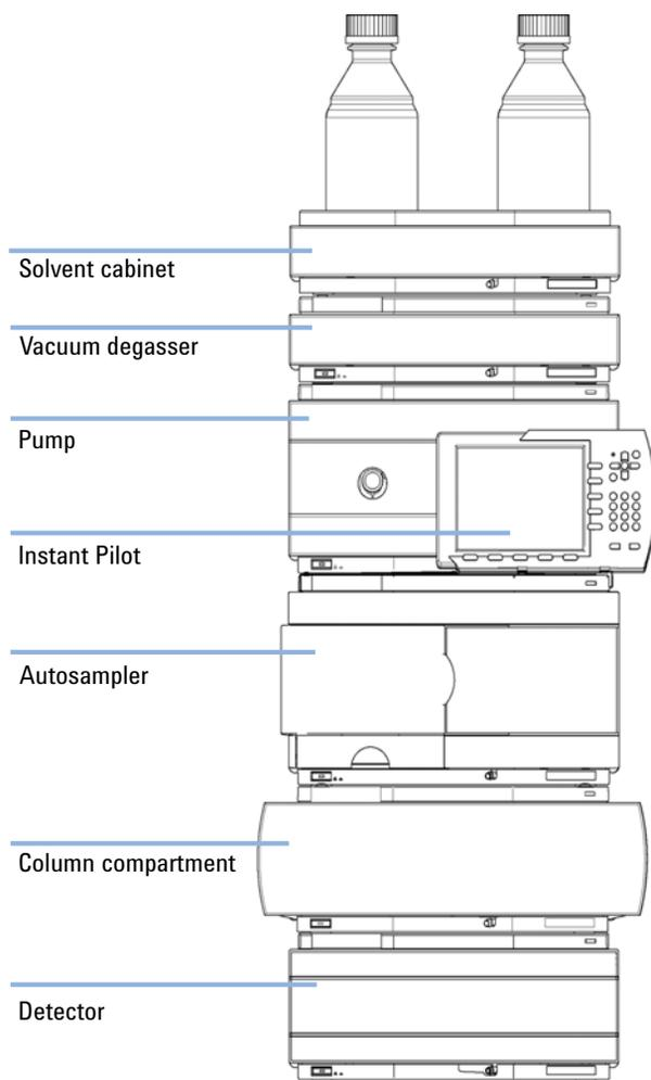
**Figure 3** Recommended Stack Configuration for 1260 Infinity (Front View)
