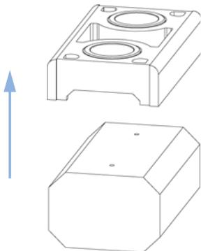
**6** This figure shows the correct holding of the quartz body and the cell seal assembly.
