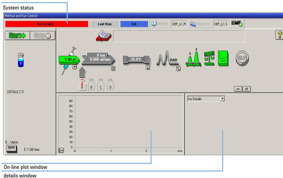
Figure 15 Initial ChemStation screen (Method and Run Control)
