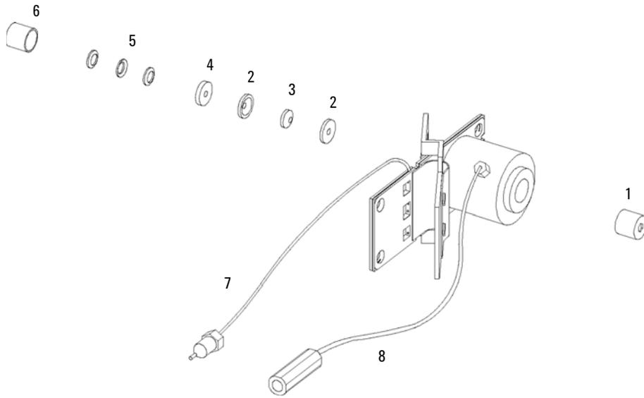
**Figure 77** High pressure flow cell - parts
