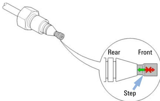
**Figure 106** Capillary fitting
