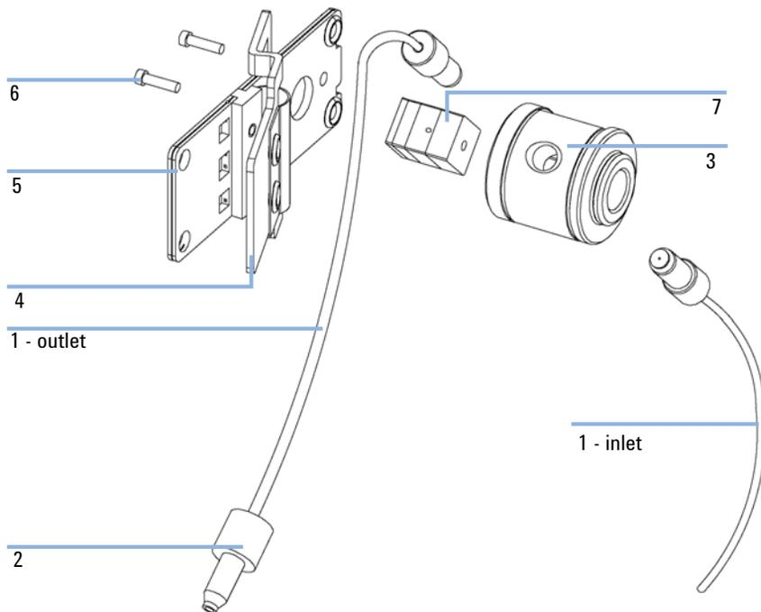
**Figure 75** Prep Flow Cell - Quartz Parts
