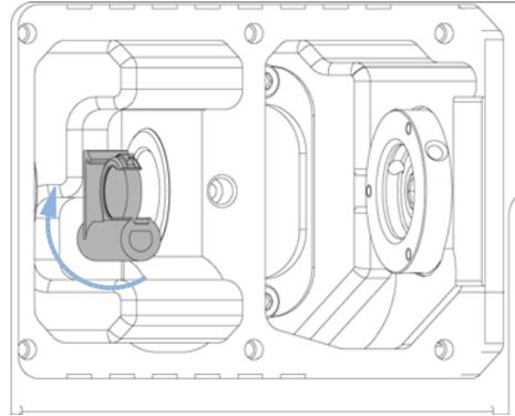
3 While releasing the holder with a screw driver (at the top), carefully remove the holmium oxide filter.
