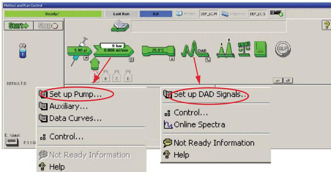
**Figure 19** Open the module menu
