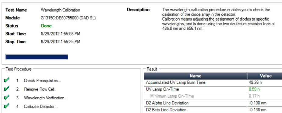
Figure 59 Wavelength Calibration
