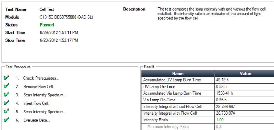
Figure 54 Cell Test
