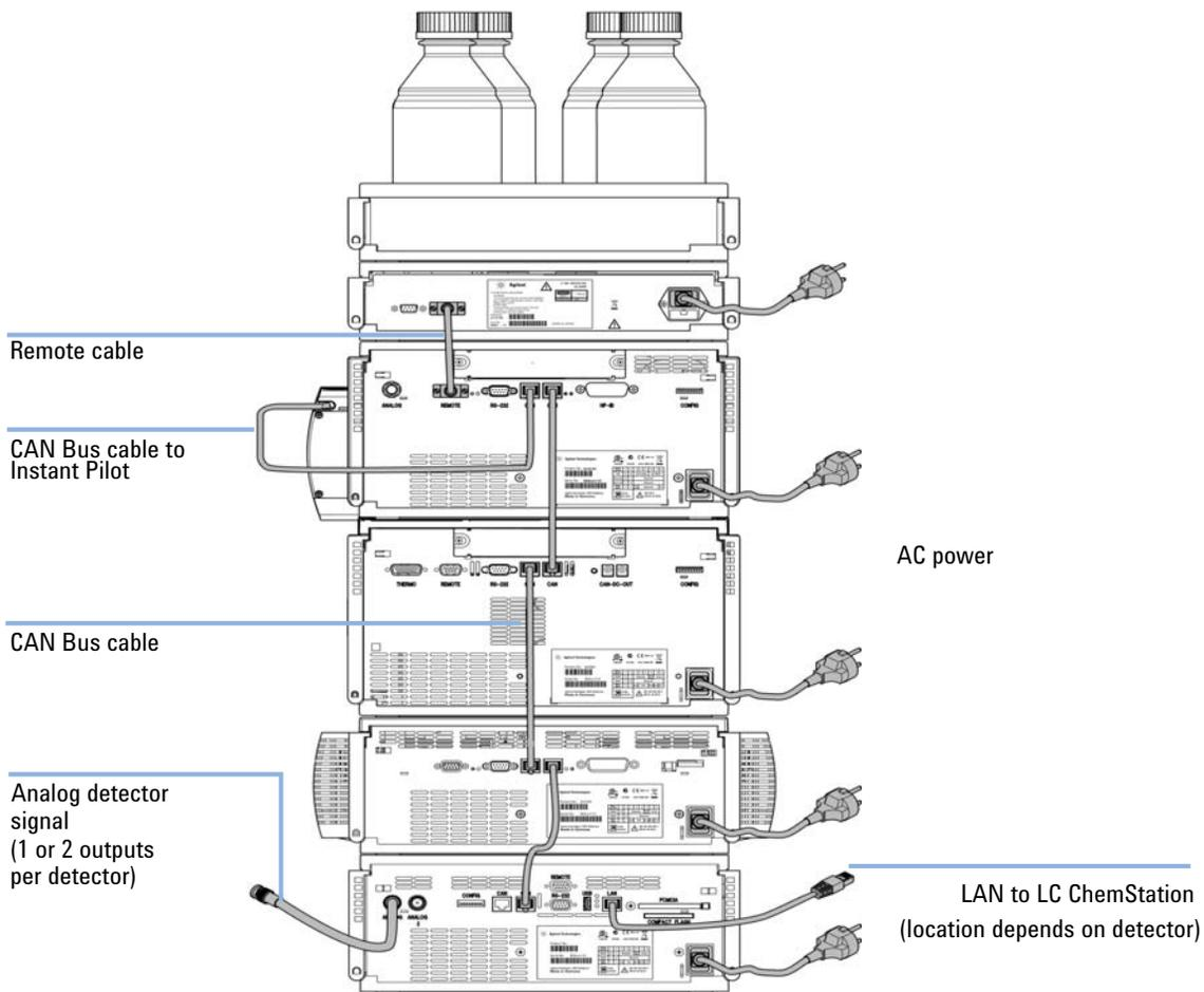
**Figure 4** Recommended Stack Configuration for 1260 Infinity (Rear View)
