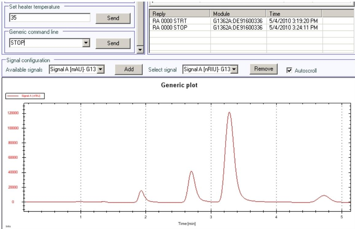
Figure 56 Test Chromatogram with Agilent Lab Advisor
