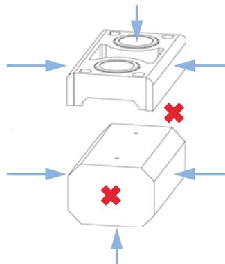
**7** Replace the cell seal assembly onto the quartz body. Always use a new seal assembly to exclude damage during disassembling.
