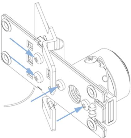
**14** Fix the inlet capillary to the flow cell body handtight first. Then do a 1/4 turn with a 4-mm wrench.
