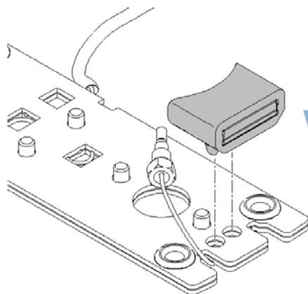
**13** Fix the heat exchanger to the clamp unit and the flow cell body to the heat exchanger.
