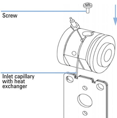
**12** Carefully insert the I.D. tag into the new heat exchanger. Shown is the default orientation. See Note at the beginning of this section.
