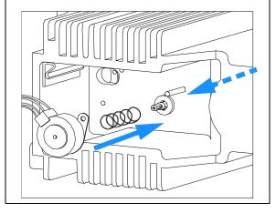
**3** Before installing the filter motor, press the filter lever in from the other side.
