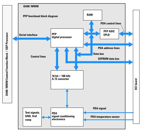
Figure 60 Block Diagram PFP Functions
