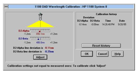
Figure 20 Wavelength Calibration
