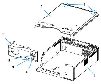
Figure 50 Sheet Metal Kit Parts (G1315B/G1365B)
