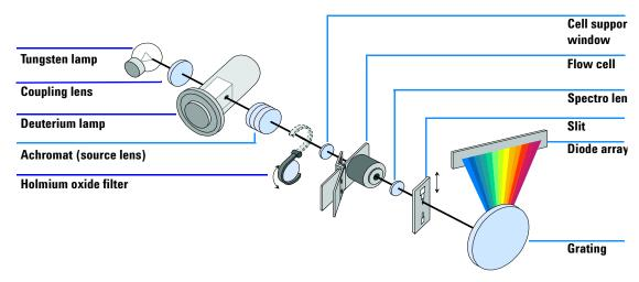
Figure 57 Optical System of the Detector
