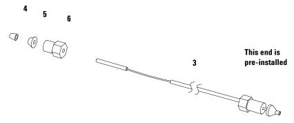
Figure 56 Inlet Capillary (Column-Detector) Parts
