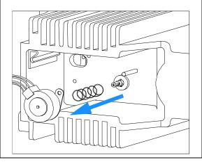
**4** While counter-holding the filter lever, press the filter motor onto the filter shaft until it clicks into the final position.
