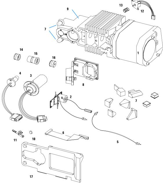
Figure 36 Optical Unit Parts
