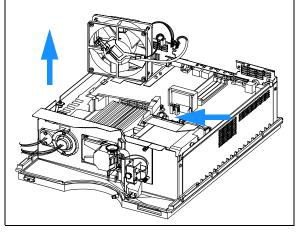
The heater and temperature sensor assemblies are clipped into the fan assembly. In case the temperature sensor or the heater assembly fails, they can be unclipped separately from the fan assembly.
