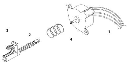
Figure 44 Holmium Oxide Filter Parts
