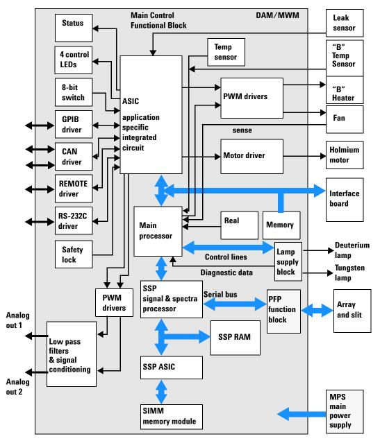
Figure 59 Block Diagram Detector Main Controller Functionality
