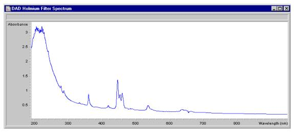
Figure 21 Holmium Oxide Test
