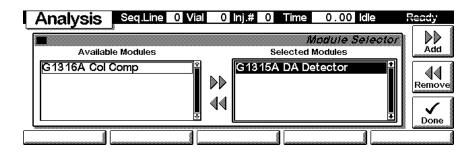
Here, e.g. the column compartment parameters are shown on the display as well. The number of parameters on the display are restricted as additional modules are added. Maximum 4 modules are shown automatically. If more modules are in the system, you have to chose in Setup view.
