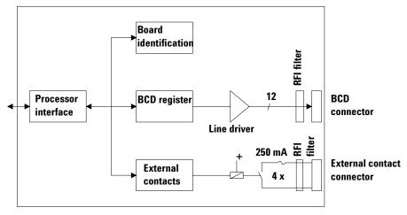
Figure 64 Block Diagram BCD Board
