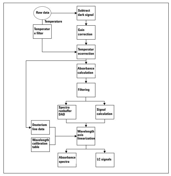
Figure 63 Firmware Flow Diagram
