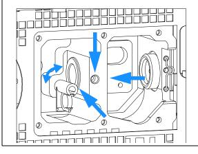
**13** While counter-holding the filter lever, insert the filter motor onto the filter shaft until it clicks into the final position.
