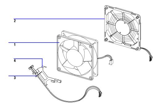
Figure 43 Fan Assembly Parts
