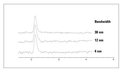
Figure 11 Influence of Bandwidth on Signal and Noise
