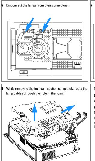
Remove the two lamp connectors towards the back by depressing their connector tabs with a screwdriver.
