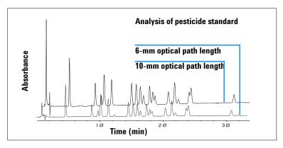
Figure 8 Influence of Cell Path Length on Signal Height
