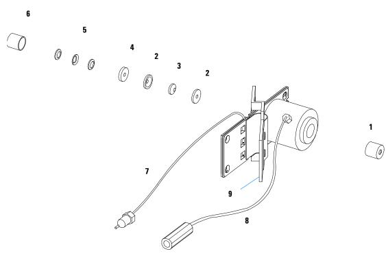
Figure 41 High Pressure Flow Cell Assembly Parts
