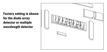
Figure 66 8-bit Configuration Switch
