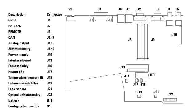
Figure 34 Location of Connectors on Detector Main Board
