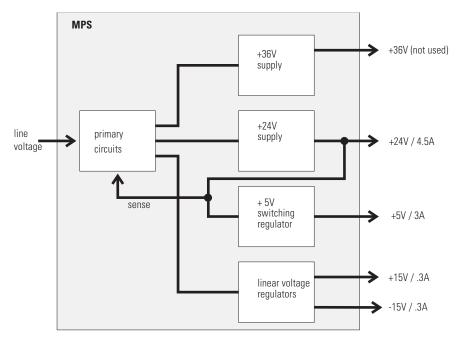
Figure 67 Main Power Supply (MPS) Blockdiagram
