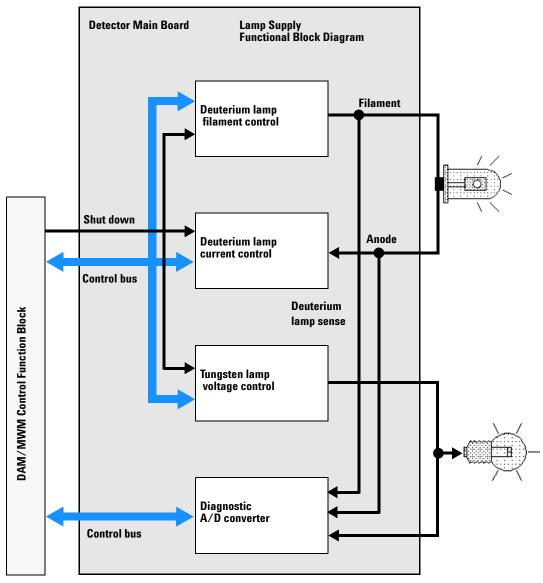
Figure 61 Block Diagram Lamp Supply Functions
