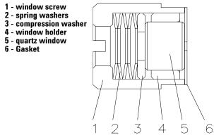
Figure 40 Orientation of Spring Washers.
