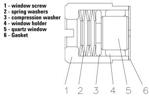
Figure 38 Orientation of Spring Washers.
