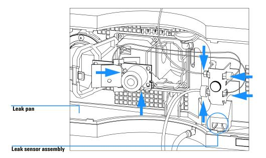
Figure 31 Observing for Leaks
