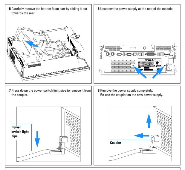
The repair level of the power supply assembly is exchange of the complete assembly. No serviceable parts inside.
