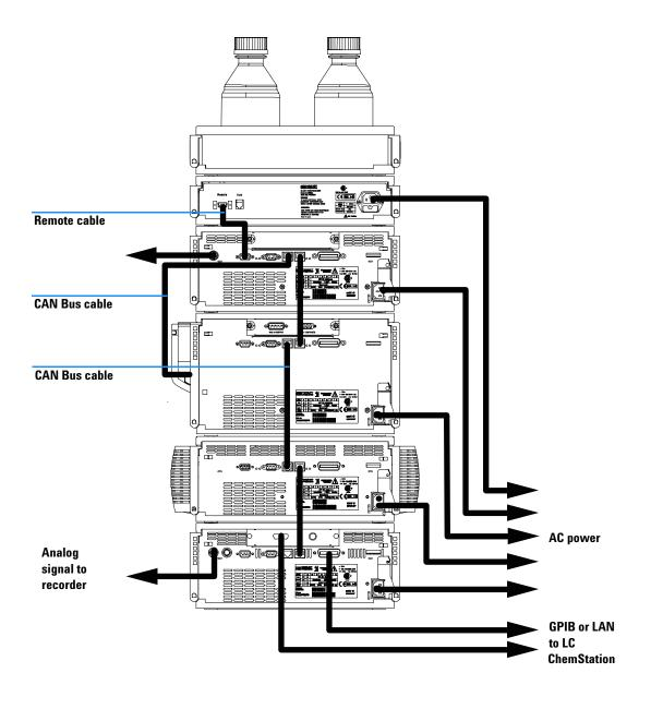
Figure 4 Recommended Stack Configuration (Rear View)
