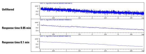
Figure 9 Influence of Response Time on Signal and Noise
