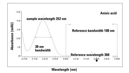
**Figure 10** Optimization of Wavelength Setting
