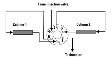
Figure 3 Micro column switching valve connections
