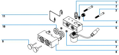
Figure 9 Pump head assembly
