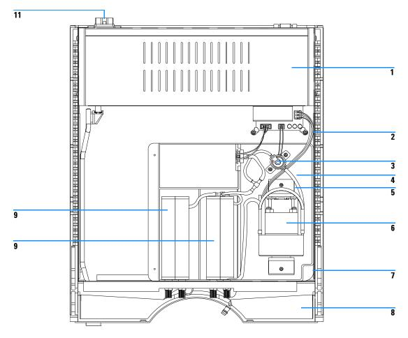
Figure 4 Micro vacuum degasser main assemblies
