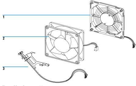
Figure 32 Fan assembly parts
