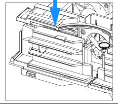
**6** Press down completely until it clicks into its holding position.
