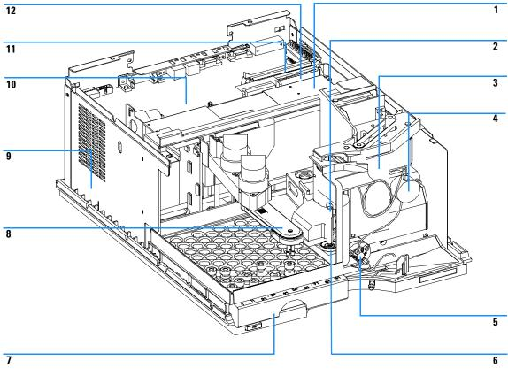
Figure 17 Thermostatted micro autosampler main assemblies
