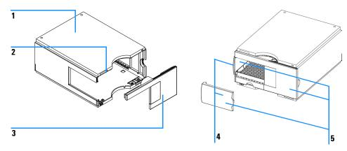
Figure 22 Thermostatted micro autosampler cover parts
