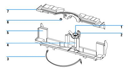
Figure 28 Thermostatted column compartment leak parts
