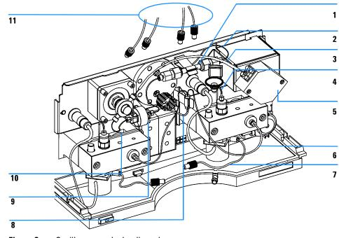
**Figure 8** Capillary pump hydraulic path
