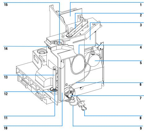
Figure 19 Sampling unit for the micro autosampler
