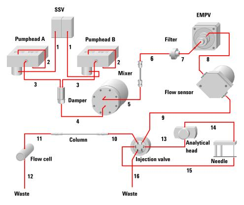
Figure 2 Capillary flow diagram of the Agilent 1100 system capillary LC system
