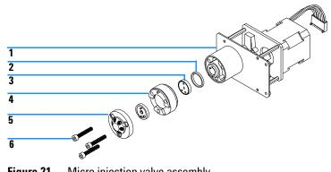
Figure 21 Micro injection valve assembly
