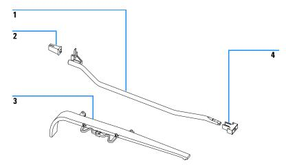
Figure 37 Power and Status Light Pipes
