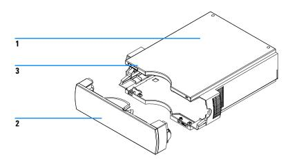
Figure 27 Thermostatted column compartment cover parts
