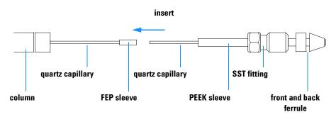
Figure 47 Connecting small i.d. capillaries
