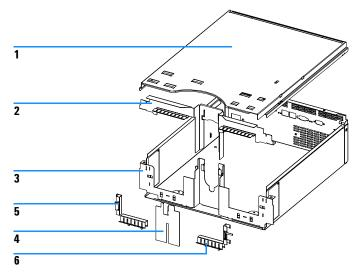
Figure 26 Thermostatted column compartment sheet metal kit
