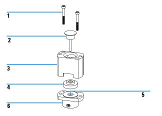
Figure 20 Micro analytical head assembly
