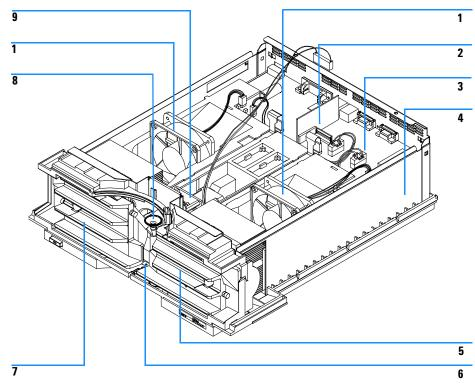
Figure 24 Thermostatted column compartment main assemblies
