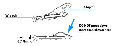
Figure 46 Wrench plus Torque Adapter
