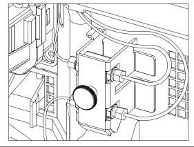
Remove the flow cell and perform a leak test.
