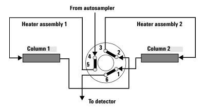
Figure 42Precolumn back-flushing
