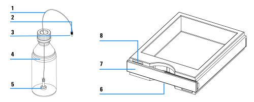
Figure 7 Solvent cabinet and bottle head assembly
