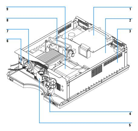
Figure 29 Diode array detector main assemblies
