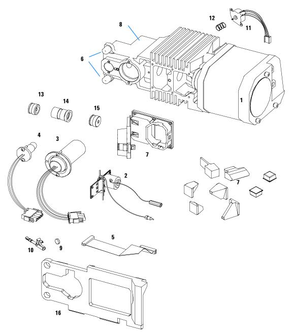
Figure 30 Optical Unit Parts
