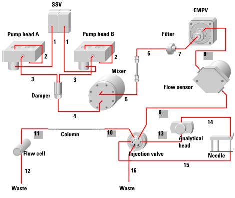
Figure 39 Capillary pump flow diagram
