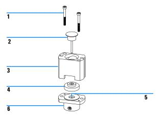
Figure 13 Micro analytical head assembly
