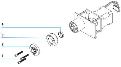
Figure 43 Micro column switching valve
