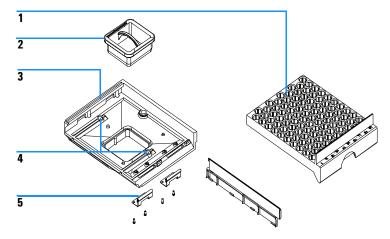
Figure 23 Thermostatted autosampler vial trays and tray base
