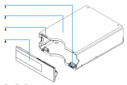
Figure 34 Diode array detector cover parts
