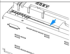
**7** Refit the connector screws and reconnect all connectors.
