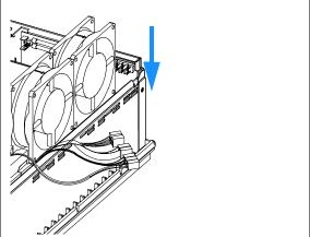
Reinsert the Top Foam and route the cables in the guide channels in the Top Foam.
