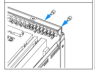
8 Replace the top foam section, metal cover and top cover.
