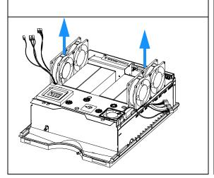
**2** Replace the defective fan, and reinsert the pair of Fans. Note the orientation of the fans.
