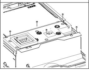
**9** Route the cables in the guide channels and reconnect the connectors in the correct order (See label on Power Supply).
