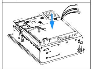
Reconnect the connectors in the correct order (See label on top of Power Supply).
