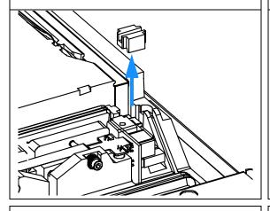
**4** Unplug the connectors at the TCA Board, careful lift the sensors out of their seat and remove the sensor flexboard.
