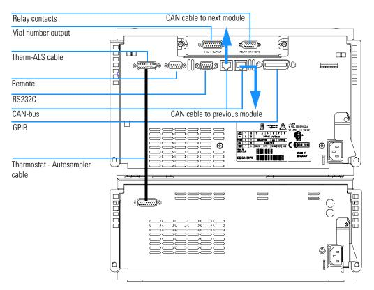
• The GPIB connector is used to connect the thermostatted autosampler with a computer. The address and control switch module next to the GPIB connector determines the GPIB address of your thermostatted autosampler. The switches are preset to a default address (see Autosampler Reference Manual) and this is recognized immediately after power on.
