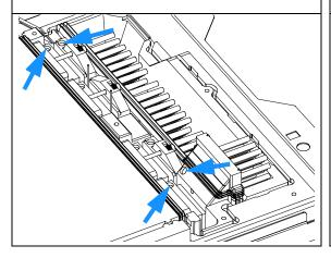
**6** Install the new sensor flexboard carefully by pressing each sensor individually into the seats, and then route the flexboard through the sealing adapter channel.
