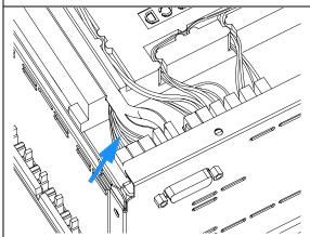
**2** Carefully lift the Fan upwards.
