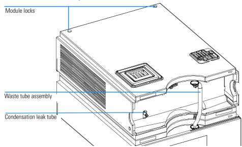
4 Connect the condensation leak tube to the main waste exit of the ALS thermostat and place into an appropriate vessel. It is possible to either let the condensation leak tubing exit the module at the front or at the left side of the module. Make sure that the leak tube is fully fixed on the outlet.
