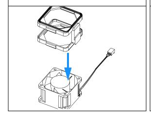
**4** Insert the new Fan in the Fan Gasket. See arrow at the side of Fan for correct airflow direction.
