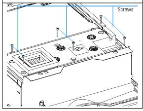
**2** Carefully lift the upper part of hardfoam encapsulation away.
