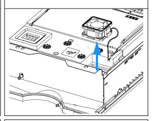
3 Remove the Fan from the Fan Gasket.
