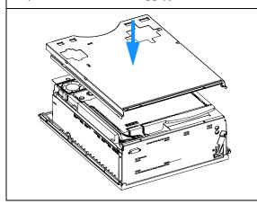
10 Reinstall the Top Plate and the Top Cover.
