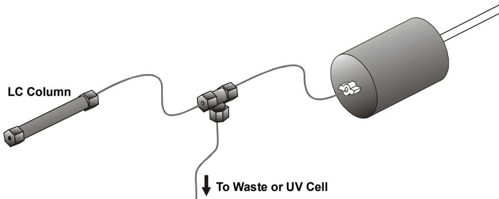
Figure 6-2 Post-column Splitting
