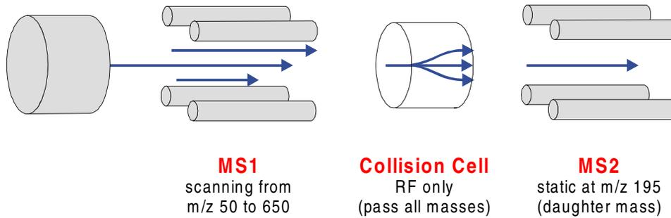
Figure 1-5 MS-MS Mode - Obtaining a Parent Ion Spectrum
