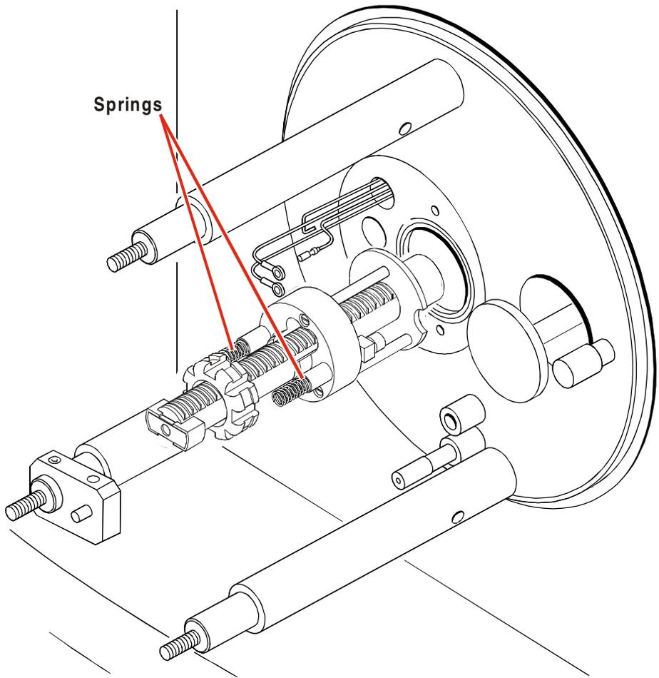
Figure 8-9 Ion Tunnel Assembly Springs
