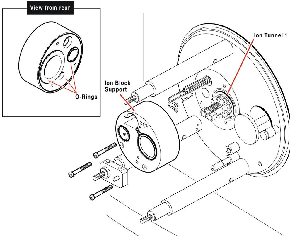
Figure 8-7 Removing and Cleaning Ion Block Assembly
