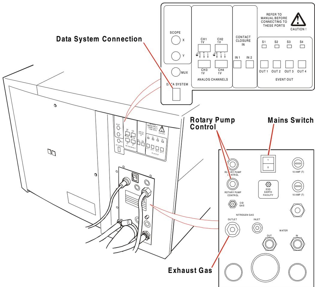
Figure 2-3 Rear Exhaust and Peripheral Connections
