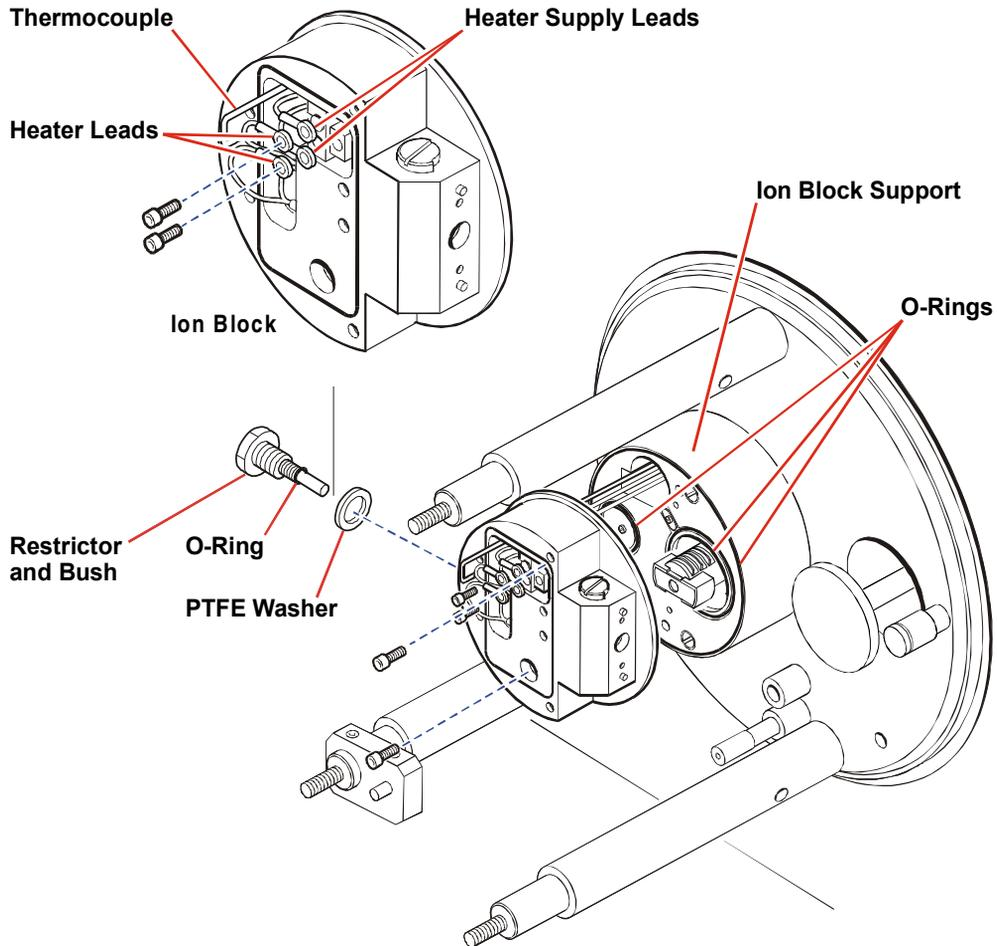
Figure 8-6 Ion Block Removal
