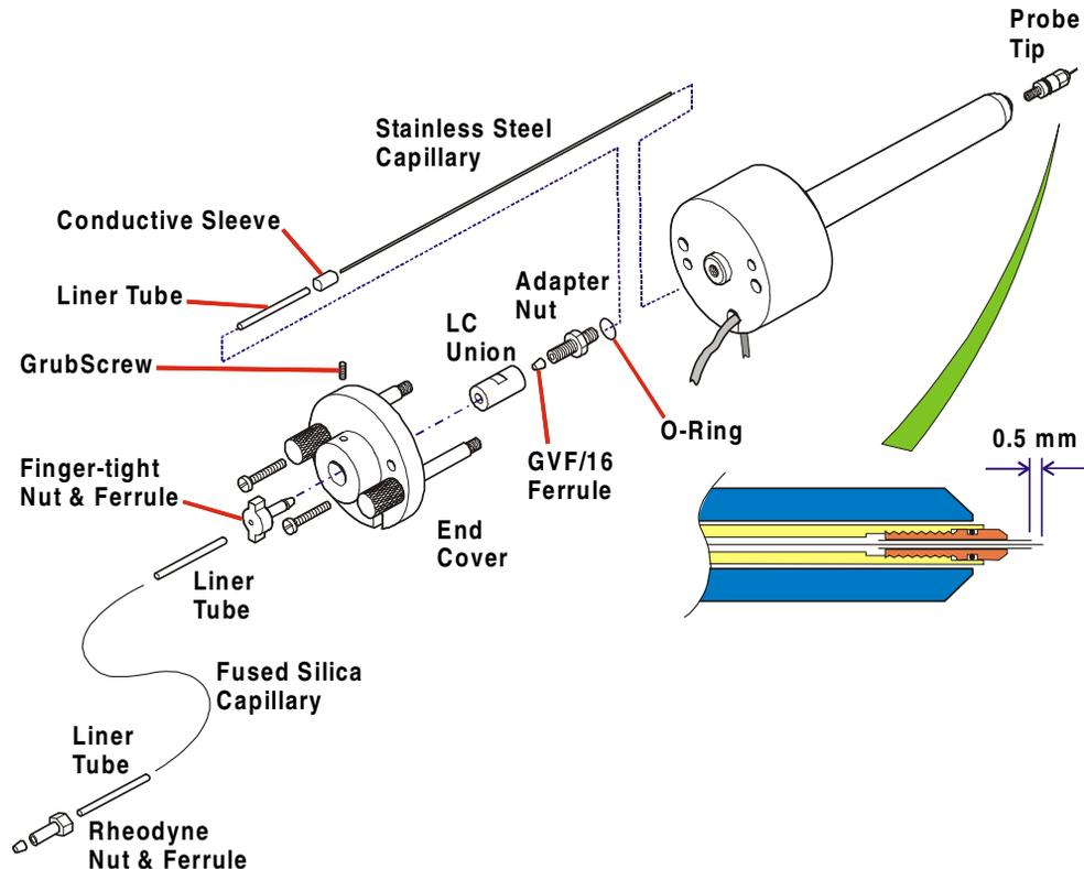
Figure 8-10 Renewal of Stainless Steel Sample Capillary
