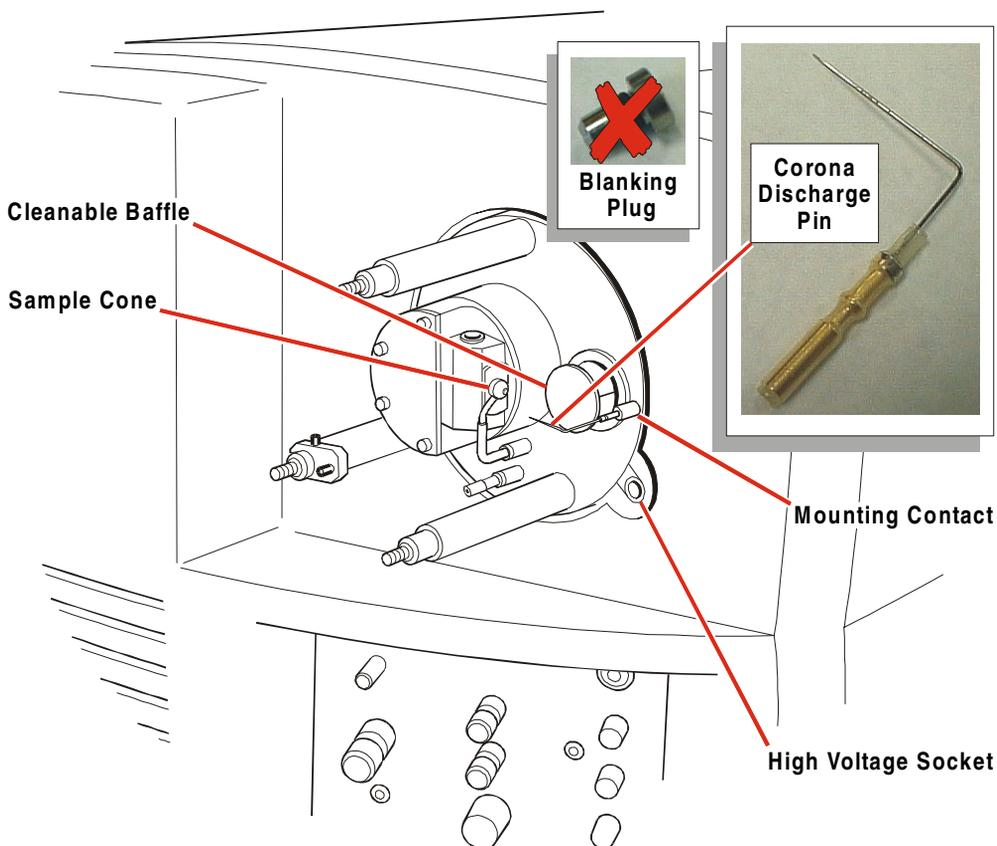
Figure 2-8 Inserting Corona Discharge Pin for APCI
