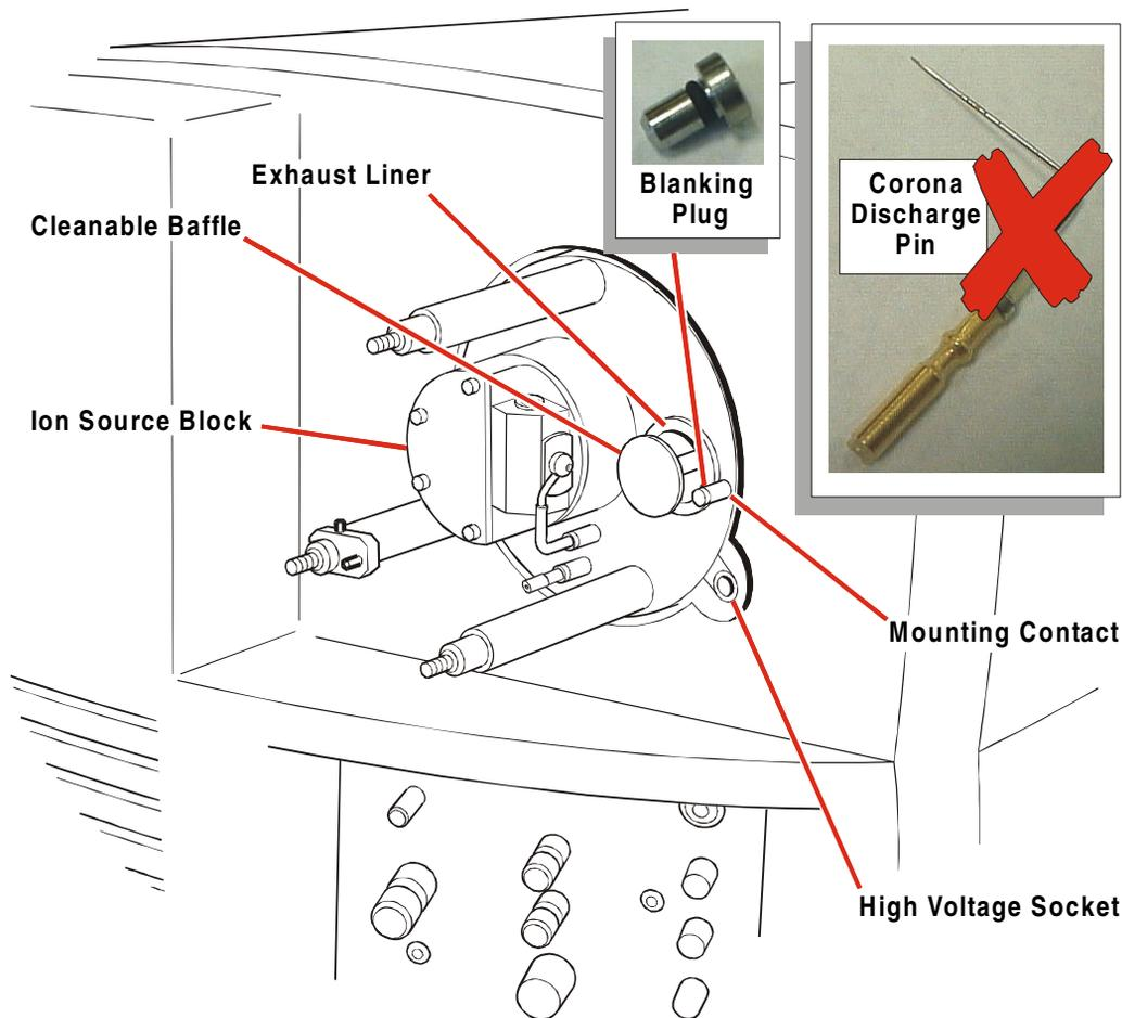
Figure 6-4 Source Setup for Electrospray
