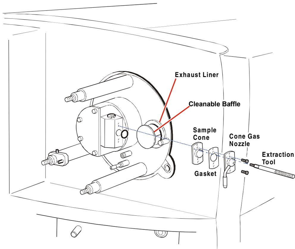
Figure 8-4 Sample Cone Removal
