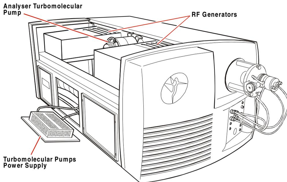
Figure 1-16 Main Electronics Modules
