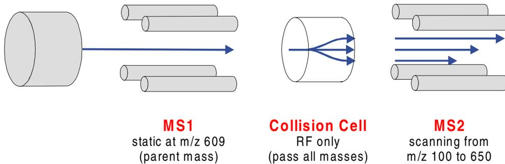
Figure 1-3 MS-MS Mode - Obtaining a Daughter Ion Spectrum
