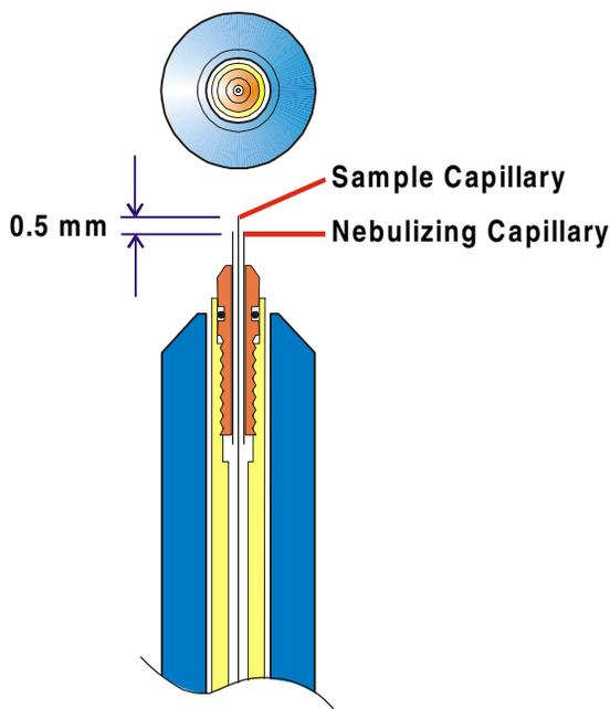
Figure 6-5 Probe Tip Capillary Fine Adjustment
