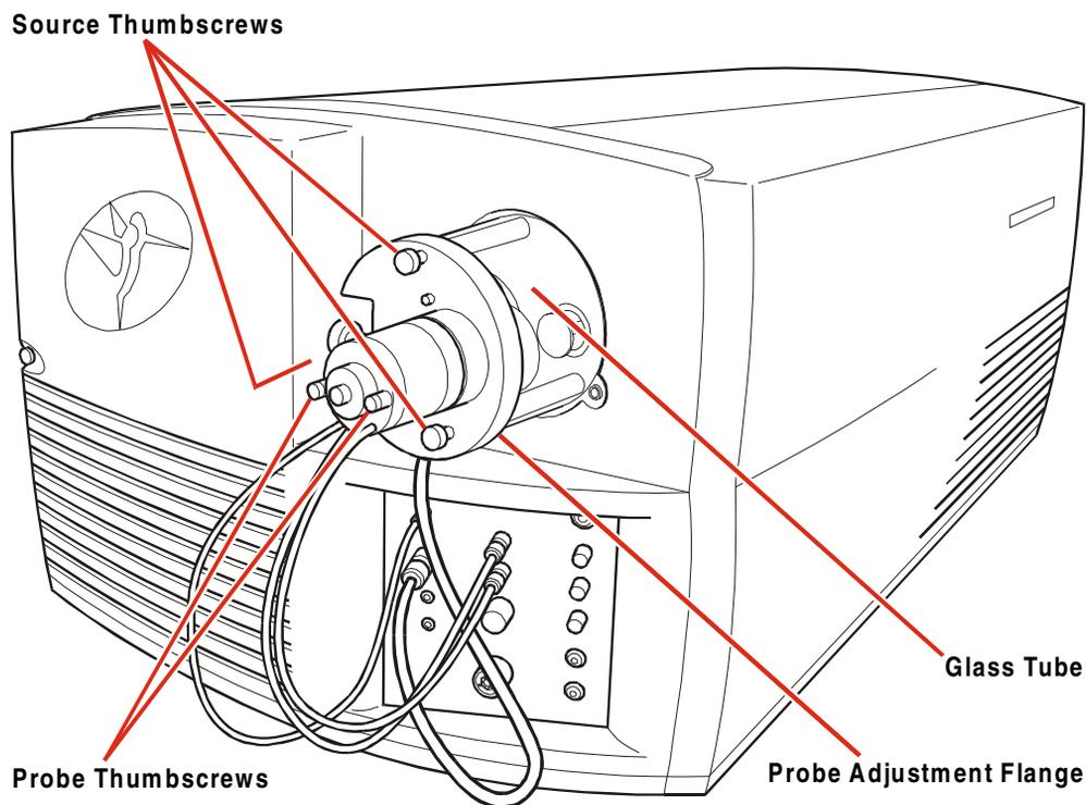
Figure 8-2 Source Dismantling for Sample Cone Access
