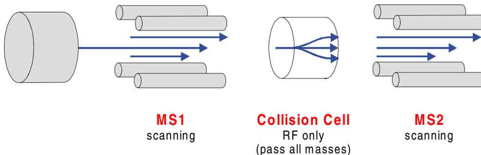
Figure 1-9 Constant Neutral Loss Spectrum
