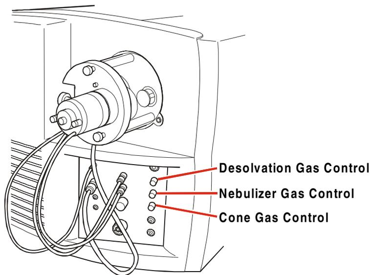
Figure 6-8 Gas Flow Controls
