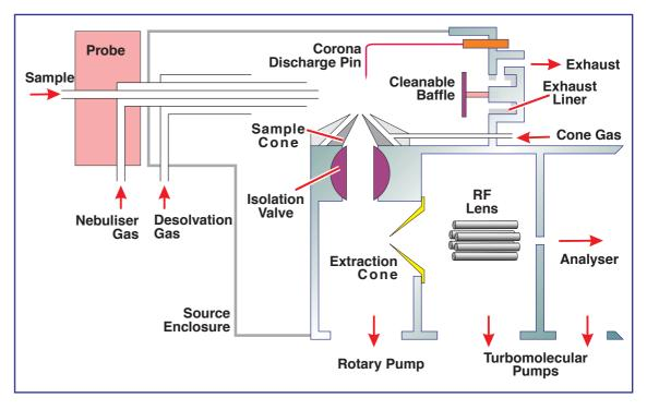
Atmospheric Pressure Chemical Ionisation (APcI) is an easy to use LC-MS interface that produces singly-charged protonated or deprotonated molecules for a broad range of involatile analytes.
