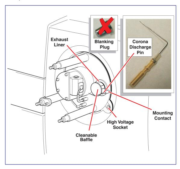
APcI may be operated with or without the cleanable baffle fitted.
