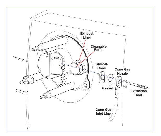
Dry the cone and nozzle using nitrogen.
