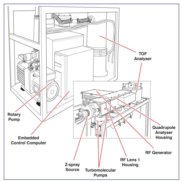
The main internal mechanical components of the instrument are:
