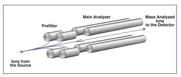
The need to clean the prefilter rods is usually indicated by poor peak shape or loss of resolution (in tuning mode), although other more likely causes, such as contamination of the source should be eliminated first.
