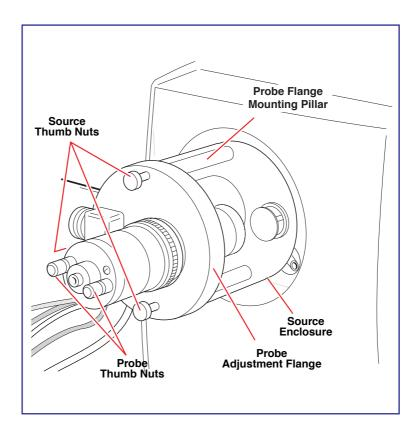
Unscrew the three probe flange mounting pillars, using the holes to obtain the necessary leverage.
