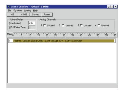
In this example MS1 would begin at m/z300 and step in 1Da intervals up to m/z1000. The spectrum integration time for each step would be 0.9 sec and each step would take 1.0 sec (i.e. 0.9 sec + 0.1 sec). 700 steps at 1 sec/step = 11.66 minutes so the retention time is set to 11.7 min to terminate acquisition at the end of the cycle. (If the retention time is set to a longer period, the cycle will begin again at m/z300 and continue until the retention time is reached.)
