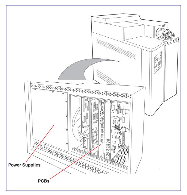
The following electronics modules are located adjacent to the TOF analyser housing:
