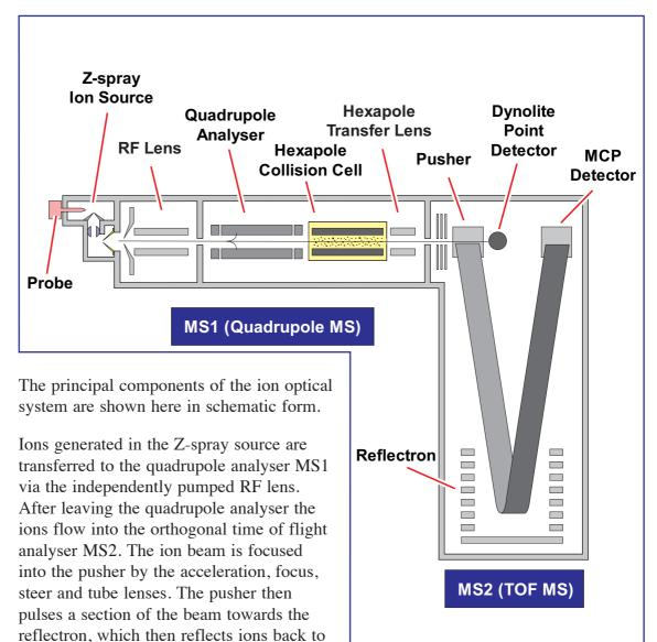
As ions travel from the pusher to the detector they are separated in mass according to their flight times, with ions of the highest mass to charge ratio (m/z) arriving later.
