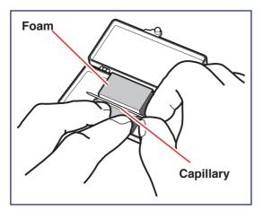
Carefully remove the capillary from its case by lifting vertically while pressing down on the foam with two fingers.
