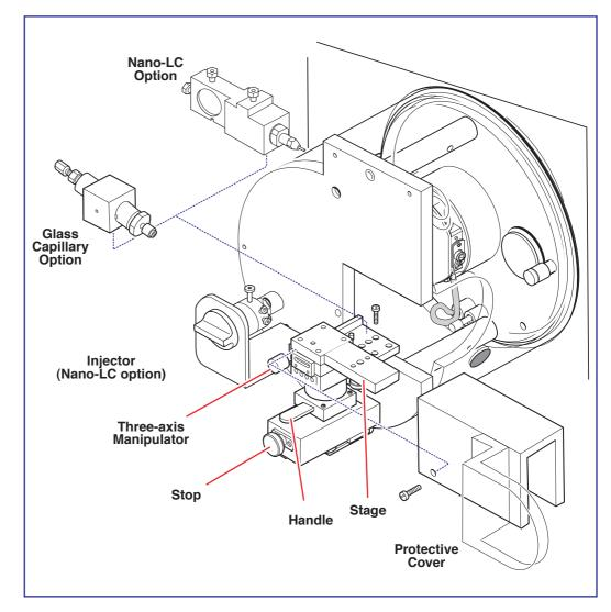
The optional nanoflow interface allows electrospray ionisation to be performed in the flow rate range 5 to 1000 nanolitres per minute. There are two options for the spraying capillary, which can be alternately fitted to the interface:
