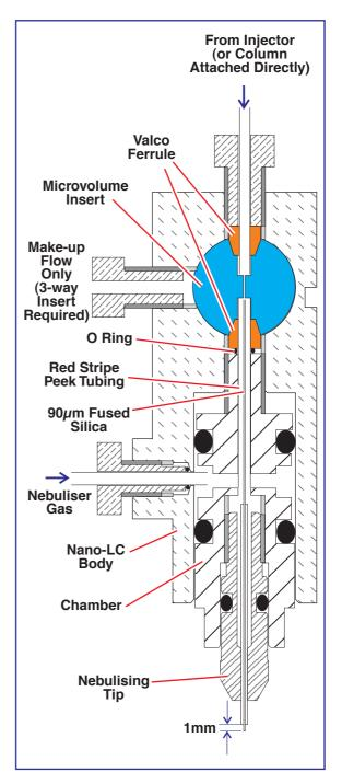
The O ring is required to seal the region between the ferrule and the end of the thread on the nano-LC chamber.
