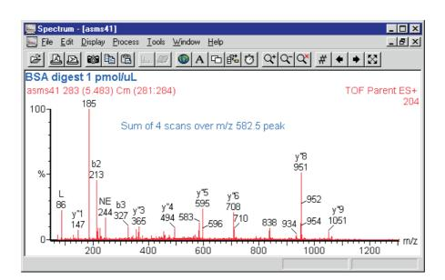
At low levels where precursor scanning of this type would be most valuable, data of this quality is unlikely to be produced with only a few seconds acquisition time for a precursor ion and a product spectrum would need to be acquired for longer with a separate experiment.
