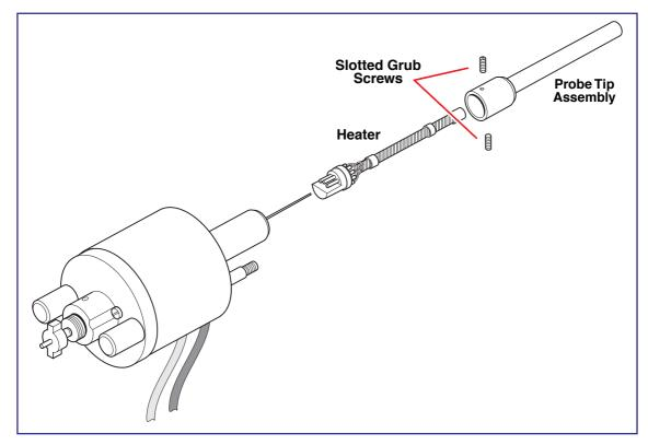
Remove the probe tip assembly by carefully loosening the two grub screws.
