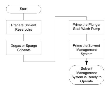
Figure 3-12 Preparing the Solvent Management System for Operation
