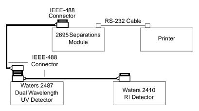
Figure 1-5 Digital Signal Control of an HPLC System
