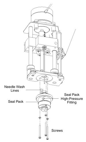
Figure 7-14 Removing the Seal Pack
