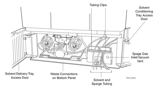
Figure 2-5 Fluidic Connections in the Separations Module
