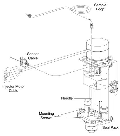
Figure 7-13 Removing the Injector
