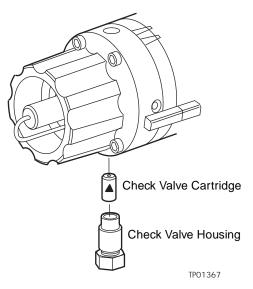
Figure 7-6 Inlet Check Valve
