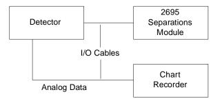
Figure 1-6 I/O Signal Control of an HPLC System
