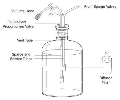
Figure 2-6 Installing Sparge Lines in a Solvent Reservoir
