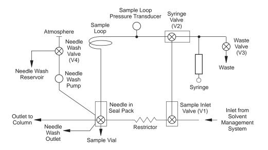
Figure 1-3 Fluidic Path Through the Sample Management System
