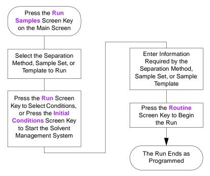
Figure 5-2 Making an Automatic Run in Stand-Alone Mode
