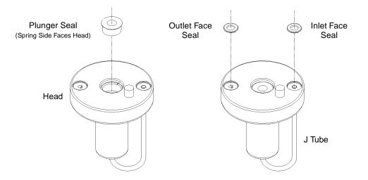
Figure 7-3 Plunger and Face Seal Orientation
