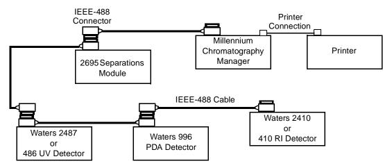
Figure 1-7 Typical 2695 Separations Module HPLC System Under Millennium Chromatography Manager Control
