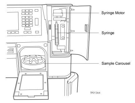
Figure 7-8 Sample Management System Components (Front View)
