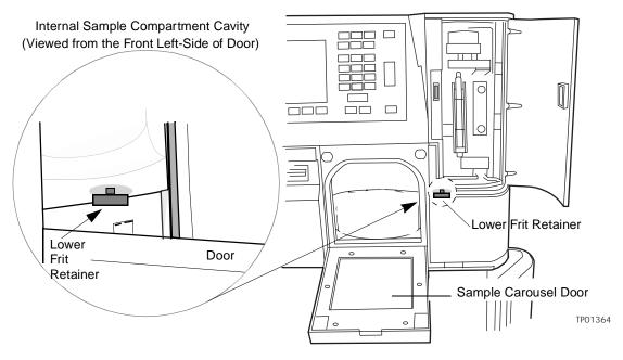
Figure 7-10 Locating the Lower Frit Retainer
