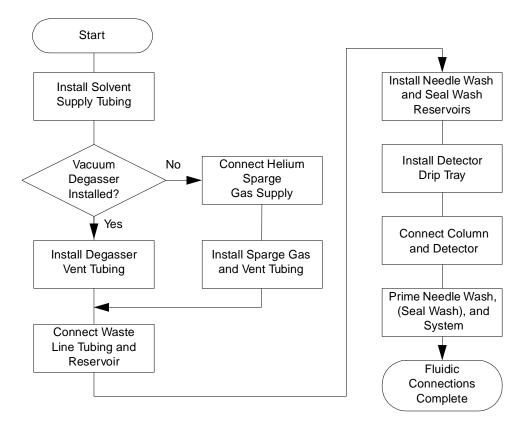
Figure 2-4 Steps to Making Fluidic Connections
