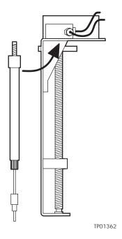
Figure 7-12 Installing the Syringe
