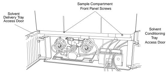
Figure 7-17 Accessing the Sample Compartment
