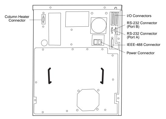
Figure 2-3 Rear Panel of the 2695 Separations Module
