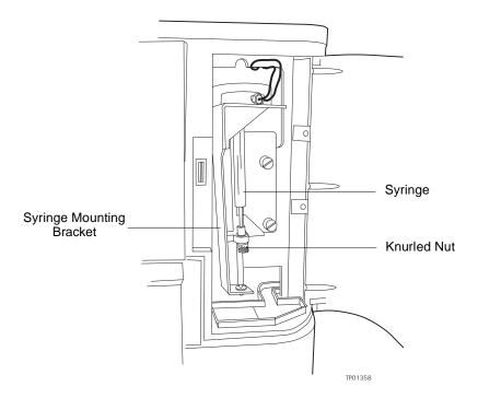
Figure 7-11 Syringe Assembly Components
