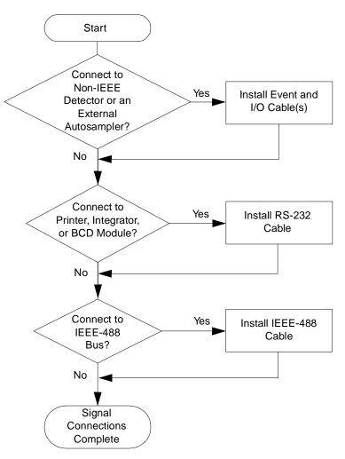
Figure 2-11 Step to Making Signal Connections
