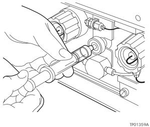
Figure 4-8 Prime/Vent Valve with Syringe
