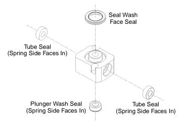
Figure 7-4 Seal-Wash Assembly Seals
