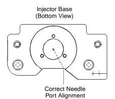
Figure 7-16 Aligning the Needle Port
