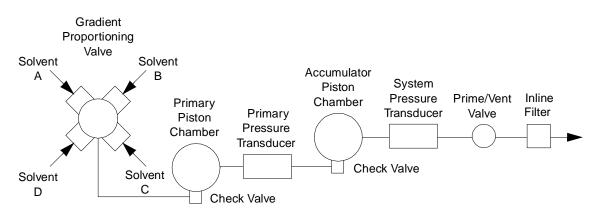
Figure 1-2 Fluidic Path Through the Solvent Management System
