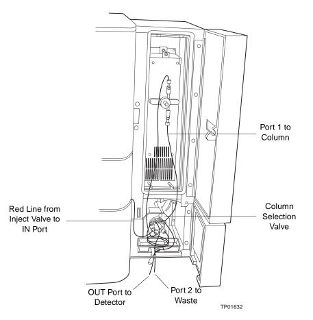
Figure 1-8 2695 Column Heater with 3-Column Selection Valve Installed
