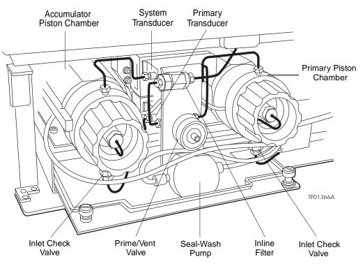
Figure 7-1 Solvent Management System Components
