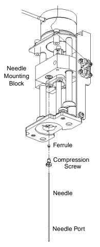
Figure 7-15 Replacing the Needle
