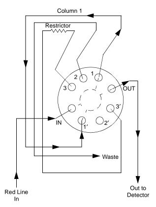
Figure 2-8 Three-Column Selection Valve Configuration (As Shipped)
