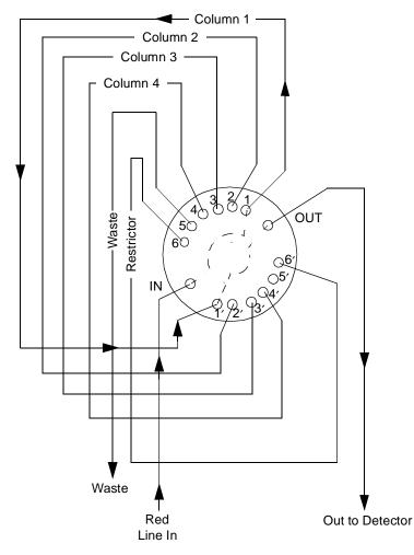
Figure 2-9 Six-Column Selection Valve Connections (Example)
