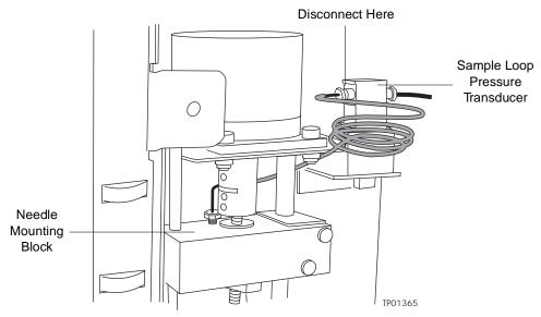
Figure 2-13 Disconnecting the Sample Loop
