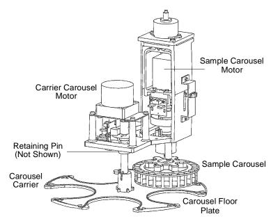
Figure 7-18 Sample Compartment Components
