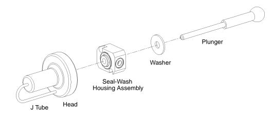
Figure 7-5 Plunger, Seal-Wash, and Head
