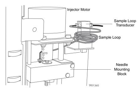
Figure 7-9 Sample Management System Components (Right-Side View)
