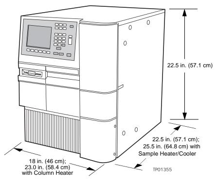
Figure 2-2 Typical System Dimensions
