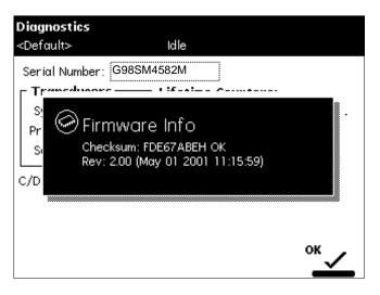
Figure 8-25 Displaying the Firmware Checksum
