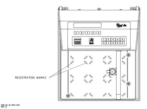
Figure 2-7 Registration Marks on Drip Pan
