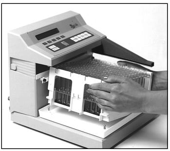
Figure 2-4 Installing the Test Tube Rack
