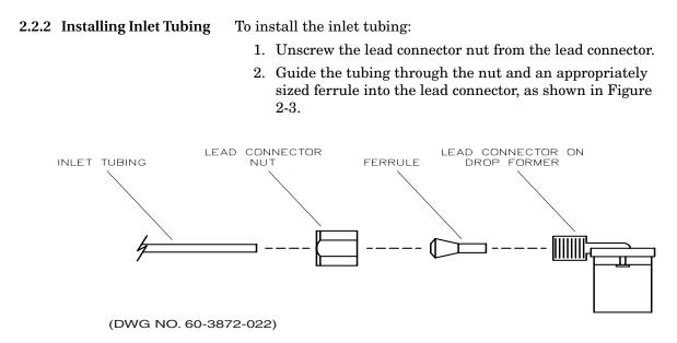
Figure 2-3 Installing the Inlet Tubing
