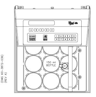
Figure 2-8 150 ml Bottles Positioned on Drip Pan
