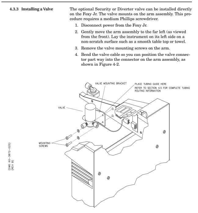
Figure 4-2 Installing the Valve on the Arm Assembly
