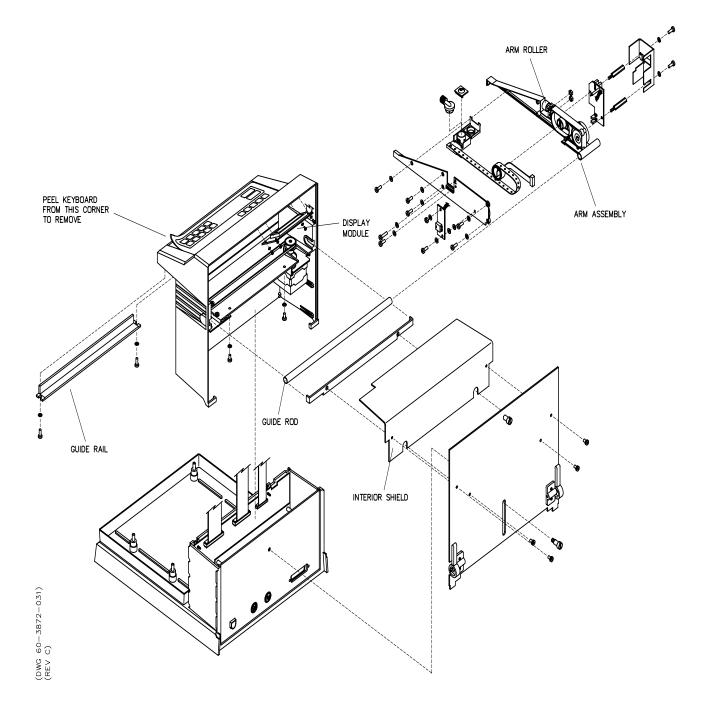
Figure 7-5 Foxy Jr. Exploded View
