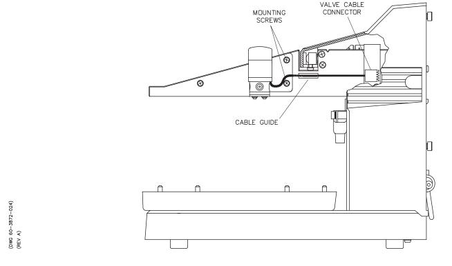
Figure 4-3 Attaching the Valve Cable
