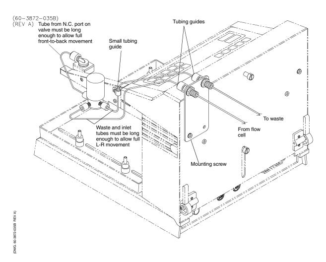
Figure 4-6 Routing Tubing with Accessory Valve
