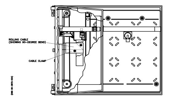
Figure 7-13 Rolling the Cable and Clamp, Top View
