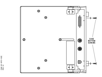
Figure 7-3 Removing the Case Bottom Screws
