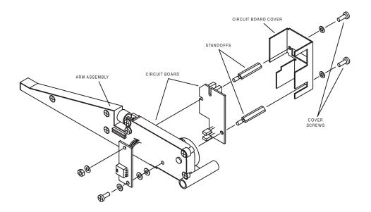
Figure 7-8 Removing the Arm Circuit Board Hardware
