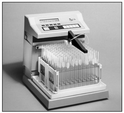
Figure 1-1 Foxy Jr. Fraction Collector
