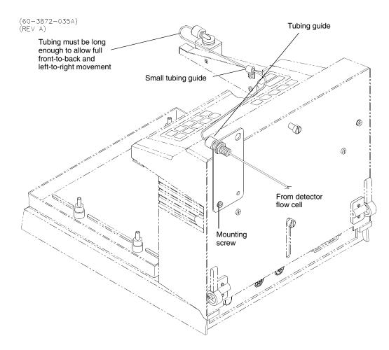
Figure 4-5 Small Diameter Tubing Routing
