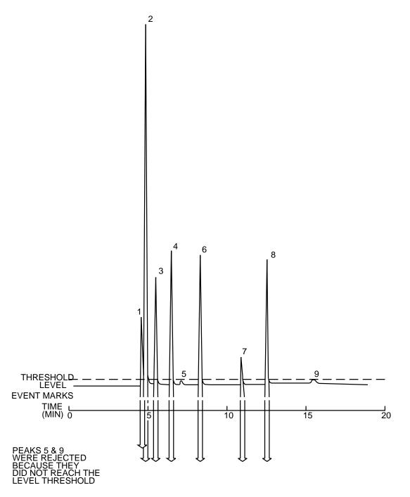
Figure 3-6 Slope and Level Sensing Collection
