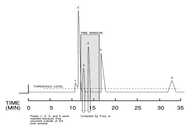
Figure 3-8 Time Windows/Level Sensing
