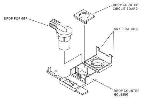
Figure 7-9 Replacing the Drop Counter Circuit Board
