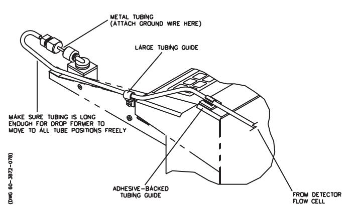
Figure 4-7 Routing Large Diameter Tubing
