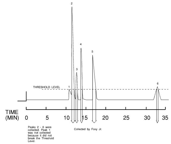
Figure 3-4 Level Sensing Collection
