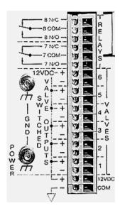
Figure 4-13 Rear Panel Showing Location of +12 VDC and Unswitched Com Source
