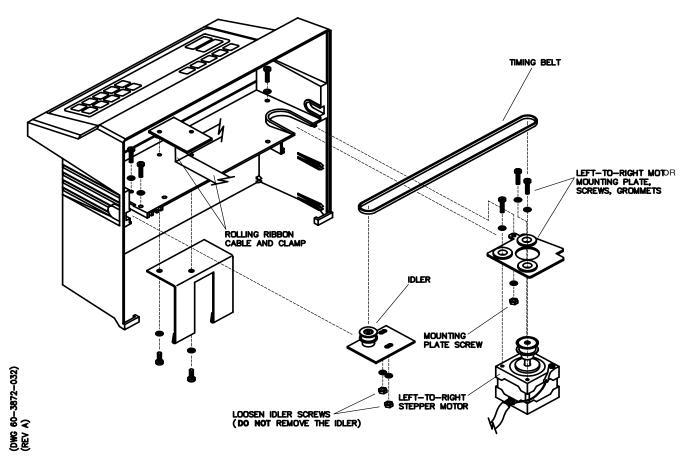
Figure 7-6 Removing the Timing Belt (exploded view)
