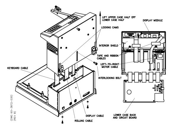
Figure 7-4 Cable Locations on Circuit Boards, Case Disassembly
