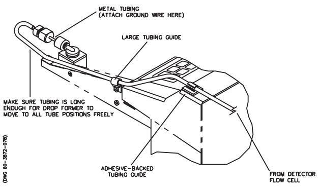
Figure 2-6 Connecting Grounded Metal Tubing to the Drop Former
