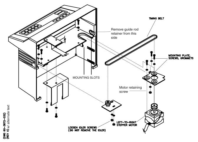
Figure 7-7 Replacing the L-R Motor
