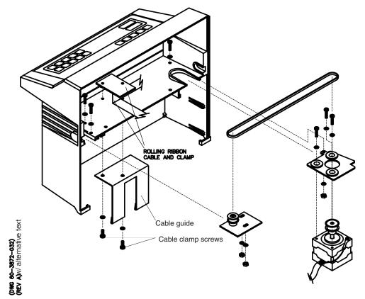
Figure 7-12 Rolling the Cable Mounting Hardware
