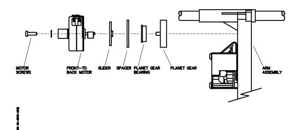
Figure 7-10 Front-to-back Drive Assembly
