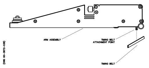
Figure 7-11 Removing the Timing Belt from Arm
