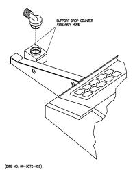
Figure 2-2 Removing the Drop Former
