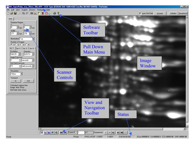
**NOTE**: The Software toolbar is a flexible dockable/undockable toolbar. It can be picked up and moved left, right, top or bottom, docked or left floating for your convenience. The Scan and Camera control tabs and View & navigation toolbar are also left or right dockable or can be floating.
