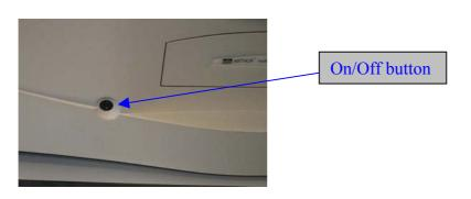
WARNING: when the instrument is started up the transport carrier comes out automatically. Make sure you leave space for this in front of the instrument.
