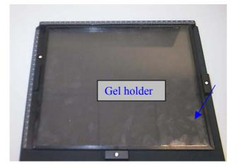
The adapter plate fits on the carrier frame on which there are three studs to locate the adapter plate.
