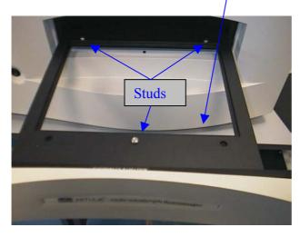
On the back of the adapter plate are three recesses which fit over the studs. It is easiest to load the adapter plate at an angle so that you can see under it to locate the rear studs and then lower it to locate the third stud at the front.
