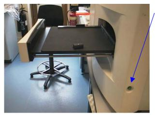
Press the green button on the side of the instrument to drive the transport carrier into the instrument. Note that you have to hold the button down all the time until the carrier is in fully in the instrument.
