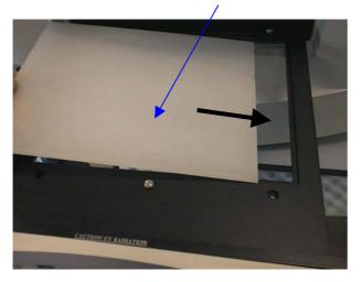
For flat-field correction you can use this as it is. For sample imaging, use the open sample carrier plate shown on the previous page. Place it on the transport carrier. Make sure it is located on the three studs.
