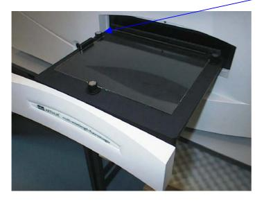
You can check the correct height by eye. The centre of the sample should be in line with the slit at the back of the sample carrier plate. This slit is exactly 9mm above the plate.
