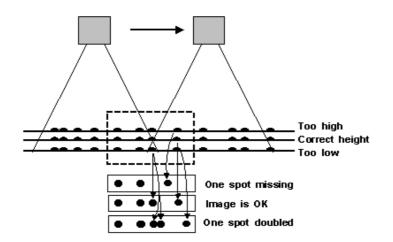
The camera moves a predefined distance, which is defined by the pixel sizes in the 'scanner.ini' file. If the sample is positioned too high up there will be a gap between each frame and parts of the image will be missed. If the sample is too low there will be an overlap between frames and part of the sample will be imaged twice.
