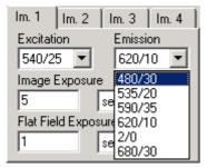
Note: a value of 0/0 means the position is empty, and /0 represents a long-pass filter i.e. 485/0 is a long-pass filter).
