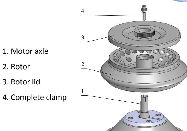
Fig.3. Assembly of angle rotor
