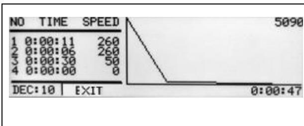
New section programming possible (the whole line 4 is blinking). Programming as in the case of the section 1. If speed of the last section=0, it is possible to save the created characteristics by choosing the **EXIT** option with **▲▼** keys and pressing the **SET** key and then choose **EXIT** and press **SET**.
