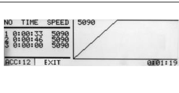
Programming of new section possible (the whole line 3 is blinking). Programming as in the case of section 1. It is possible also to abandon the programming: with **▲▼** keys choose the **EXIT** option (it will blink) and save (press the **SET**) only the acceleration characteristics of 2 section with **TIME/SPEED** parameters described in the line 1 and 2.
