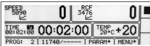
Icon signals that program with user acceleration/deceleration characteristics are loaded.
