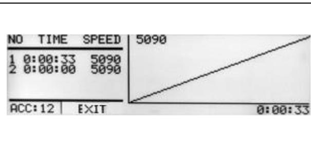
Programming of new section possible (the whole line 2 is blinking). Programming as in the case of section 1. It is possible also to abandon the programming: with UP/DOWN keys choose the **EXIT** option (it will blink) and save (press the **SET**) only the acceleration characteristics of 1 section with **TIME/SPEED** parameters described in the line 1.
