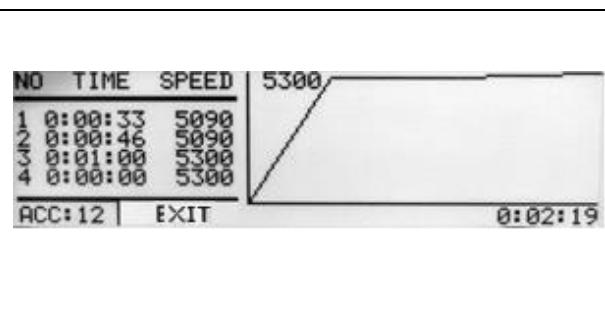
Programming of new section possible (the whole line 4 is blinking). Programming as in the case of section 1. It is possible also to abandon the programming: with **▲▼** keys choose the **EXIT** option (it will blink) and save (press the **SET**) only the acceleration characteristics of 3 section with **TIME/SPEED** parameters described in the line 1, 2 and 3.
