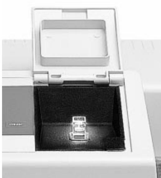
**Figure 1.5: Cuvette Chamber**
