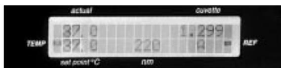
The left side of the display shows the temperature, both actual and set point, and whether or not the temperature is at the set point (enunciator blinks if not at set point). The middle of the display shows the wavelength. The right side of the display shows the data received from the reading as either absorbance or percent transmission and indicates whether or not a reference measurement was made (enunciator blinks if no reference reading was taken).
