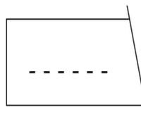
Zeroing of the display (taring) is automatic. While the zeroing is in progress and the horizontal segments appear in the display, you can abort the process by briefly pressing the «Re-Zero» key again.
