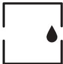
If you wish to employ fine dispensing (weighing in) of a fine powder or small amounts of liquid, select the **weighing in** position. This provides a continuous display of all decimal places, and the weight increase can thus be followed easily.
