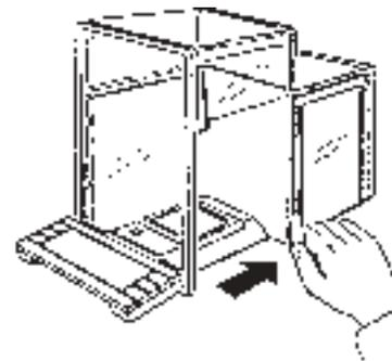
**For loading the balance, open only as many doors as necessary. With relatively small weighing samples or rather small tare containers, it is normally sufficient to open a single door. This lessens the influence of drafts and speeds up the weighing process.**
