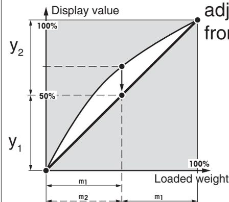
In this mode you can also initiate the fully automatic adjustment and linearization at any time with a keystroke. This is practical, for instance, when your AT reports during a weighing that it wishes to adjust itself. Section 5.4 shows you how to proceed in such a case.
