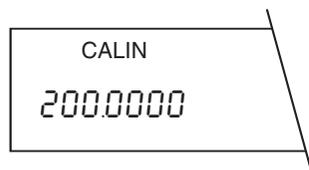
After a short time, the audio warning beep sounds and the requested, model-dependent adjustment weight appears in the display, for example, 200 g.
