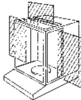
The fixed bars of a traditional draft shield prevent access to the weighing chamber.
