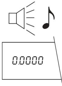
As soon as the warning beep sounds, zeroing of the balance is complete and the fully automatic door function opens the draft shield.
