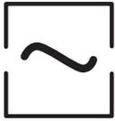
This setting is suitable for **normal ambient conditions**; the balance operates at **moderate speed** in this case. This position is set in the factory.
