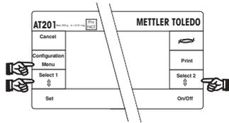
By pressing and holding the «**Configuration**» key, you call up the configuration register. You select the different
