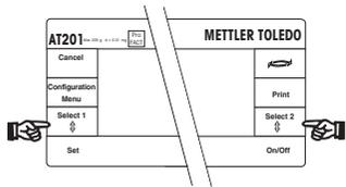
The **semiautomatic** operation can be effected either with the left or the right  $\updownarrow$  key. In this case, the draft shield is opened and closed by the motor.
