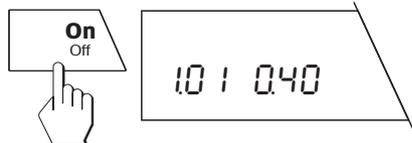
Press the «**On/Off**» key. The display shows the installed software version briefly and the normal weight display then appears.
