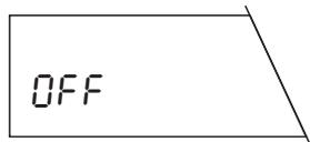
The balance now performs a self-test in which all display segments light up. "OFF" then appears in the display ("OFF" shows that the balance was disconnected from the power supply).
