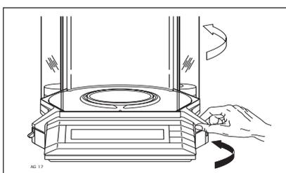
If you wish to open and close both draft shield doors individually, push **both coupling elements to the bottom position**. Owing to the space requirements for insertion of the doors, only one of the doors can be opened fully at any one time.
