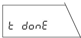
The balance confirms that the test has been performed.
