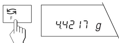
You can use the «F» key at any time to switch the display between the percent display, weighing unit 1 and weighing unit 2.
