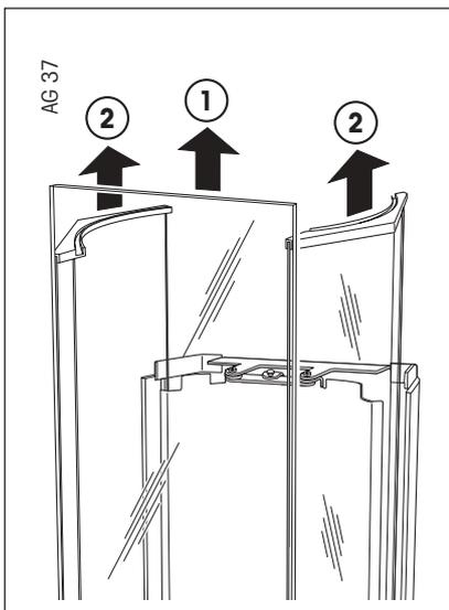
Remove the front door (1) and then lift the two side weighing chamber doors (2) out of their guide. Important: The two side doors can be removed only if they are in the very front ("closed") position!
