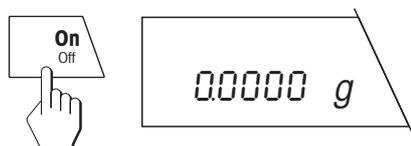
To **switch on the balance**, press the «**On/Off**» key **briefly**. As soon as the normal weight display appears, your balance is ready for weighing.
