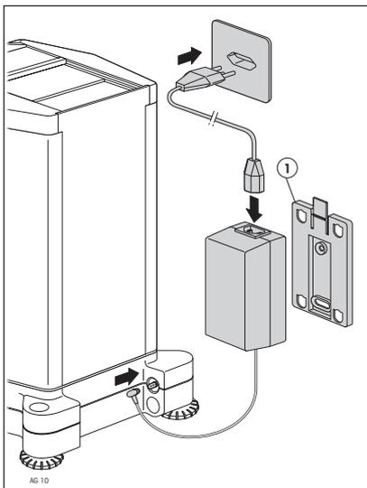
Should you wish to use the holder (1) supplied for the AC adapter: Attach the holder to a suitable, sufficiently stable area using two screws (e.g. to the wall or the underside of a bench top). Press the AC adapter in the holder.
