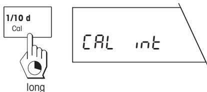
Start the adjustment operation by pressing and holding the «Cal» key. The balance briefly shows that adjustment (calibration) is being performed with the internal weight.
