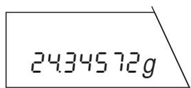
If you remove or decrease the weight following a weighing in the range above 31 or 81 grams, the balance automatically returns to the fine range.
