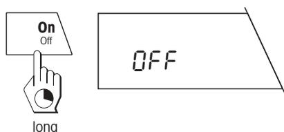
To **switch off the balance**, press and **hold** the «**On/Off**» key until the message “OFF” appears in the display.
