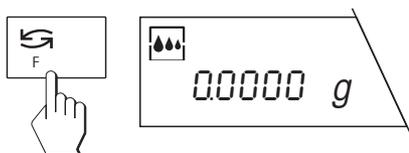
Briefly press the " $\rightarrow \text{F} \leftarrow$ " key. The symbol of the weighing process adapter in the display confirms that dynamic weighing has been activated.
