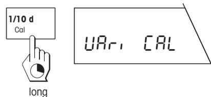
Start the calibration operation by pressing and holding the «**Cal**» key. The balance shows briefly that an external weight is being used for calibration.
