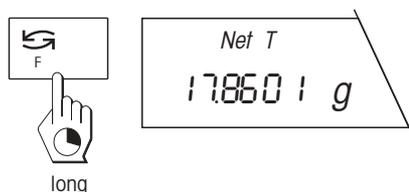
Now add the component to the container until the desired net total weight is reached.
