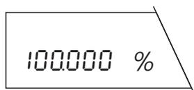
On completion of the weighing-in operation, your balance is ready for percent weighing.
