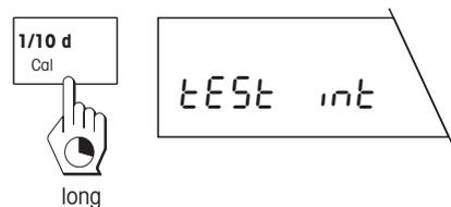
Initiate the test procedure by pressing and holding the «**Cal**» key. The balance briefly confirms that the test will be carried out with the internal weight.
