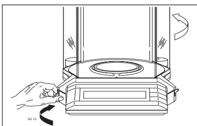
If you operate the draft shield with one hand and wish to load the balance using the other, push **one coupling element downward and the other upward**.
