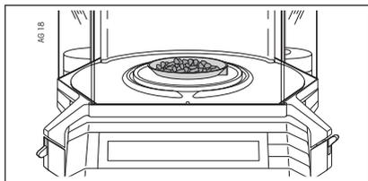
After you have performed taring, open the draft shield, place the weighing sample on the pan and close the draft shield.
