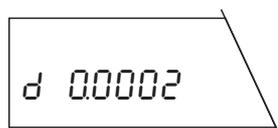
The balance now shows the difference (deviation) between the calibration and the current test weighing for 10 seconds.
