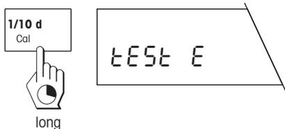
Initiate the test procedure by pressing and holding the «Cal» key. The balance briefly confirms that the test will be carried out with an external weight.
