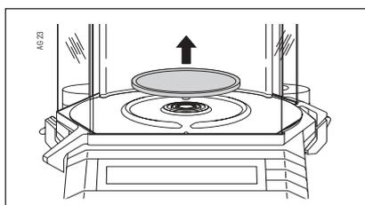
Open the draft shield and remove the weighing pan (with the AG135, AG285 also the draft shield element).
