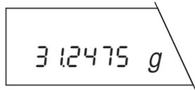
If the weight is greater than 31 or 81 grams, the balance quits the fine range and displays in the normal weighing range.
