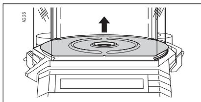
Remove the weighing chamber plate.
