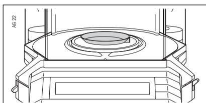
If you work with a weighing container, place it on the weighing pan in the normal weighing mode.
