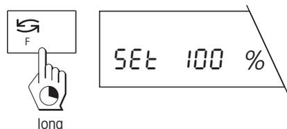
Your balance needs a reference weight corresponding to 100%. Press and hold the «F» key until you are prompted to load the reference weight.
