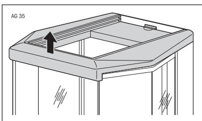
Carefully lift up the weighing chamber cover and remove.
