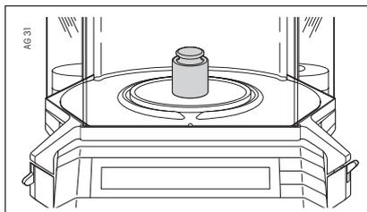
Place the requested weight in the middle of the weighing pan.
