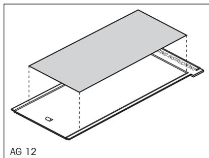
Carefully remove the sticker with the short-form operating instructions from its backing film and stick the short-form operating instructions to the slide.
