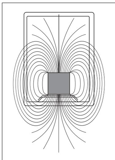
The magnetism of a weighing sample can lead to the weighing result being dependent on the position of the weighing sample on the weighing pan and to a result that is difficult to reproduce. Magnetic forces are interpreted wrongly by the balance as an additional load.
