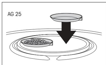
Place the additional weighing container on the weighing pan next to the weighing containers already tared.
