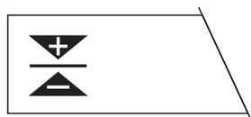
For rapid determination of the preset value (100%), a visual weighing-in aid appears in the display. When the target weight is within  $\pm 2.5\%$ , both arrows are visible. This tolerance setting is fixed and can be changed only via the interface.
