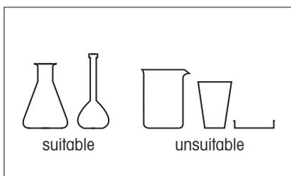
Always use the smallest possible weighing container as the error tends to increase with increasing container size. Further, you should use weighing containers with as narrow a neck as possible and a cover.
