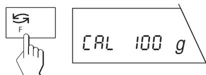
If you do not wish to calibrate with the suggested weight, you can select a different weight\* by briefly pressing the «**F**» key. The available weights depend on the balance model.
