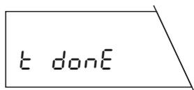
The balance confirms that the test has been performed and then returns automatically to the weighing mode.
