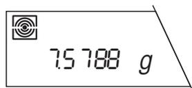
Briefly press the « $\rightarrow$ » key. As soon as the weighing result is stable, the status indicator of the repeatability fades and the result is transferred to the attached device.
