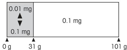
If you have an AG135 or AG285 balance, you have a dual-range balance. These models also have a fine (semimicro) range from 0 to 31 or 81 grams, respectively. In this fine range the balance shows the result with a higher resolution, i.e. with one decimal place more. In contrast to the DeltaRange® balances, this fine range can not be moved, i.e. it always starts at 0 and ends always at 31 or 81 grams.
