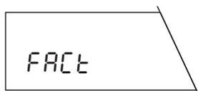
This is the factory setting. The balance adjusts (calibrates) itself fully automatically. With certified versions of the balances, this function is always active even if a different setting has been preselected in the menu; FACT does thus not appear at all here.
