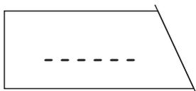
Taring runs automatically. If you tare the balance when it is unstable, the taring operation will be shown in the display by horizontal segments.
