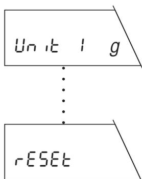
The next menu option appears in the display. Each time the «**Menu**» key is pressed, the balance switches to the following menu option.
