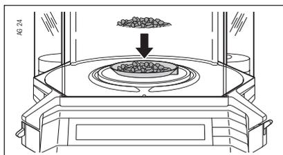
Briefly press the «G» key and the desired weight is confirmed as an additional component.
