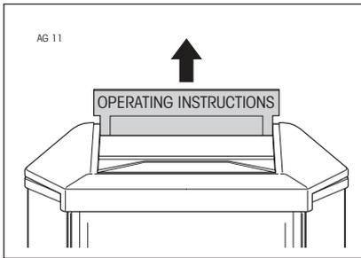
Remove the slide with the short-form operating instructions. Then carefully pull off the panes of the top weighing chamber door backwards from the balance. Hold the bottom pane firmly to avoid dropping it.
