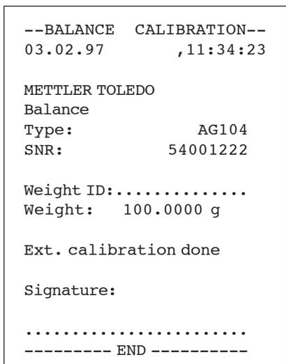
If your balance is connected to a printer, the adjustment (calibration) is recorded automatically in conformance with GLP. The record opposite is a specimen printed out with the METTLER TOLEDO LC-P45 Printer. Records printed with other printers may differ somewhat from the example shown.
