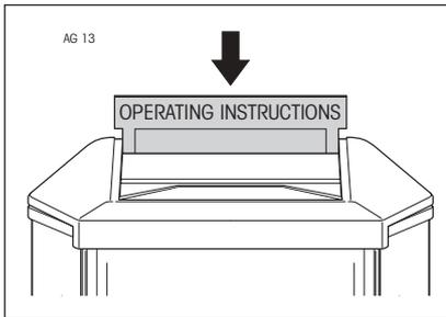
Place the slide in its guide slot on the balance and push it down as far as it will go.
