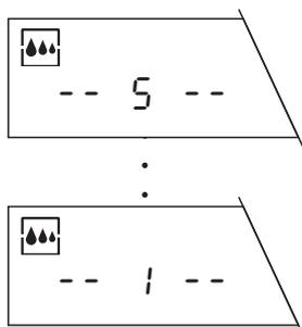
The remaining weighing time (in seconds) is continuously displayed.
