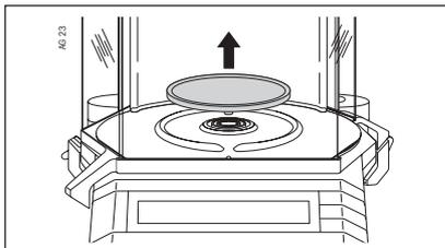
Remove the weighing chamber plate.
