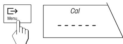
Confirm the selected weight with the «**Menu**» key. This also initiates the calibration procedure. The balance determines the zero point.
