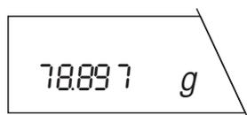
If the fine range is exceeded in the display, the balance display automatically switches to the lower readability.
