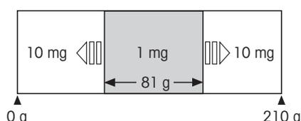
The illustration opposite shows the principle of the movable fine range in which one additional decimal place is displayed (in this example, the movable fine range comprises 81 grams).
