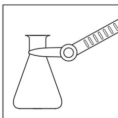
Never hold weighing samples or containers with your hand (approx. 35 °C), but only with tongs or tweezers. Never place your hand in the weighing chamber. This avoids temperature changes which can be caused by body heat.
