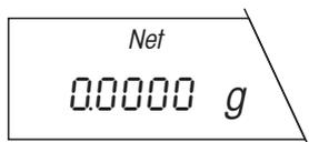
After the first component has been weighed in, the display is reset to zero and the balance is now ready for weighing in of the second component.
