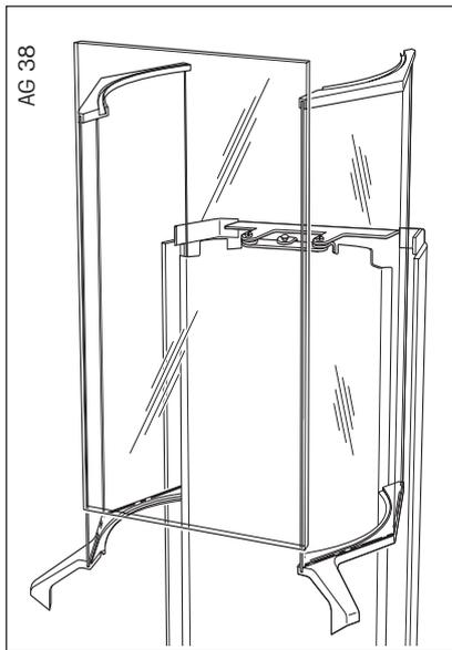
Assemble your balance in reverse order. When inserting the two side weighing chamber doors, ensure that they are correctly positioned in their guide slot. Do not forget to lock the weighing chamber cover!
