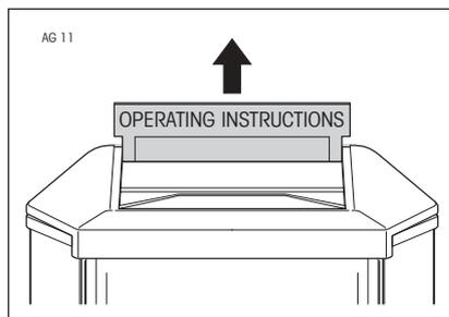
Pull the slide for the short-form operating instructions upward out of the balance (you must overcome a slight resistance which serves as a stop). Place the slide on a flat surface.
