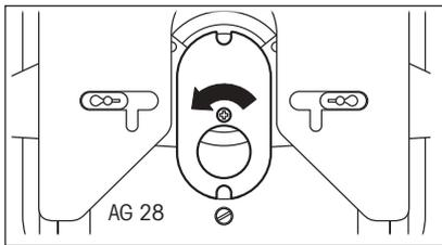
Unscrew the screw of the hanger cover. You need unscrew the screw only until you can turn the cover.
