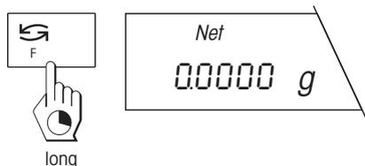
Press and hold the «F» key again until the balance switches back to the weight display. You can now weigh in additional components.
