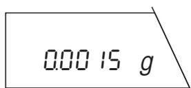
The balance displays the result in **weighing unit 1**.
