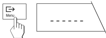
Then press the «Menu» key briefly. While the horizontal dashes are displayed, your balance is calculating the reference weight.
