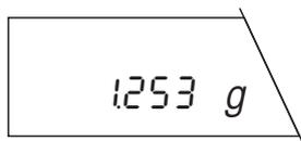
... the balance operates with **lower readability** (one decimal place less), but displays the result considerably **faster**. Press the «**1/10d**» key again to return to normal readability.
