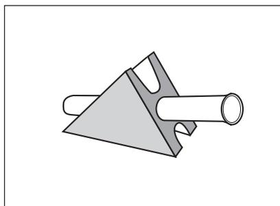
Instead of supports made of the materials mentioned above, use the optional triangular holder. You can order the triangular holder from METTLER TOLDEO with the number 210435.
