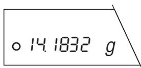
Wait until the circular symbol of the stability detector fades. When the symbol has faded, the weighing result is stable.
