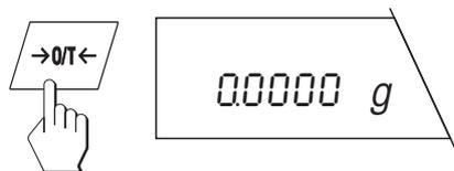
Briefly press the «→0/T←» key. The balance is now tared with the additional weight of the new weighing container. If your balance is connected to a printer, the tare weight of the new container is printed out. You can now weigh in additional components.
