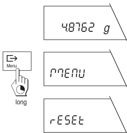
Press and hold the «**Menu**» key until the balance switches to the menu.
