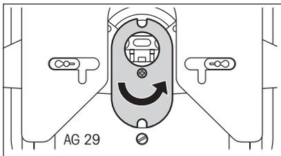
Turn the cover by 180 °C. Center the hole in the cover exactly over the opening in the base of the balance.
