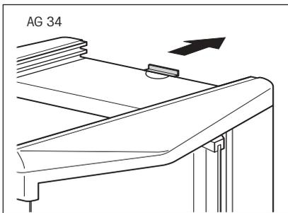
Undo the locking device of the weighing chamber cover.
