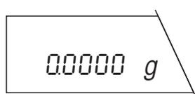
After switching on, DeltaRange® balances operate in the fine range as standard.
