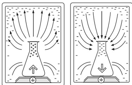
This charging frequently appears in heated rooms with **dry air** (less than around 40% rel. humidity) and with weighing samples made of **glass** or **plastic**. Electrostatic charging generates forces which can disturb the weighing. This leads to constantly changing and unstable display results.
