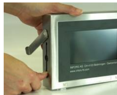
Push the button to release the memory card
