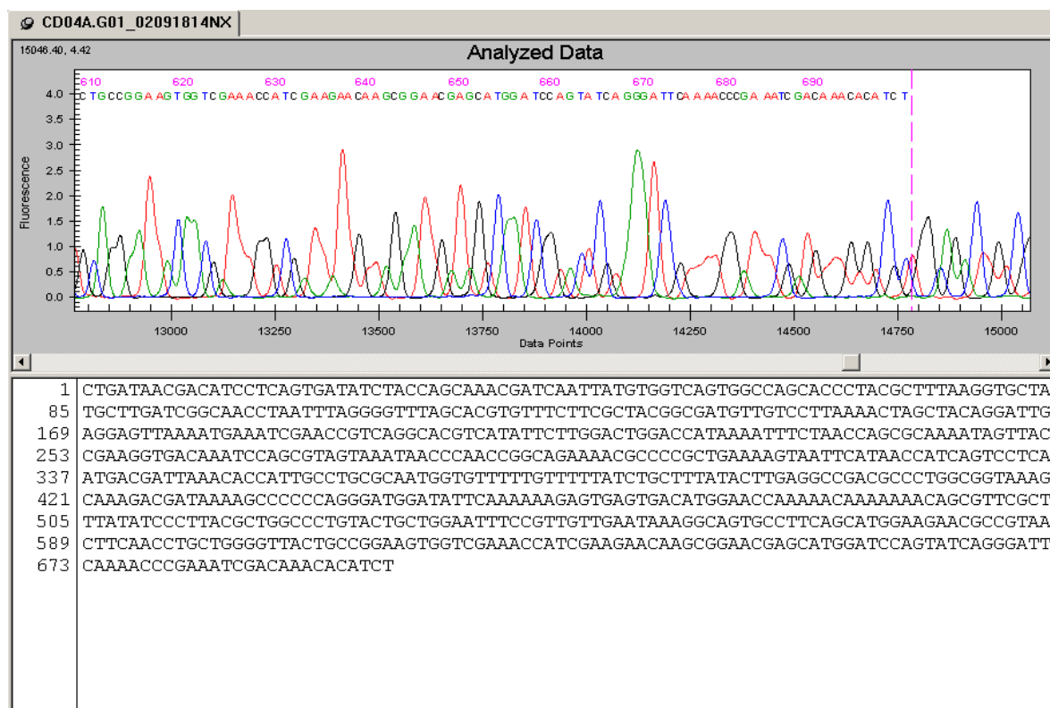
Figure 109: Base Sequence and Trace Views after Sequence-based Trimming – Sequence-based Trimming Applied
