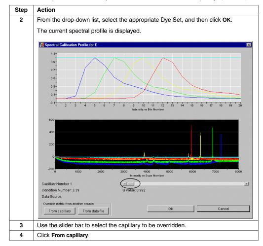
To override a spectral calibration profile with data from another capillary: (continued)
