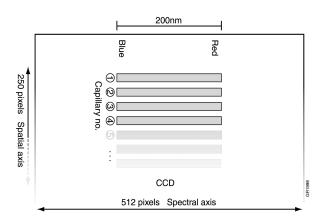
The collected emission spectrum ranges from 500 nm (blue) to 700 nm (red).
