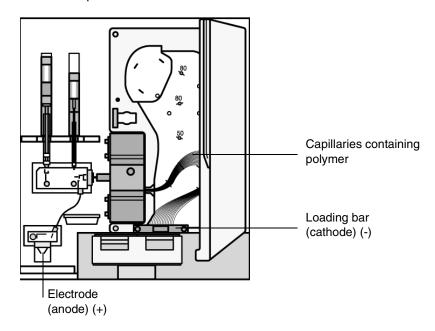
**Description** During electrophoresis, a high voltage is applied between the loading bar (cathode) and the electrode located on the lower polymer block (anode). The voltage drives the movement of negatively charged DNA fragments through the polymer in the capillaries towards the anode. From the anode, the current flows back in electrical wires through the power supply to the cathode to complete the circuit.
