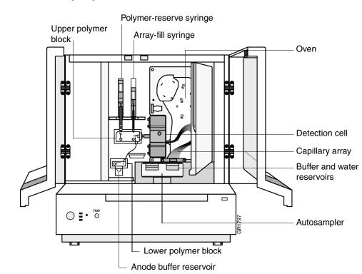
**Diagram** The following diagram shows inside the instrument's doors:
