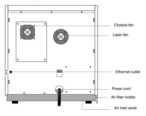
Diagram The following diagram shows the back of the instrument:
