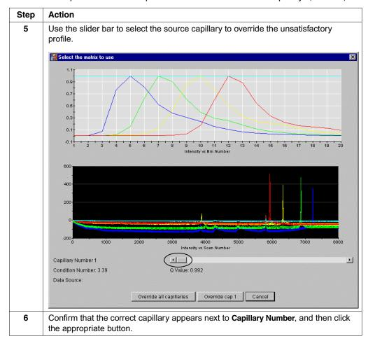
To override a spectral calibration profile with data from another capillary: (continued)
