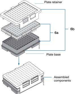
**8.** Verify that the holes of the plate retainer and the septa strip are aligned. If not, re-assemble the plate assembly (see step 7).
