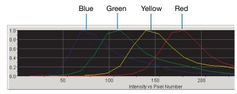
Example of a 4-dye spectral profile
