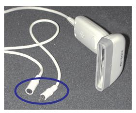
An external barcode reader can be used with the 3130/3130xl instrument. With the KEYENCE BL-80VE (see photo above), which connects to the instrument computer keyboard, you can scan barcodes into any text box in the Data Collection software. The KEYENCE BL-80VE barcode reader uses an LED as a light source.
