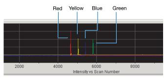
Example of a 4-dye sequencing raw data profile
