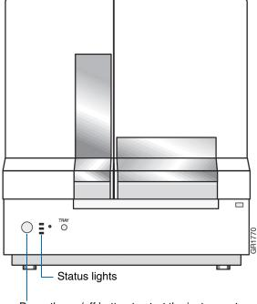
Press the on/off button to start the instrument
