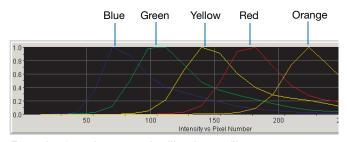
Example of a 5-dye spectral calibration profile
