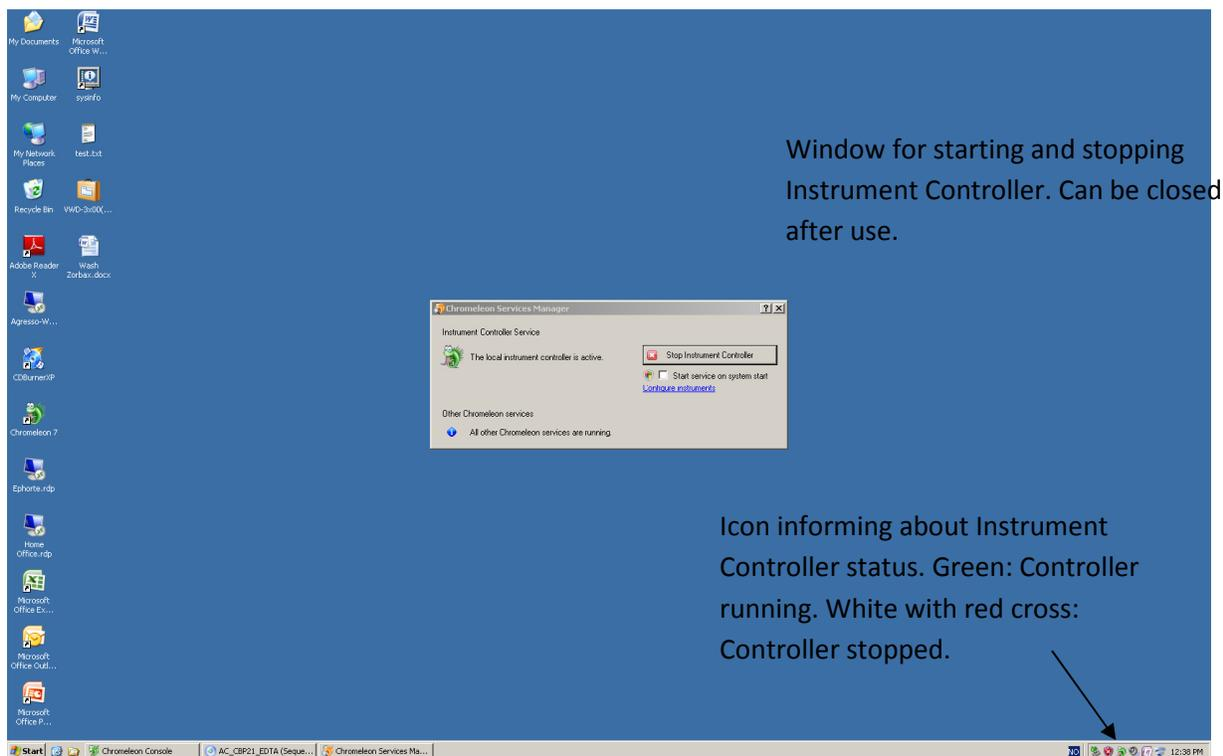
**Figure 2: Instrument Controller. Software unit that controls communication between computer and HPLC. Must be running at all times when system is operated.**
