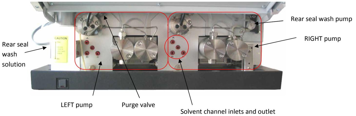
Figure 4: Internals of Dual Pump
