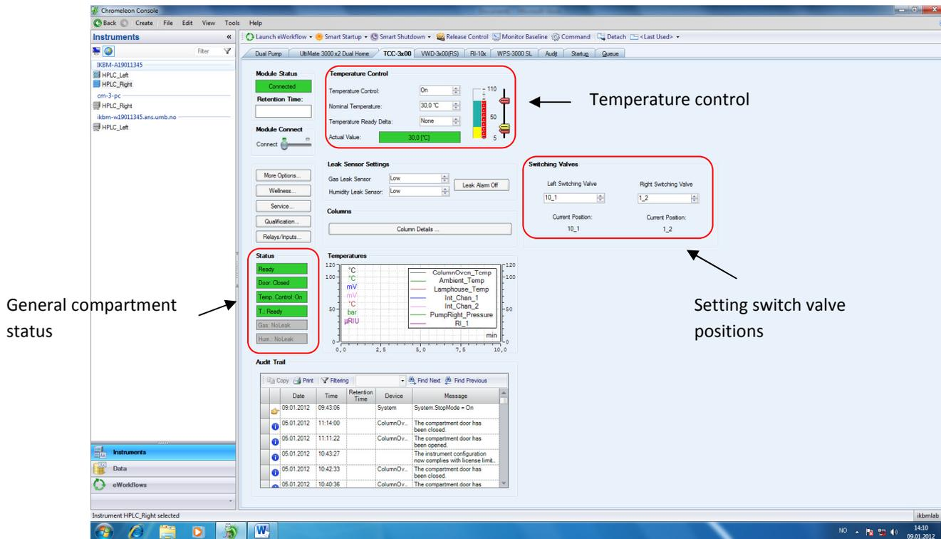
Figure 12: Column compartment tab controlling column temperature and switch valve configuration.
