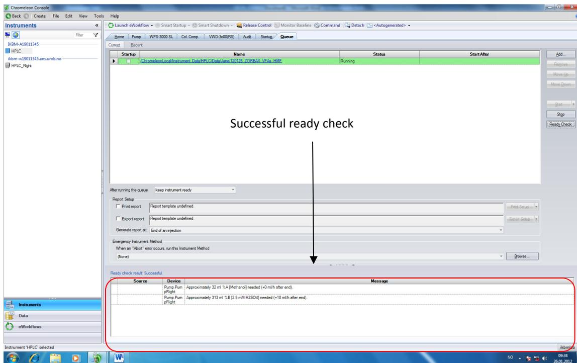
Figure 14: Top screen dump: Queue tab. Here sequences can be queued for automatic start and general checking of system status (ready check) is performed. Lower screen dump: Ready Check with estimated eluent consumption.
