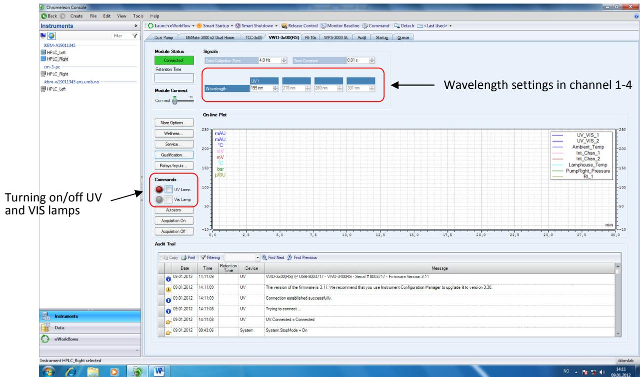
Figure 13: UV detector tab for turning on and off UV/VIS lamps and setting wavelength.
