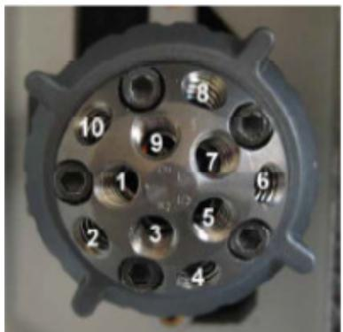
Figure 11: 10-port switch valve with port numbers.
