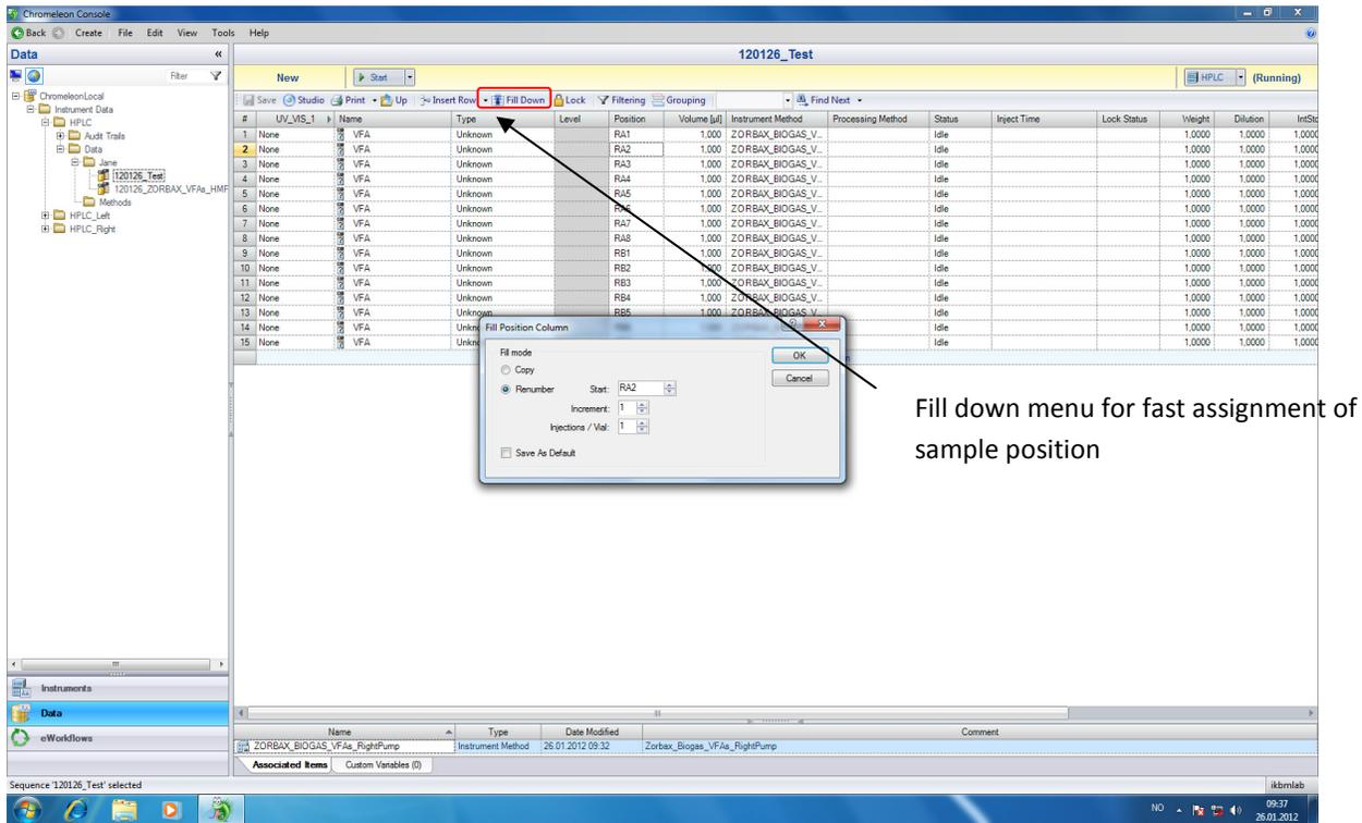
Figure 17: Fill Down menu for fast assignment of sample position. Please mark the field of the first sample in the order.
