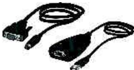
Figure B-1 Molecular Devices' custom serial cable (left) and a serial-to-USB converter (right).
