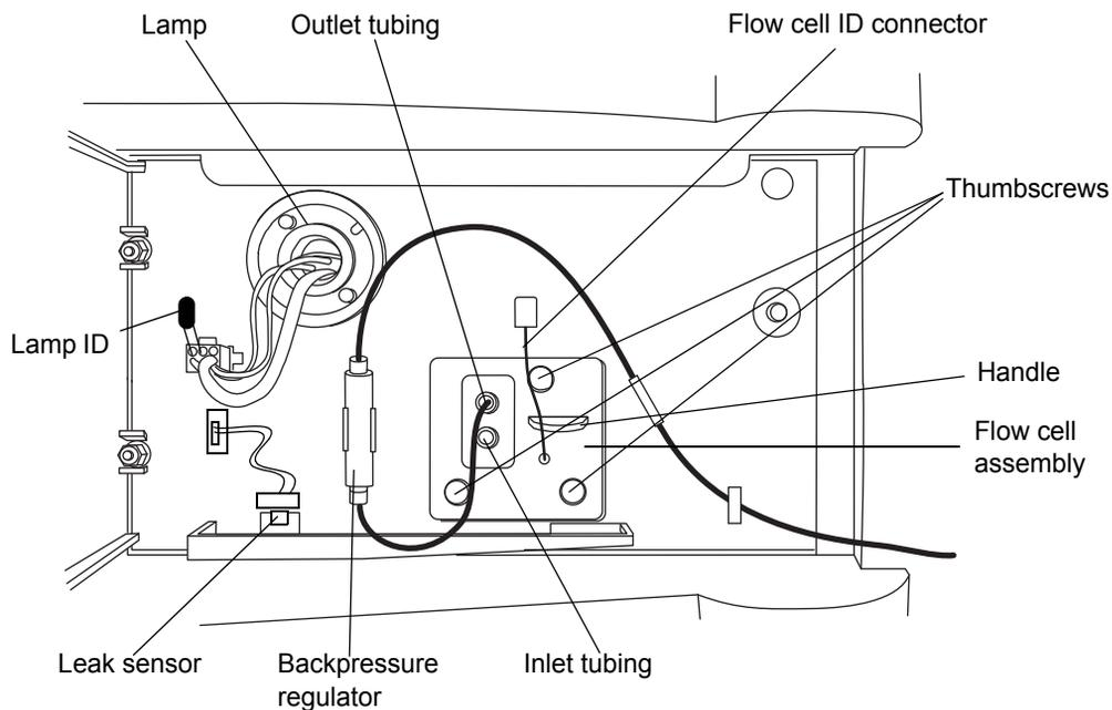
5. Remove the protective cover from the PEEK cell inlet tubing, and connect the tubing to the flow cell inlet, confirming that the label on the tubing matches the type of detector and flow cell in your system.
