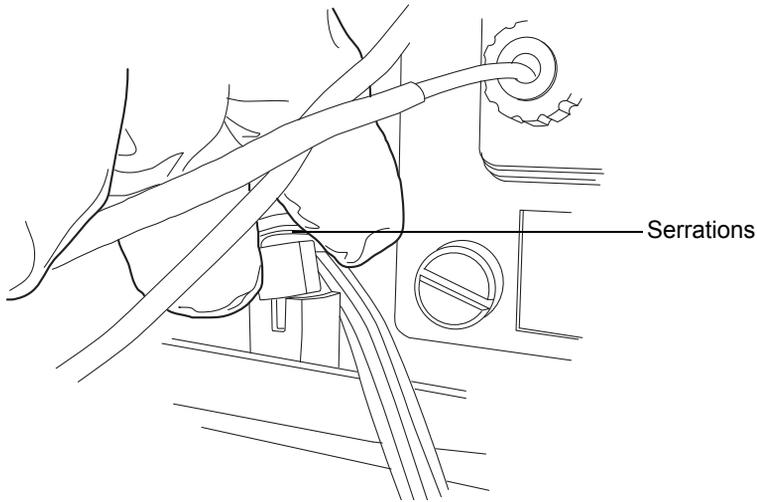
**Tip:** If you cannot easily manipulate the leak sensor after removing it from its reservoir, detach the leak sensor connector from the front of the instrument (see the figure on [page 36](#)).
