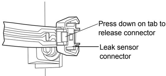
3. Remove the leak sensor from its reservoir by grasping it by its serrations and pulling upward on it.
