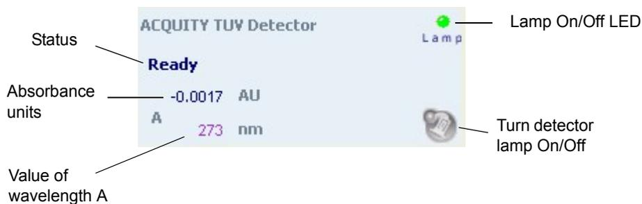
The detector control panel displays the acquisition status (if the detector is running). You cannot edit detector parameters while the system is processing samples.
