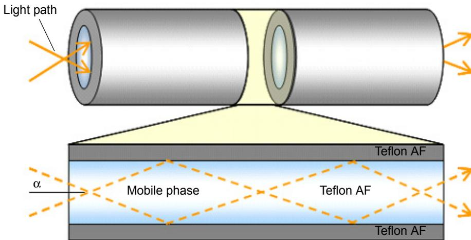
In the figure above, the light path through the cell is depicted by a pair of rays (dashed lines) that bounce off the cell wall. The energy carried by each ray is conserved after each bounce. One hundred percent of the light is reflected, hence the term “total internal reflection”. The Teflon AF tubing is an active component in the flow cell light path.
