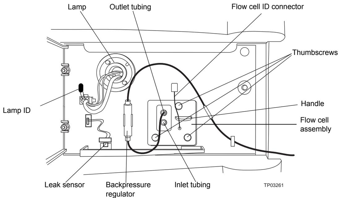
5. Disconnect the flow cell ID connector (if present).
