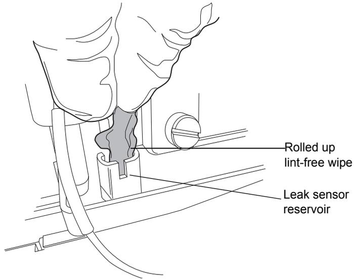
7. With a cotton swab, absorb any remaining liquid from the corners of the leak sensor reservoir and its surrounding area.
