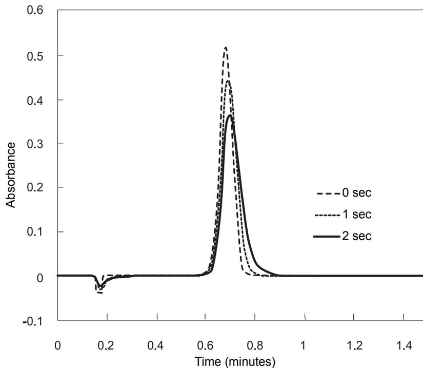
**Tip:** Although the peak shape shows some distortion and the signal output is delayed with different time-constants, the peak area remains the same.
