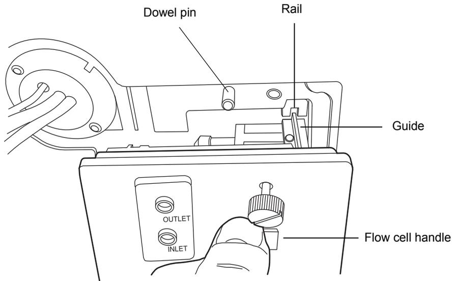
2. After the flange and rails are engaged, continue inserting the flow cell until the dowel pins on the detector engage the corresponding holes on the cell holder.
