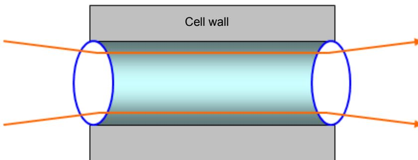
The light path through a conventional flow cell is designed to avoid contact with the cell walls, primarily to prevent rays that encounter the walls from contributing to the measured signal. The energy associated with errant rays is highly variable depending on the mobile phase composition, quality of wall
