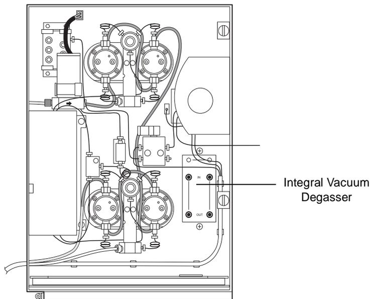
Figure 1-1 Waters 1525 HPLC Pump with Integral Vacuum Degasser
