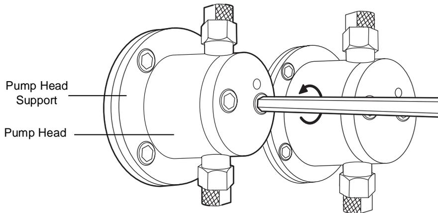
Figure 2-2 Removing Head Bolts (1525 Analytical and 1525EF Shown, 1525 $\mu$  Similar)
