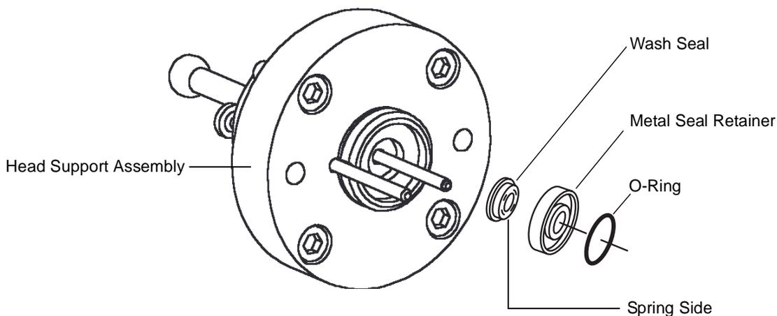
Figure 2-8 1525 $\mu$  Head Support Components
