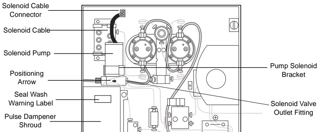
Figure 2-9 Correct Solenoid Positioning
