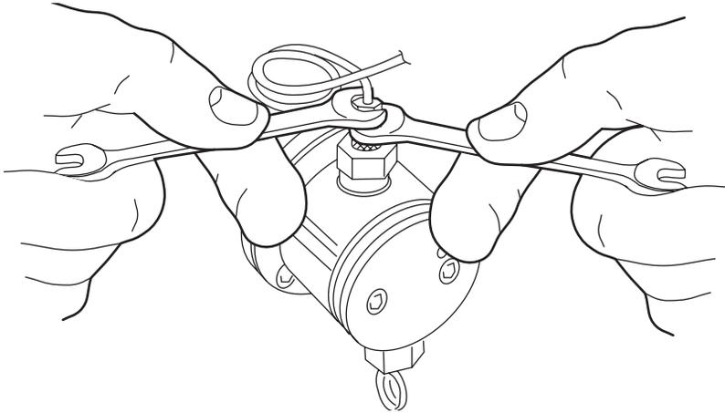
Figure 2-1 Loosening Fittings (1525 Analytical and 1525EF Models)
