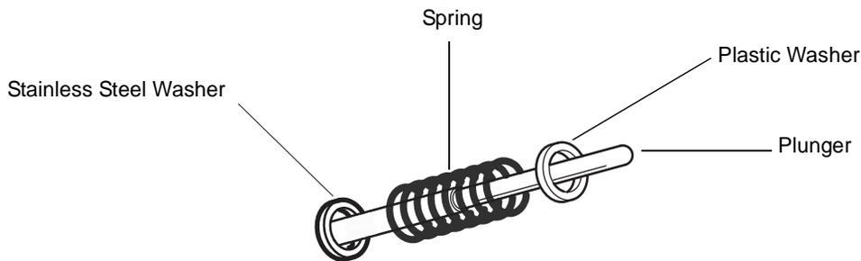
Figure 2-7 Installing the 1525EF Washers and Spring
