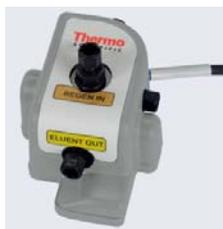
The Dionex CR-TC is a high-pressure, electrolytically-regenerated trap column. The Dionex CR-TC is designed to remove anionic or cationic contaminants in the eluent or deionized water and to reduce drift during gradient separations. The following versions of the Dionex CR-TC can be used with the EG:
