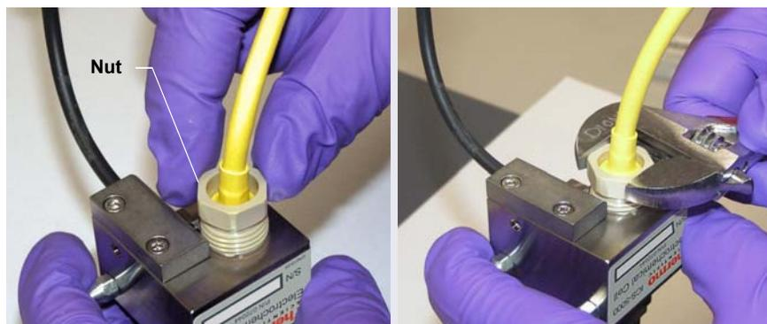
**Figure 9-73.** Installing the PdH Reference Electrode Nut
