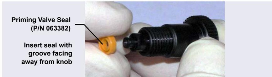
**Figure 9-12.** Replacing the Priming Valve Seal
