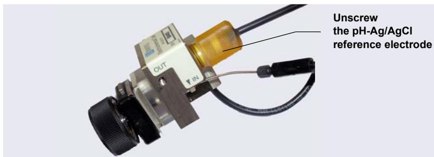
**Figure 9-59.** Removing the pH-Ag/AgCl Reference Electrode (Cell Configured for Analytical IC Shown)
