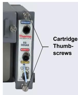
**Figure 9-41.** Capillary Cartridge Thumbscrews
