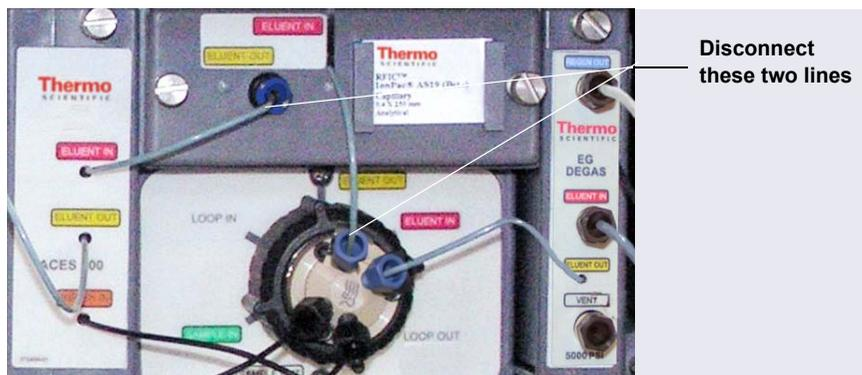
**Figure 9-44.** *Disconnect Capillary Tray Eluent Lines (Conductivity System Plumbing Shown)*
