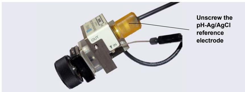
**Figure 9-66.** Removing the pH-Ag/AgCl Reference Electrode (Cell Configured for Analytical IC Shown)
