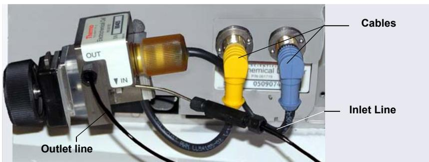
**Figure 9-55.** *Disconnecting the ED Cell
