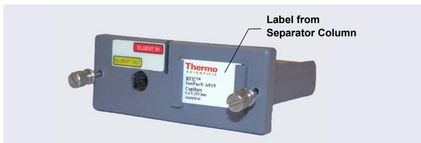
**Figure 9-46.** Capillary Column Tray with Column Label
