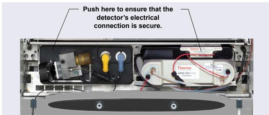
**Figure 8-1.** Detector Connection
