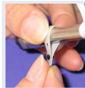
**Figure 9-75.** Attaching the Column ID System to the Column
