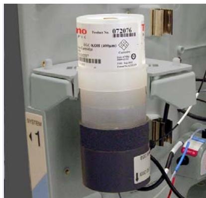
**Figure 9-19.** Capillary Dionex EGC Installed on Holder
