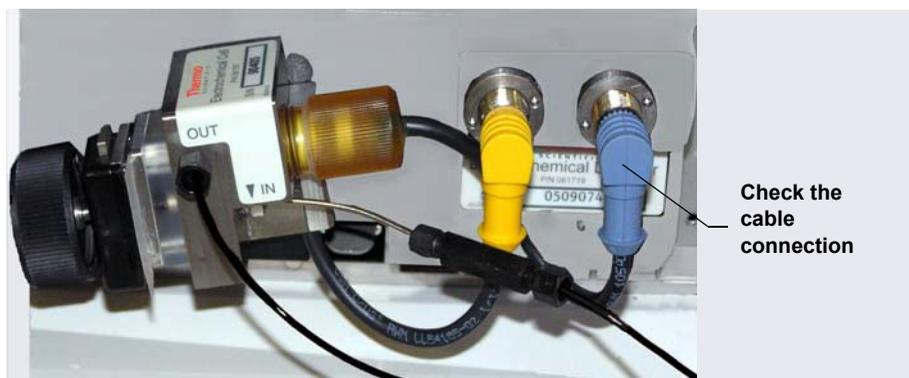
*Figure 8-8. ED Cell Electrical Connections*
