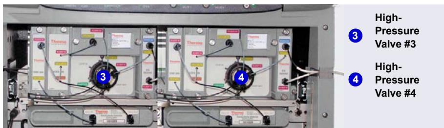
**Figure 8-6.** High-Pressure Valves #3 and #4 (On IC Cubes)
