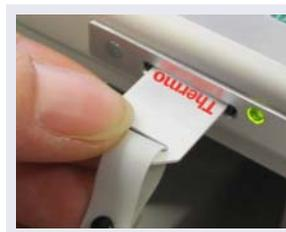
**Figure 9-76.** Inserting a Column ID Chip Card
