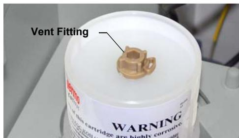
**Figure 9-15.** Capillary Dionex EGC Vent Fitting
