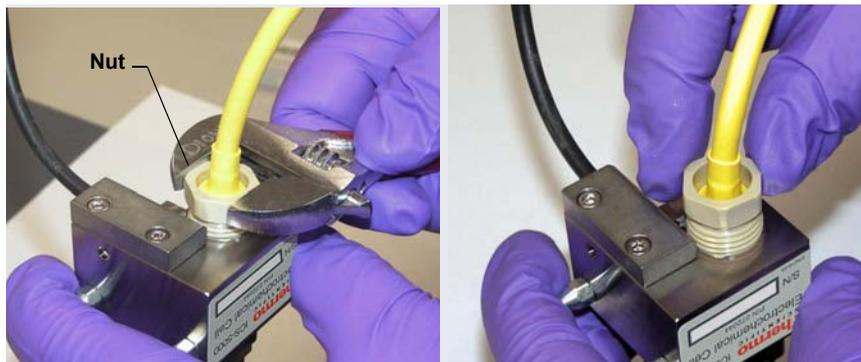
**Figure 9-68.** *Unscrewing the PdH Reference Electrode Nut*
