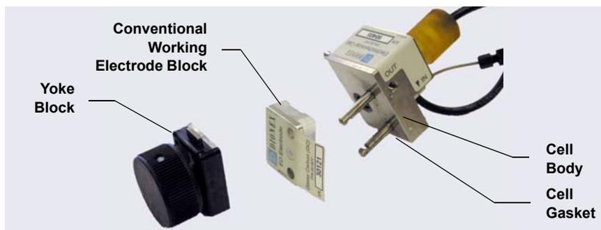
**Figure 9-57.** ED Cell Components
