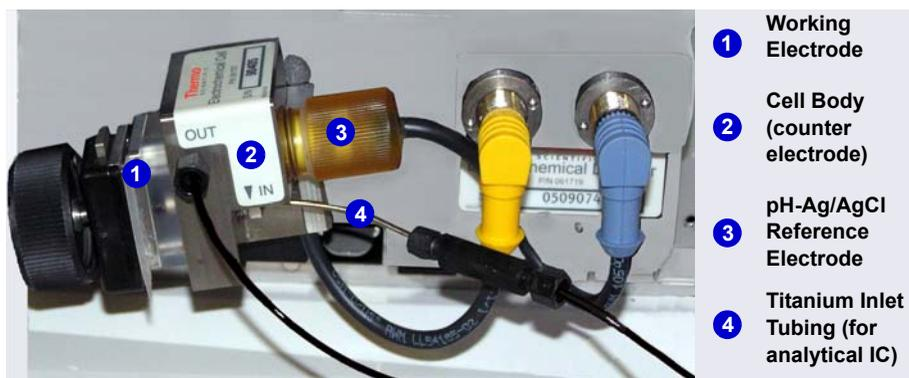
**Figure 2-32.** ED Cell with pH-Ag/AgCl Reference Electrode
