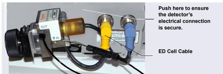
**Figure 8-4.** *Electrochemical Detector Connection (Analytical Cell Shown)*
