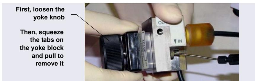
**Figure 9-56.** Disassembling the ED Cell
