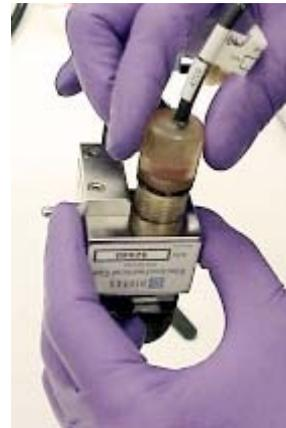
**Figure 9-64.** Installing the pH-Ag/AgCl Reference Electrode In the Reference Electrode Well
