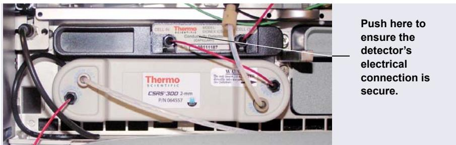
**Figure 8-3.** Conductivity Detector Connection
