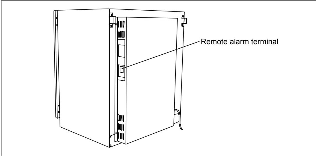
The remote alarm terminal is a contact output.
