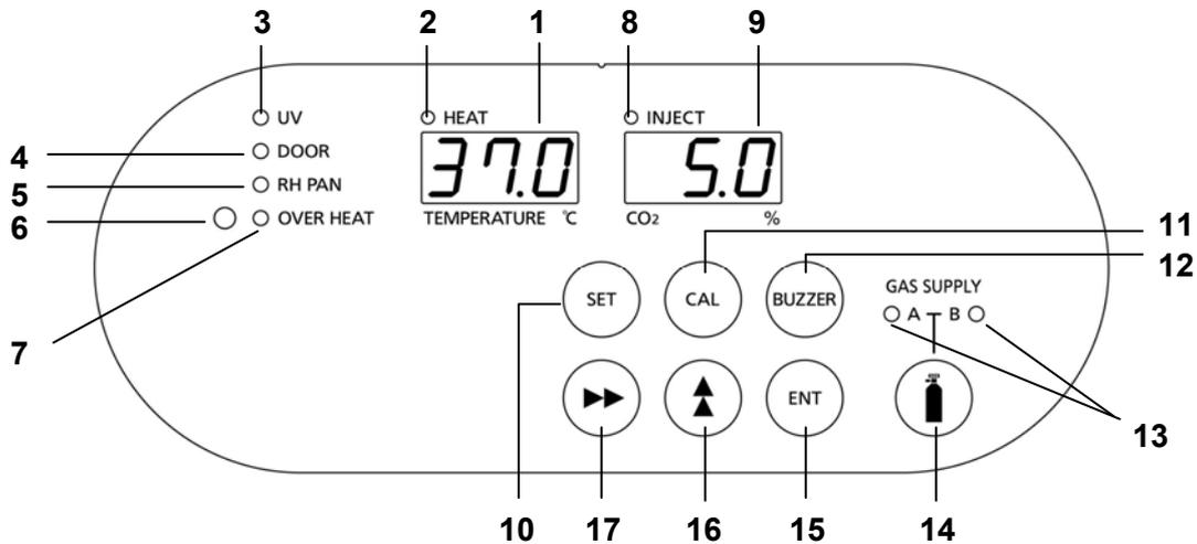
**1. Digital temperature indicator (TEMPERATURE °C):** Normally, this indicator shows the chamber temperature. In the setting mode, it shows the set value of the chamber temperature. If the self diagnostic function detects any abnormality, an error code will be displayed.
