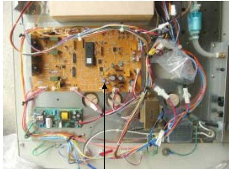
CO2 IR sensor power consumption resistance (R13)
