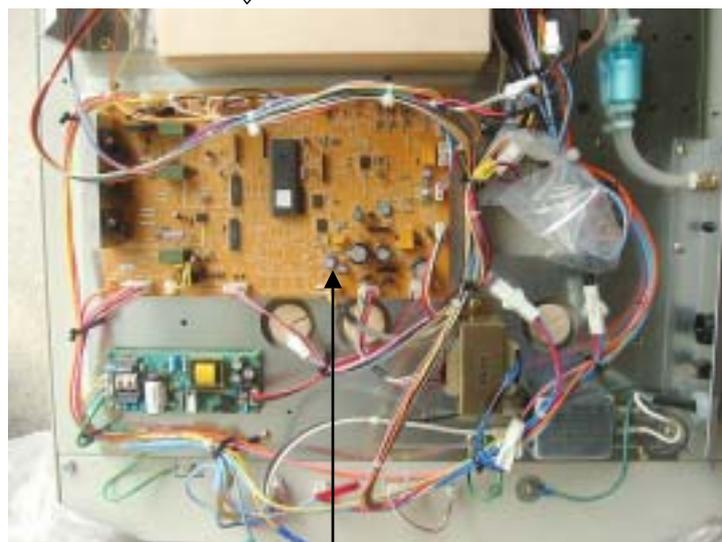
CO2 IR sensor power consumption resistance (R13)
