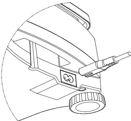
Figure 2-3A. Connect the AC power plug to the input jack on the back of scale.
