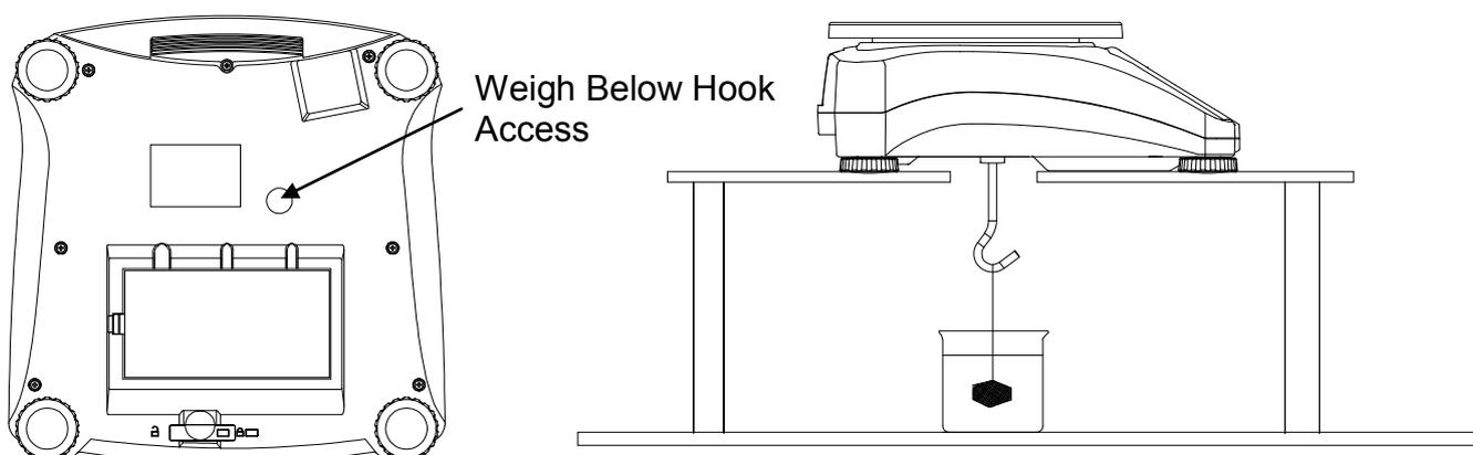
Figure 4-1. Setup for the Weigh Below Hook
