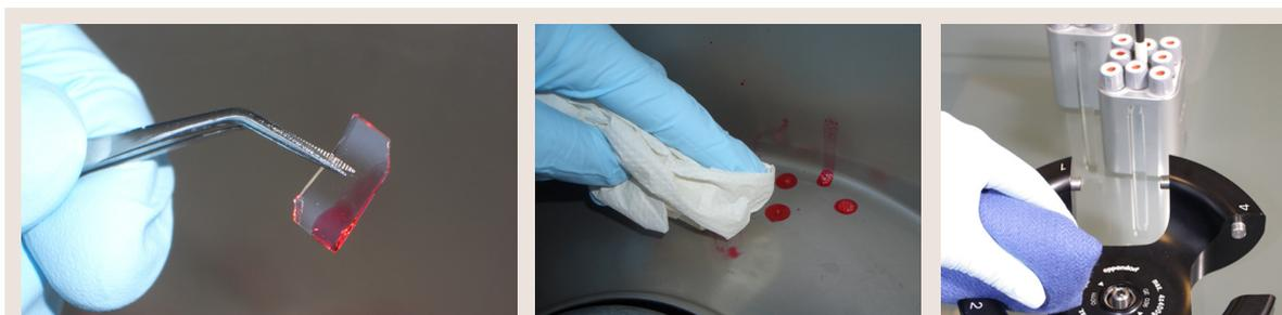
Figure 3: Decontamination of centrifuge, rotor and rotor buckets.
