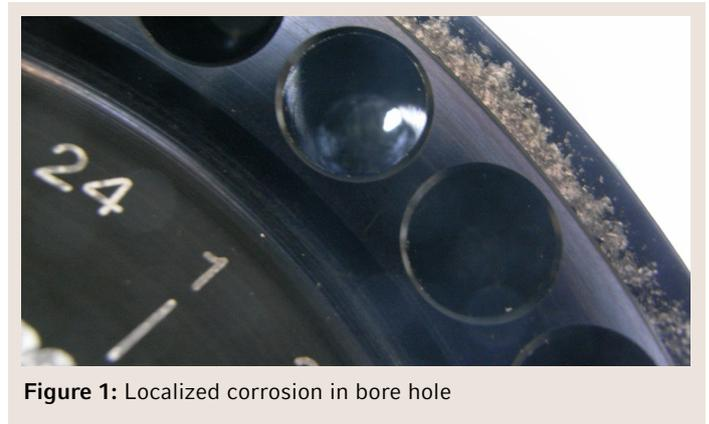
Figure 1: Localized corrosion in bore hole
