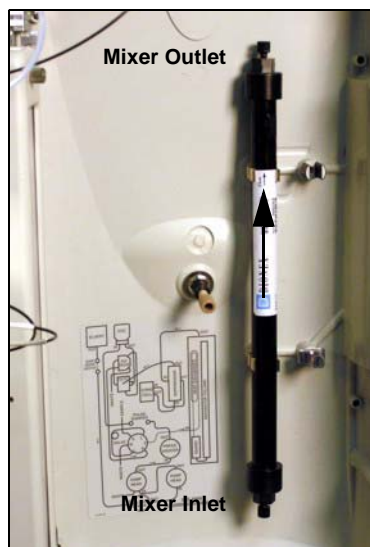
Figure B-69. EGC CO 3 Mixer Installed on the ICS-2000 Door
