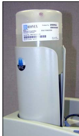
Figure B-57. EluGen Cartridge Installed in the Holder
