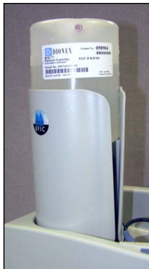
Figure B-81. EluGen Cartridge Installed in the Holder
