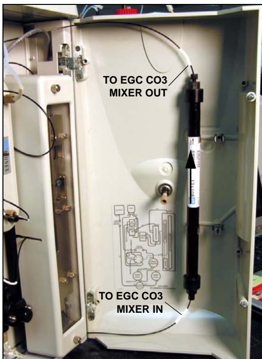
Figure 5-62. ICS-2000 with an EGC CO 3 Mixer Installed
