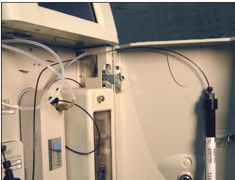
Figure B-92. Mixer Outlet Routed to the Back of the Component Panel
