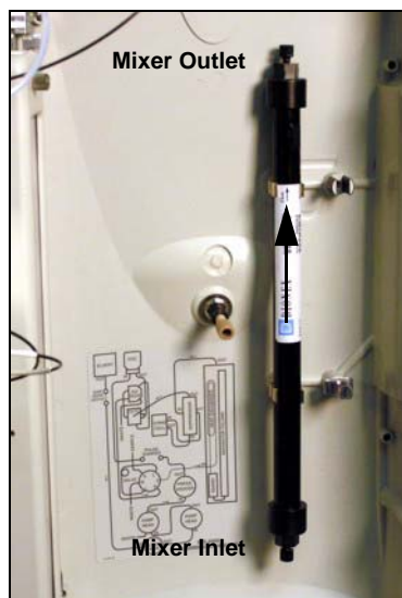
Figure B-89. EGC CO 3 Mixer Installed on the ICS-2000 Door
